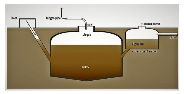
Figure 9-5: Anaerobic Digester (from Tilley et al. (2014))
