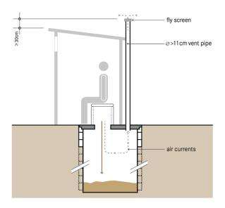
Figure 9-3: Ventilated Pit Latrine (from Orner et al. (2018))
