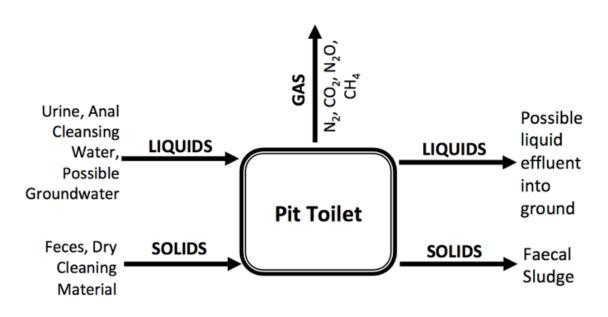
Figure 9-2: Basic inputs and outputs in a pit latrine (from Orner et al., 2018)
