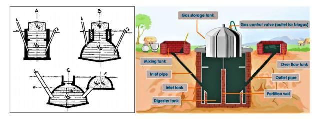
Figure 9-7: Fixed dome anaerobic digester (from Tiley 2014)
