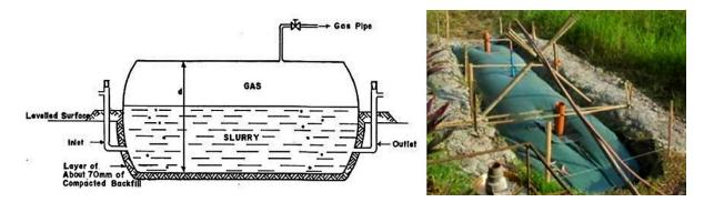
Figure 9-6: Plastic bag anaerobic digester (from Tiley, 2014)
