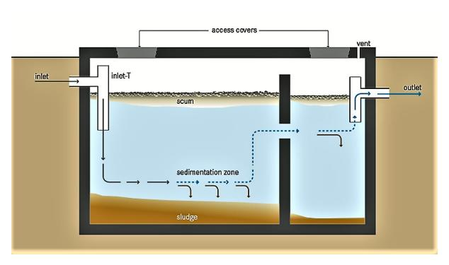
Figure 9-4: Septic Tank (from USEPA (2021))
