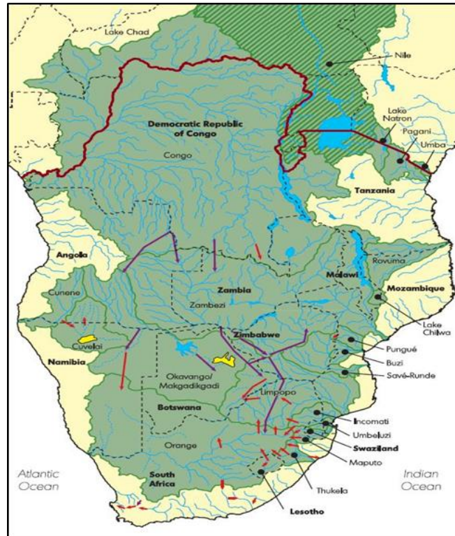
Figure 2.8: Current and planned transboundary interbasin transfers. Source: (Turton, 2016). Note: Red lines indicate current transfers; purple lines indicate planned
