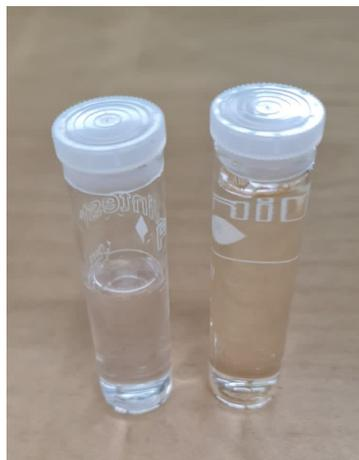
**Figure 4-14:** Treated iron ore wastewater samples after filtration. The concentration of Fe was 0.5 mg/L after treatment/flocculation.
