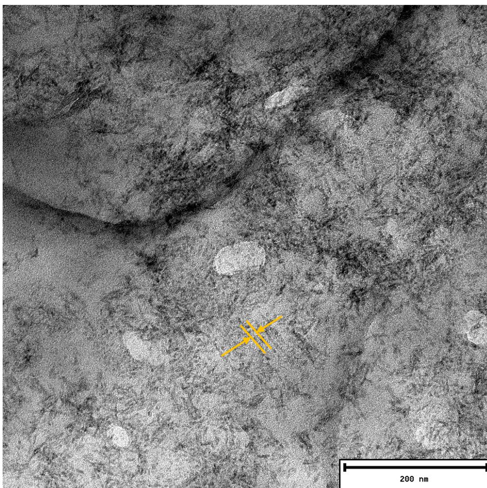
**Figure 4-8: TEM micrograph of BNC1. Orange arrows show the diameter of a rod-shaped nanocoil.**
