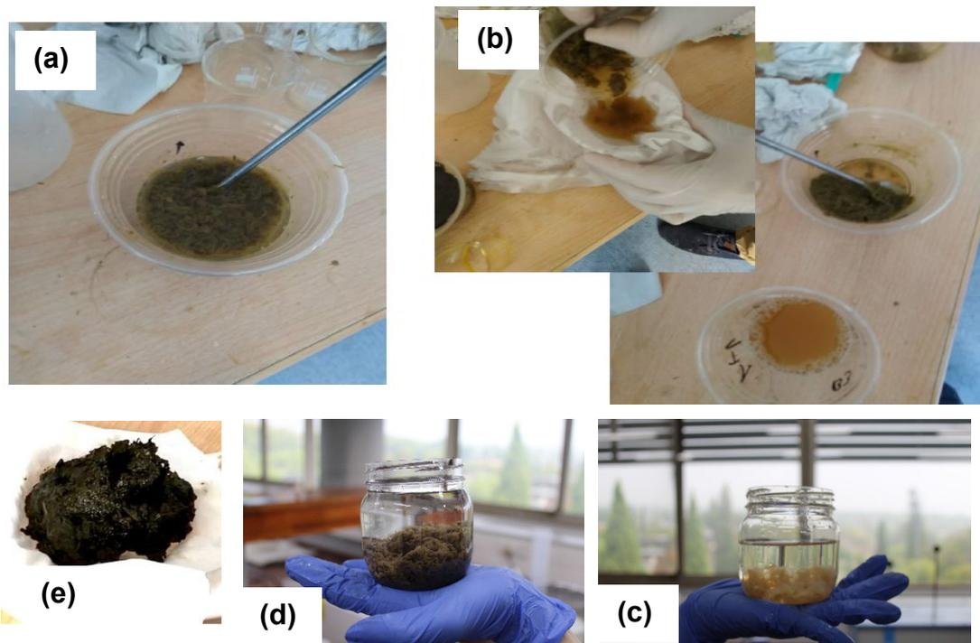
**Figure 4-5:** Pictures showing de-watering (solid removal) performance of the modified BNC: (a) sewage samples with small quantities of BNCs, (b) separation of sludge from residual water through filtration and decantation, (c, d) images showing how solids separate from solution after addition of BNCs, (d) sludge after de-watering with BNCs.
