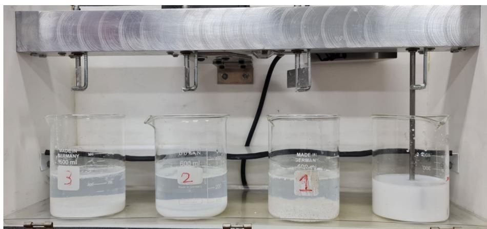
**Figure 3-4: Jar test apparatus used for BNC flocculation test work.**
