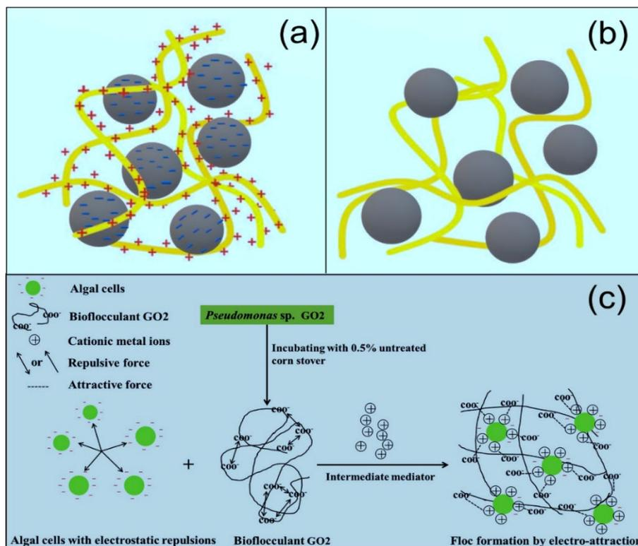
**Figure 2-1: Mechanism of flocculation during harvesting: (a) charge neutralization; (b) polymer bridging; and (c) floc formation through electrostatic interaction [16,29].**
