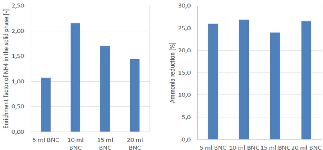
**Figure 4-2: The effect of adding different dosages of BNC1 on a wastewater sample. Data on the left show enrichment factors for ammonia. Data on the right show ammonia reduction.**
