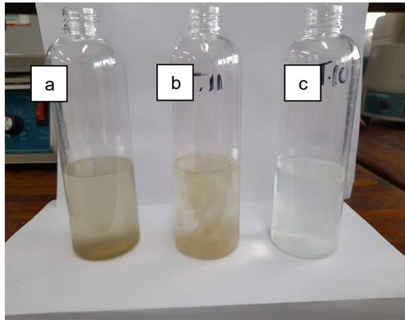
**Figure 4-16: Pictures of fisheries wastewater treated with (a) BNC2, (b) BNC1 and (c) a clear filtered solution of treated fisheries using BNC1.**
