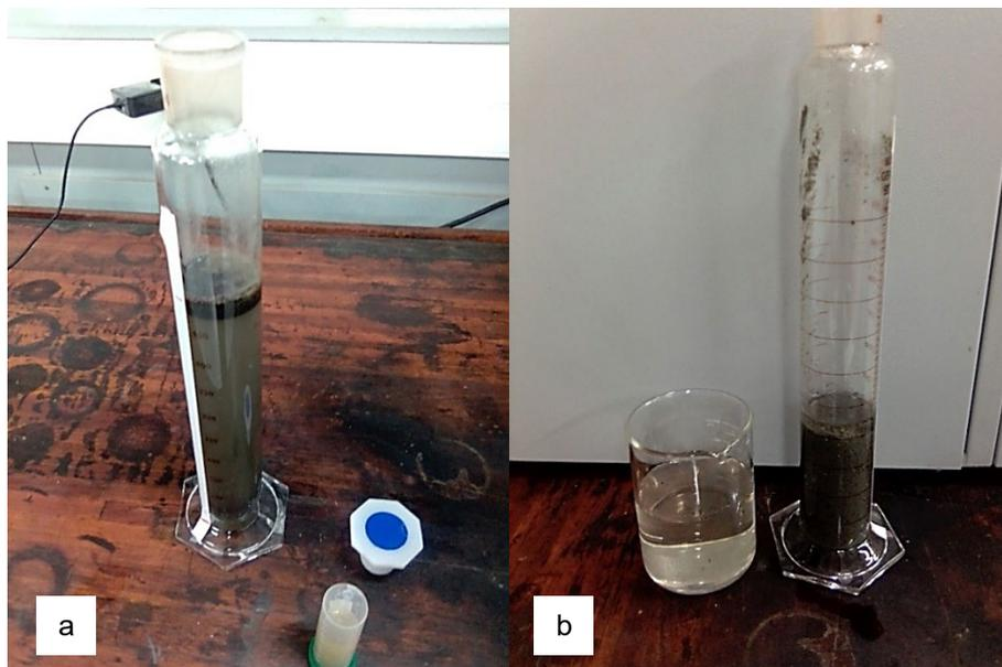
**Figure 4-15: (a) A mixture of A+B untreated wastewater, and (b) clear water removed from the cylinder after flocculation and filtration.**
