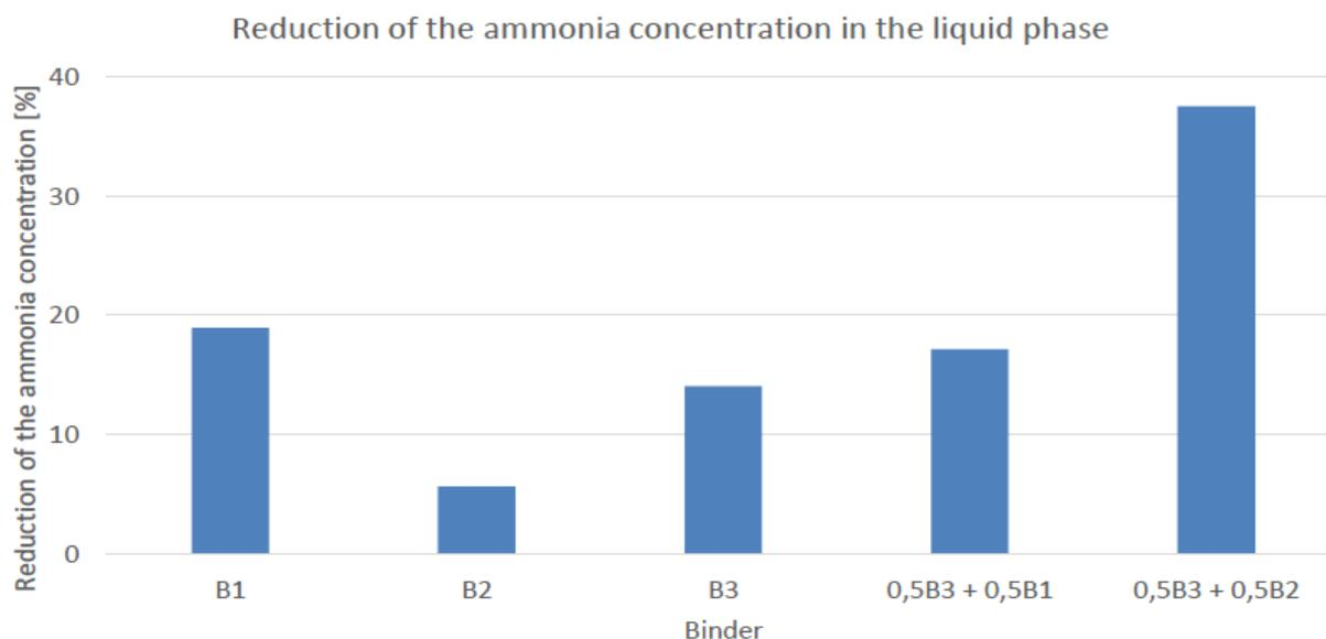
**Figure 4-3: Reduction of ammonia in the liquid phase using locally available binder materials.**
