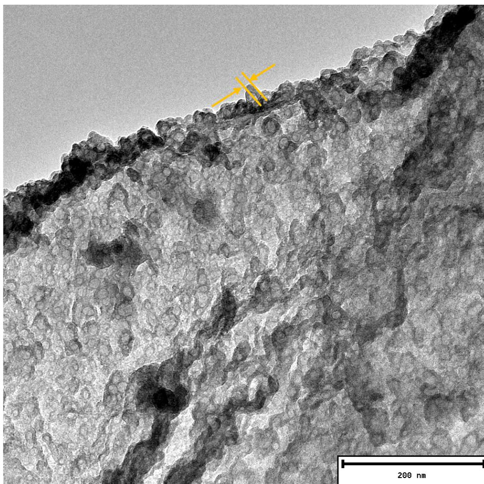
**Figure 4-9: TEM micrograph of BNC2. Orange arrows show the diameter of a round-shaped nanocoil.**
