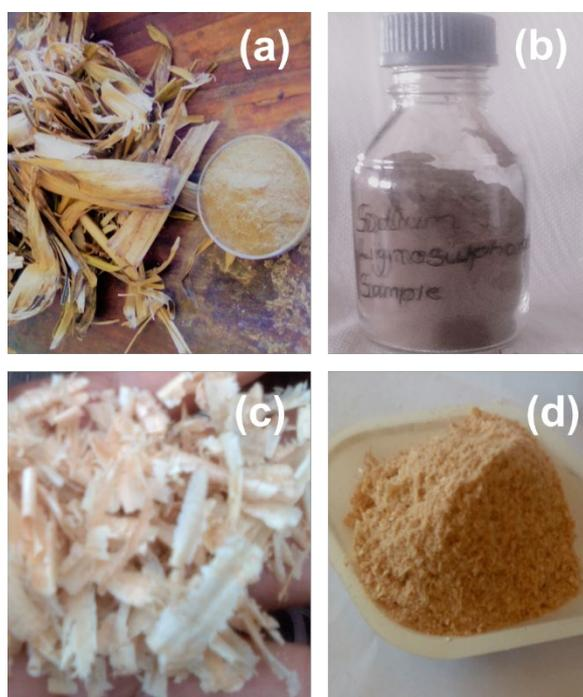
**Figure 3-1: Pictorial representation of biomass materials use in this study (a) maize stalk (agro waste), (b) lignosulfonate, (c) wood shavings, and (d) wood sawdust.**
