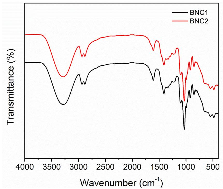
Figure 4-11: The FTIR spectra of BNC1 and BNC2.
