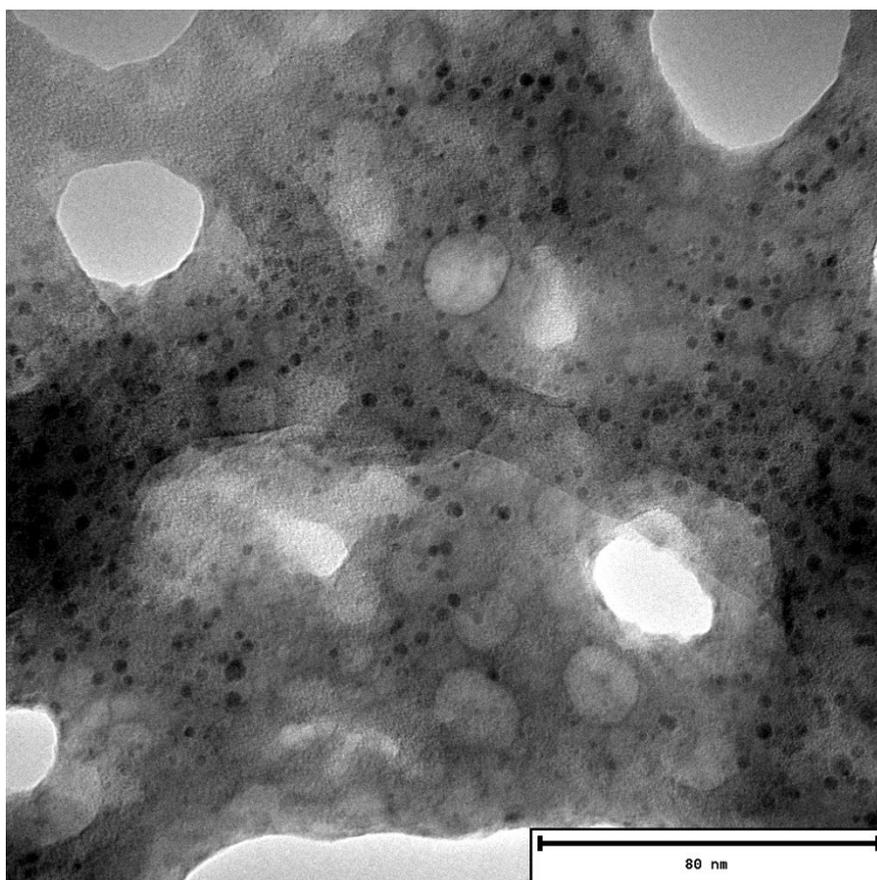
**Figure 4-10: TEM micrograph of Binder 1. The fine nanoparticles of the binder (binder 1) are black dots in the image.**
