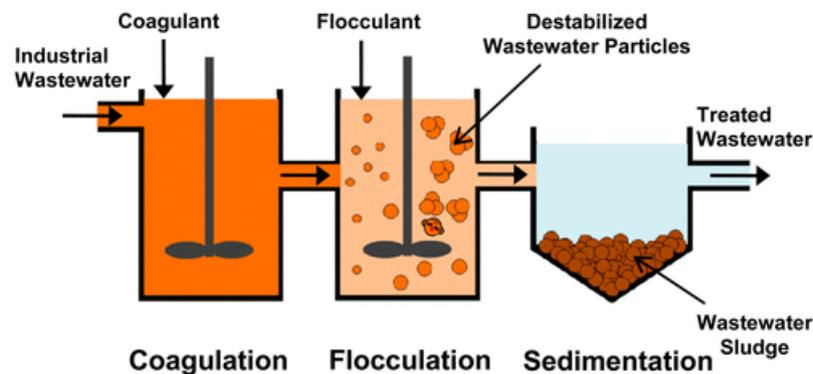
Figure 4-7: A typical coagulation-flocculation setup for industrial wastewater treatment.
