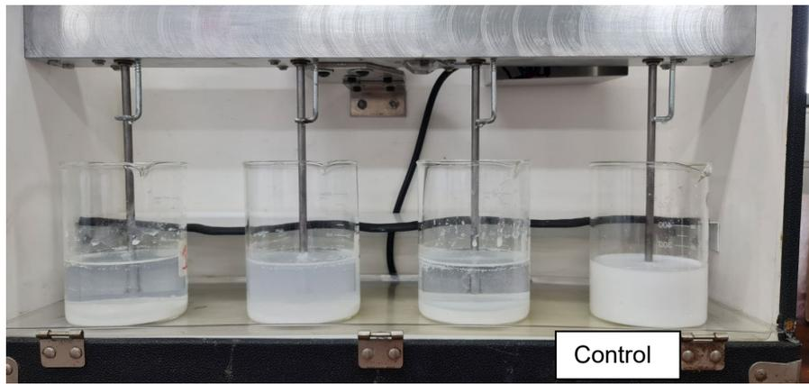
Figure 4-18: Images of milk of magnesia wastewater (250 ml) treated with different concentrations of BNC1. Smaller flocs were formed.
