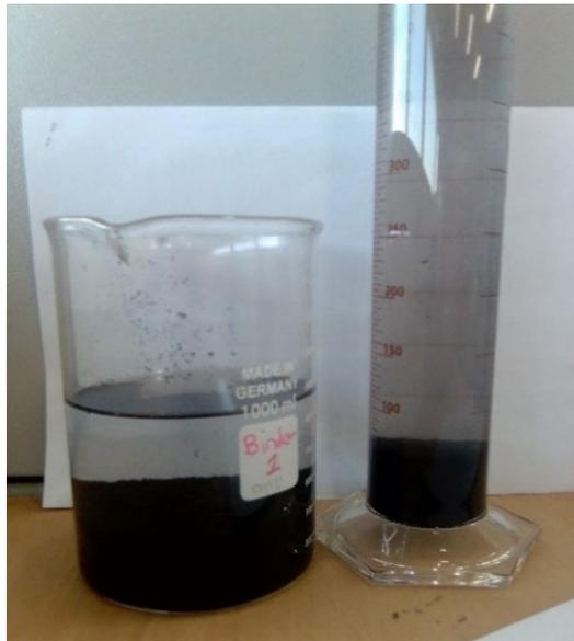
**Figure 4-20: Comparison of the coal wastewater treated with BNC1 (beaker) and with conventional chemical flocculant.**
