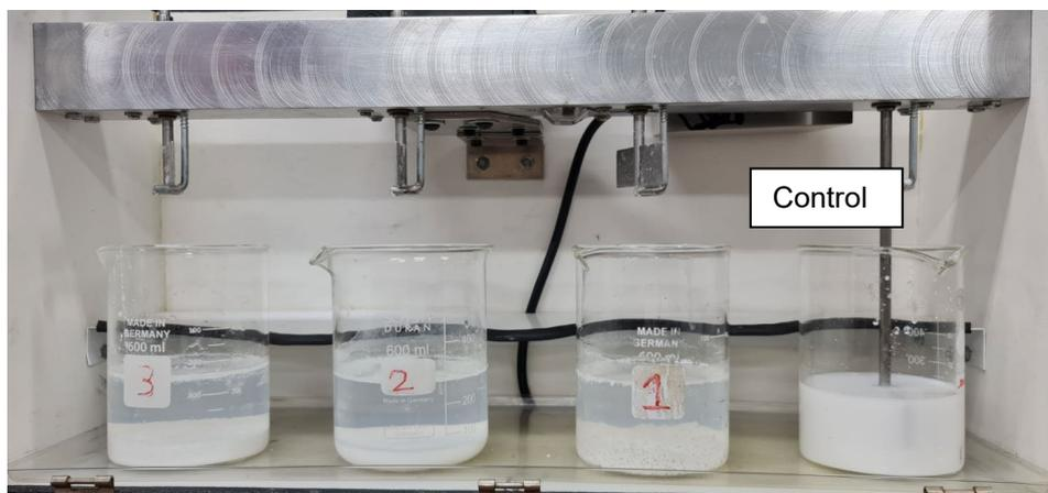
Figure 4-19: Images of milk of magnesia wastewater (250 ml) treated with different concentrations of BNC1. Bigger flocs were formed.
