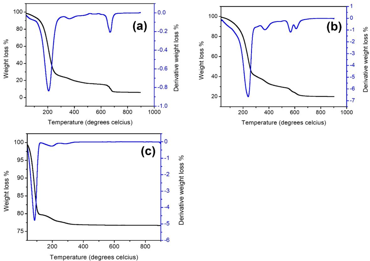
Figure 4-12: The TGA curves of (a) BNC1, (b) BNC2 and (c) binder.
