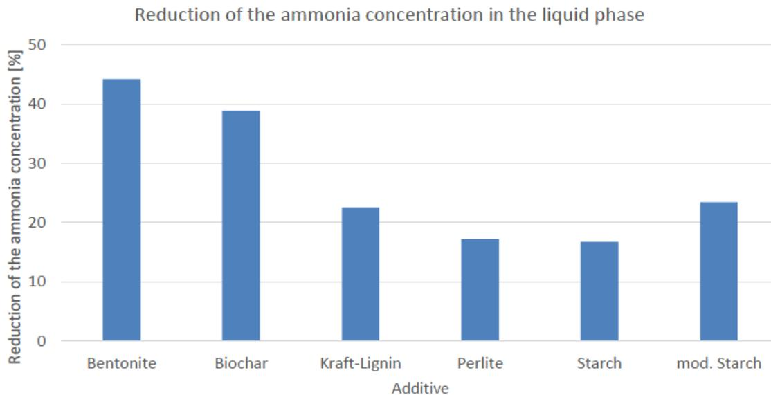
**Figure 4-1: Reduction of ammonia concentration in the liquid phase by different materials.**
