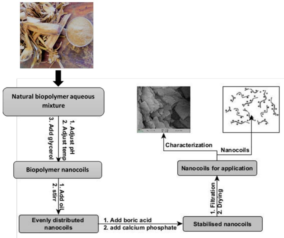
**Figure 3-2: A graphical sketch for extraction and conditioning of biopolymer nanocoils used as flocculants.**
