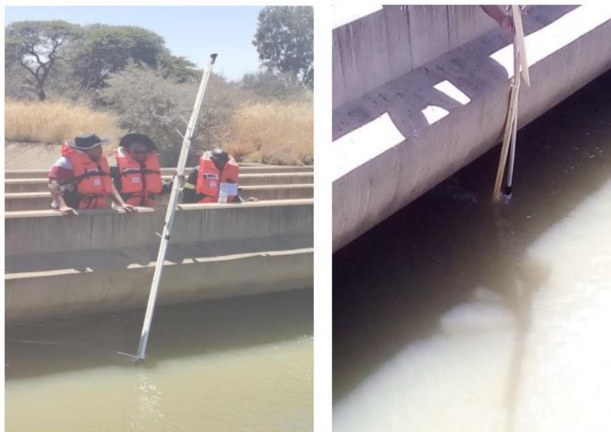
Figure 2: Photos showing an improvised support system to the flow meter pole (left) and the broken wooden support (right). The breakage was caused by the strong water flow in the main canal at Vaalharts irrigation scheme. The flow depth was greater than 2 m and the flow velocity was almost 2 m/s.
