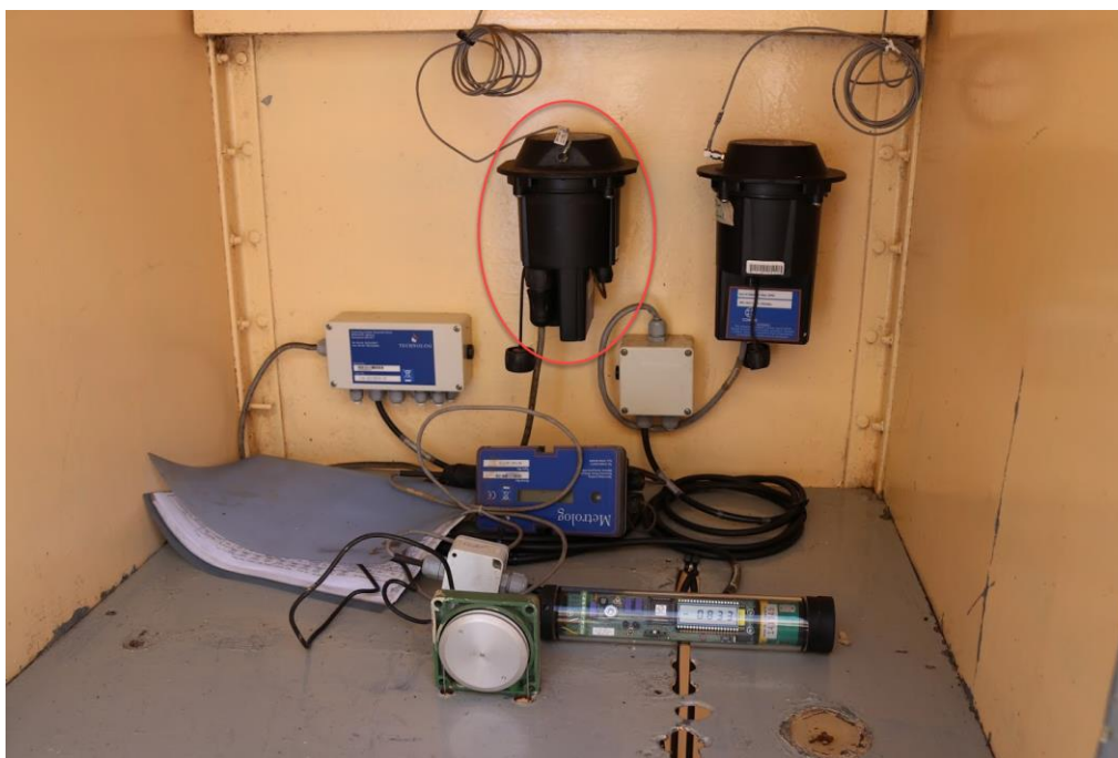
FIGURE 4.7 Cello data logger at left bank inflow for Loskop irrigation scheme
