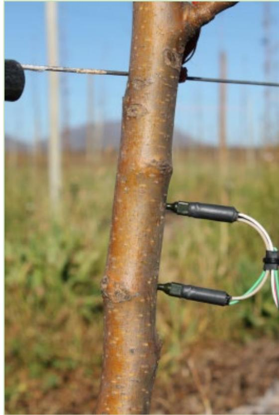
*Figure 2.6: Measurement of transpiration in young orchards using Granier probes.*
