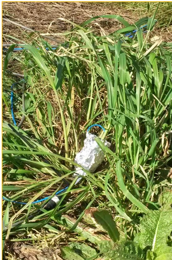
*Figure 3.3: Stem heat balance sap flow sensor measuring transpiration by grass species on the floor of an apple orchard.*
