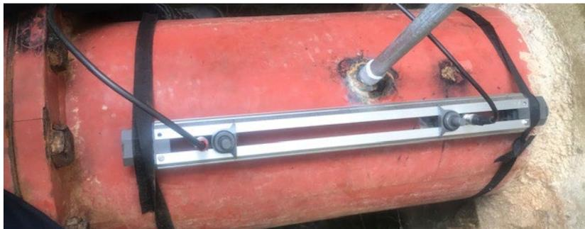
**Figure 3.8: Photo of the ultrasonic flowmeter used during this study.**
