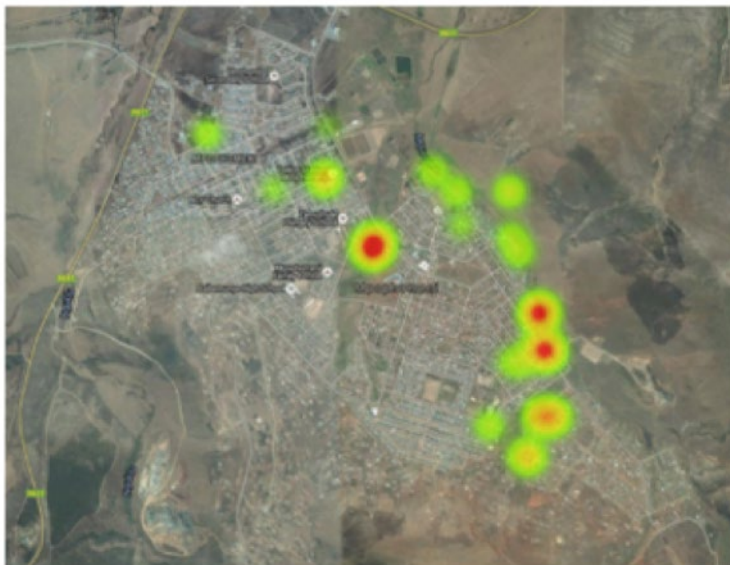
Figure 44: Heatmap illustrating the use of citizen science approaches to monitoring which facilitates rapid response. This mapping process allows the identification of “Hot Spots” of high incidents of surcharging manholes.
