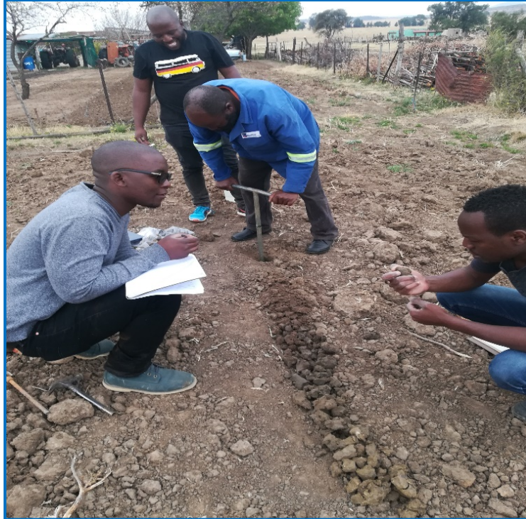
Figure 4.7 Soil field evaluation and data collection by auguring to a depth of 120 cm with the participation of farmers and students after site selection
