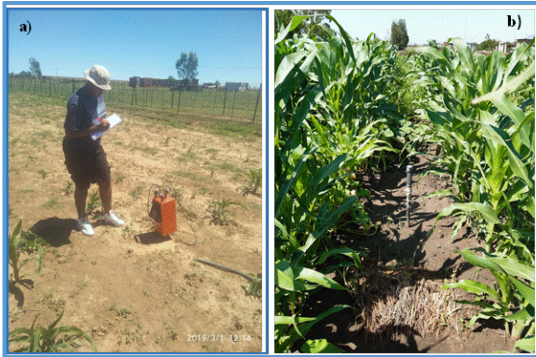
Figure 4.8 Monitoring soil water content using a) neutron water meter or neutron probe (NWM) during the growing season at Morago site demonstration plot, and b) DFM (CLP180 Moisture probe) installed between plant rows (at Paradys site)
