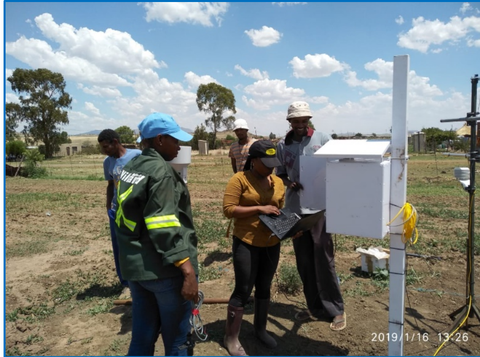
Figure 4.5 The assembled AWS erected in the demonstration plot of Paradys village. Showing regular weather data downloading by students and technicians.
