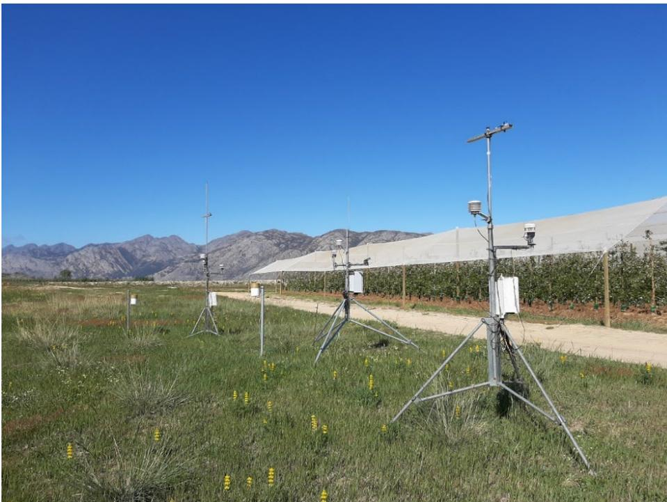
Figure 26. Positioning of the three Automatic Weather Stations for the cross-calibration exercise in September 2019.
