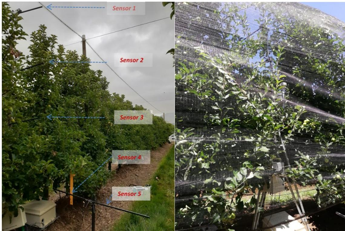
Figure 30 Placement of the quantum line sensors to measure the intercepted PAR radiation at different levels in the 'Rosy Glow' canopy (fixed net) and the 'Golden Delicious Reinders' canopy (draped net).
