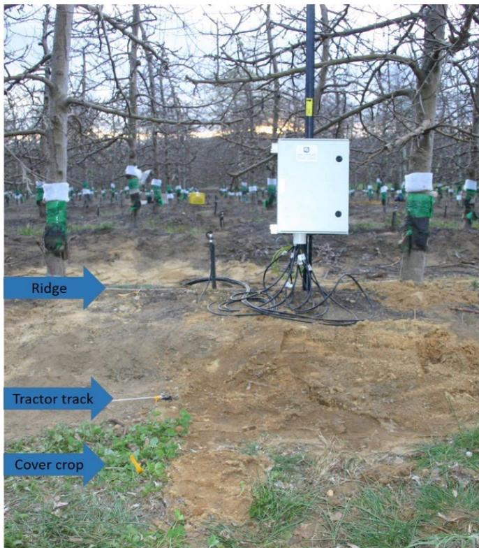
Figure 35 Installation positions of CS616 sensors in sandy soil in the draped net 'Golden Delicious Reinders' orchard at Paardekloof in 2019-2020. The rods of sensors installed across the ridge are centred on the middle of the tractor track and cover crop sensor rods. Yellow labels and white ropes indicate the positions of the sensors below ground.
