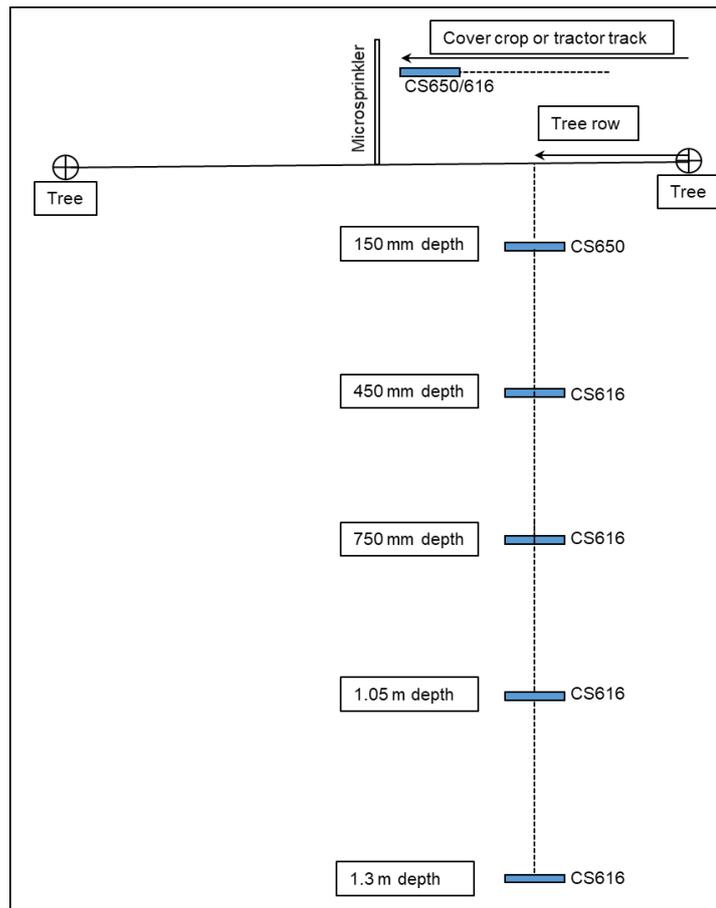
Figure 139 Illustration of the position and depths of the CS650 and CS616 sensors installed in the centre tree row, tractor track or cover crop relative to the tree (encircled cross) below the open and draped net sections in the 'Golden Delicious' orchard at Southfield in 2020. Sensors in the tree row were installed across the centre tree row.
