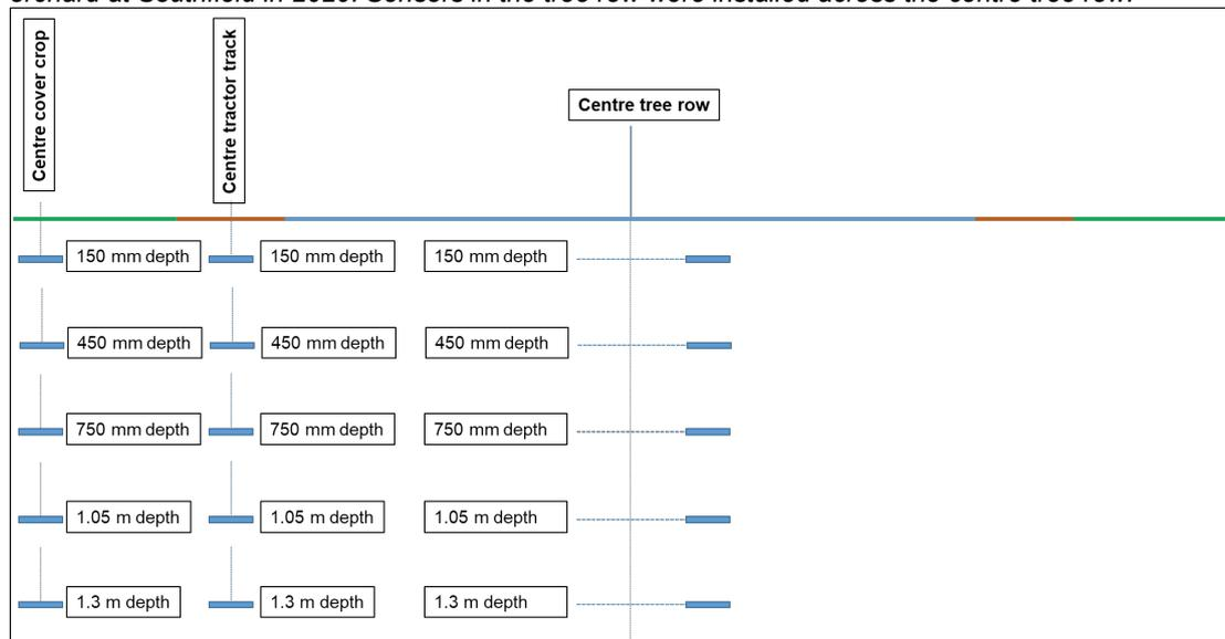
Figure 140 Illustration of the position and depths of the CS650 and CS616 sensors (blue blocks) installed in soil relative to the 'Golden Delicious' trees at Southfield in 2020.
