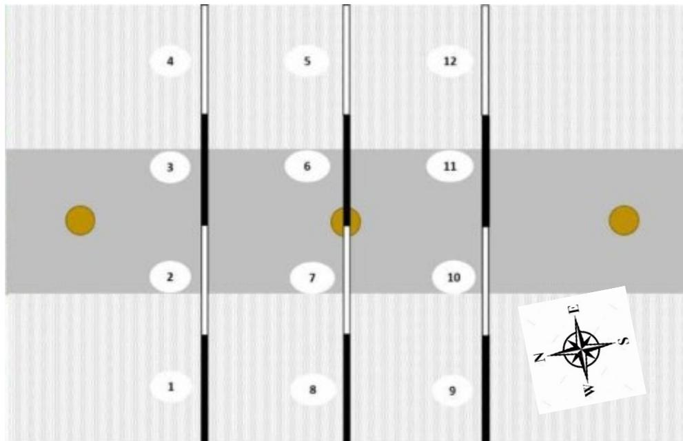
Figure 29 Grid for ceptometer PAR measurements in the shaded and open orchards. Orange circles indicate tree trunks. The row orientation is north-north-west by south-south-east.
