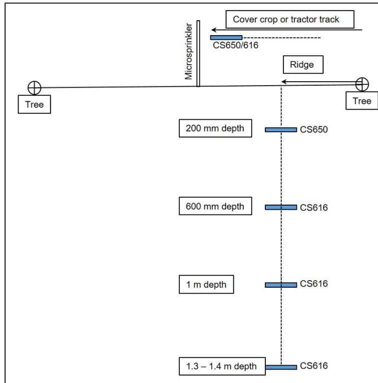
Figure 137 Illustration of the position and depths of the CS650 and/ or CS616 sensors installed in the ridge, tractor track or cover crop relative to the tree (encircled cross) in the 'Rosy Glow' and 'Golden Delicious Reinders' orchards at Paardekloof. Sensors in the ridge were installed across the ridge.
