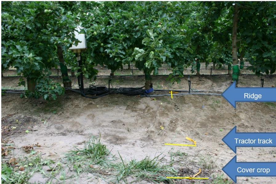
Figure 32 Installation positions of CS650 and/ or CS616 sensors in sandy soil in the 'Rosy Glow' orchard at Paardekloof in 2018-2019. The rods of sensors installed across the ridge are centred on the middle of the tractor track and cover crop sensor rods. Yellow lines and labels indicate the positions of the sensors below ground.
