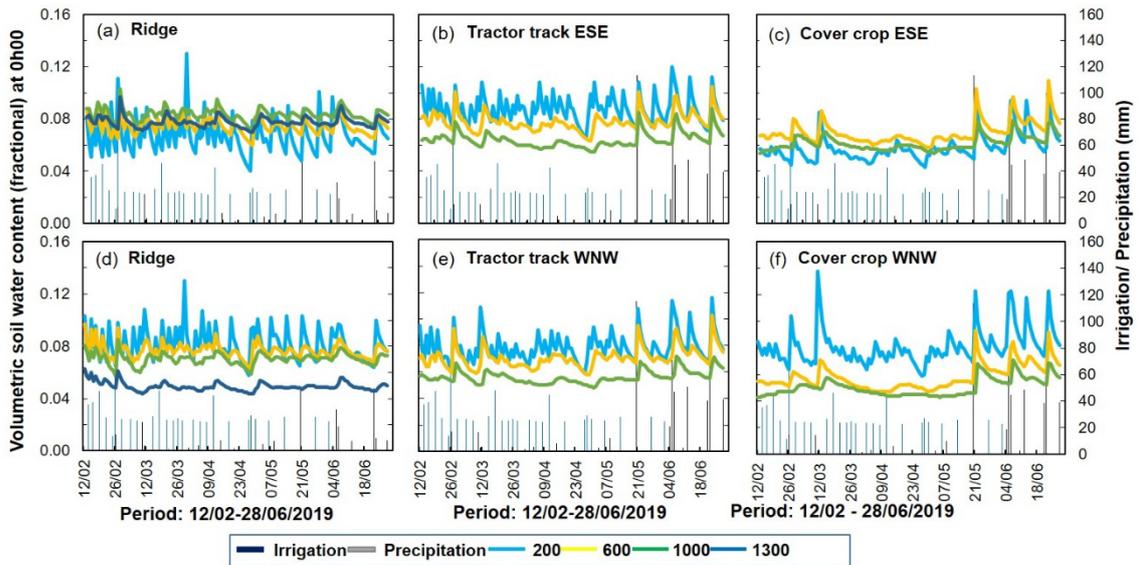
Figure 54 Soil water dynamics for the ridge (a & d), tractor track (b & e) and cover crop (c & d) on the east-south-east (b & c) and west-north-west (e & f) sides of the tree row in the fixed net section of the orchard from February until June 2019. Volumetric soil water content for the different soil depths (mm) is based on the sensor factory calibration.
