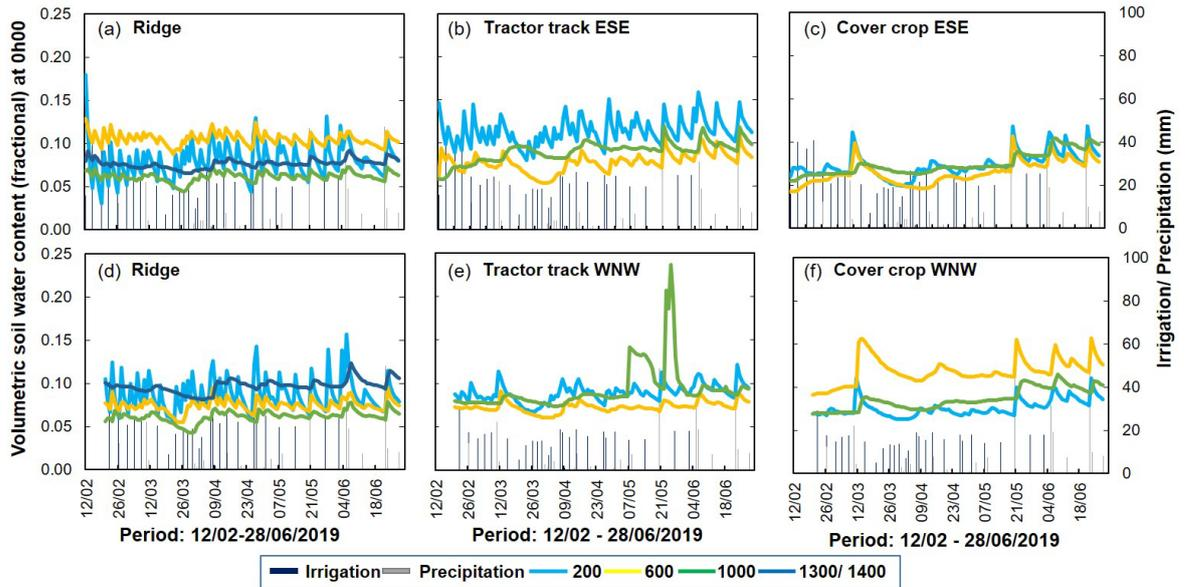
Figure 53 Soil water dynamics for the ridge (a & d), tractor track (b & e) and cover crop (c & d) on the east-south-east (b & c) and west-north-west (e & f) sides of the tree row in the open section of the orchard from February until June 2019. Volumetric soil water content for the different soil depths (mm) is based on the sensor factory calibration. The deepest soil layer in (c) and (d) is 1300 and 1400 mm, respectively.
