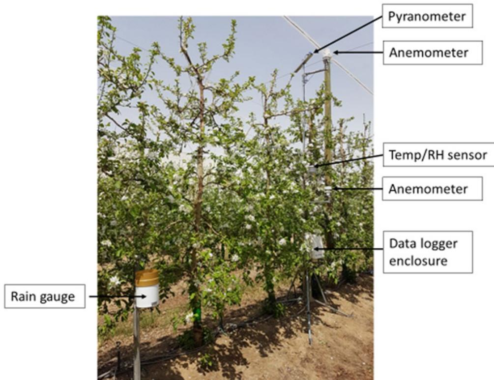
Figure 24 Automatic weather station measuring basic weather elements in the orchard under fixed white shade netting.
