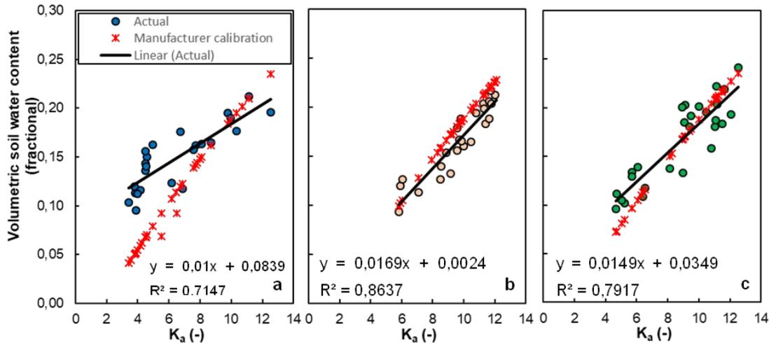
Figure 144 Comparison of CS650 manufacturer calibrated soil water content and actual volumetric soil water content sampled simultaneously at the 150 mm depth at various dielectric permittivities for the tree row (a, n=24), tractor track (b, n= 24) and cover crop areas (c, n=27). Data were combined for all four soil water balance installations.
