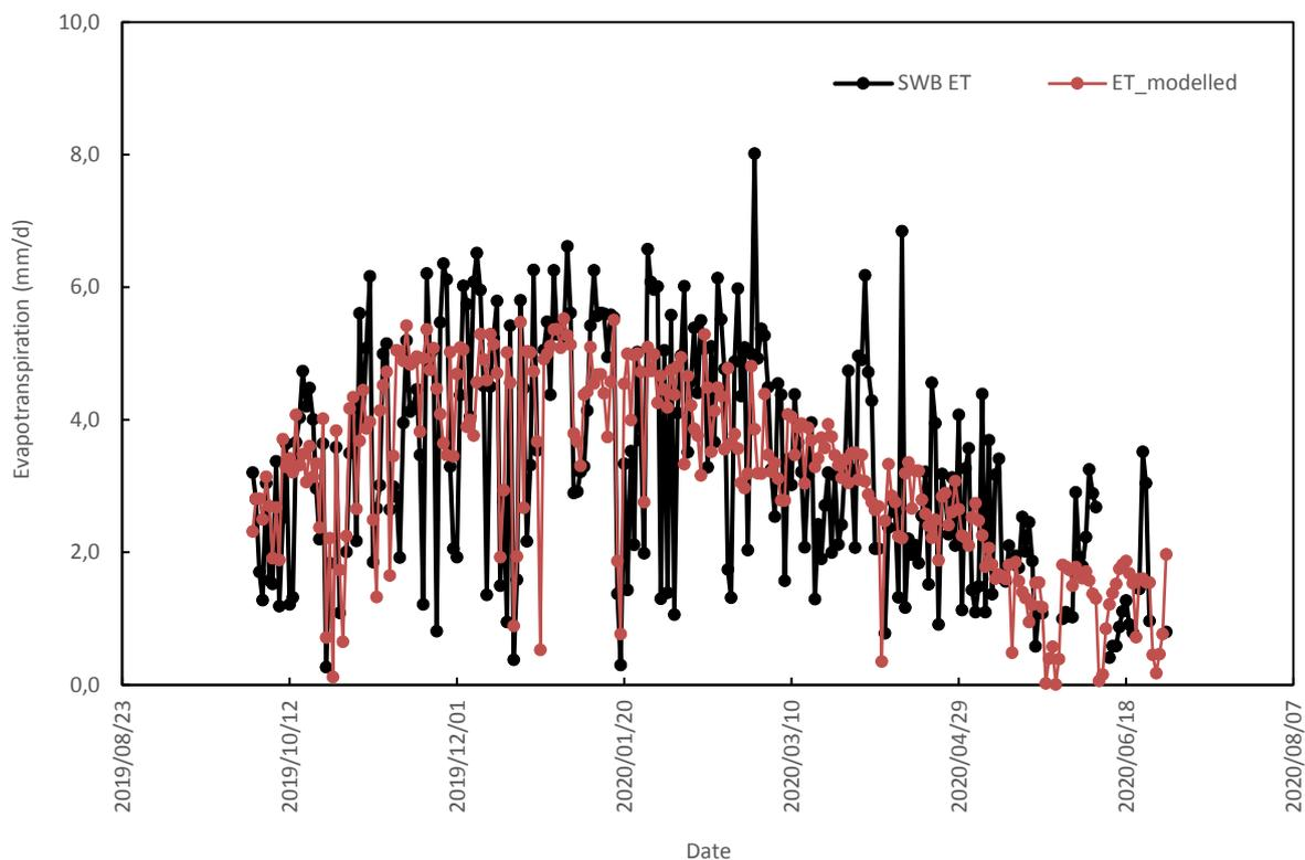
Figure 78 Comparison of evapotranspiration of the control treatment at the fixed net site determined using the soil water balance and dual source model.
