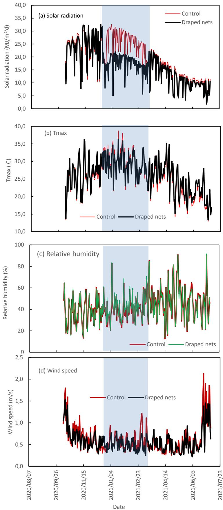
Figure 101 Effect of the draped nets on the canopy microclimate representing (a) the solar radiation, (b) maximum temperature, (c) minimum relative humidity, and (d) wind speed.
