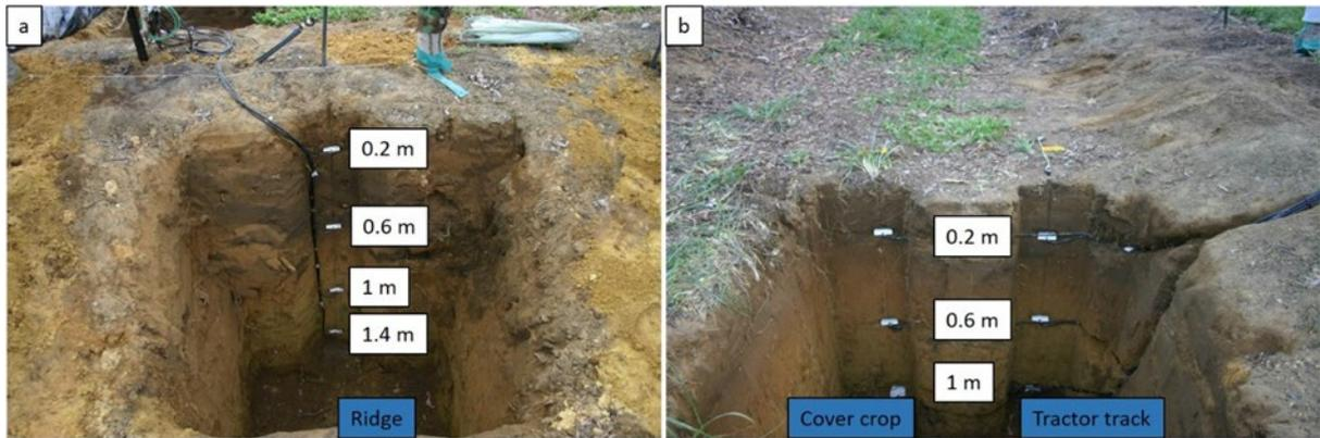
Figure 36 Soil water balance equipment installed in (a) the ridge and (b) the cover crop and tractor track in sandy soil in a ridged 'Golden Delicious Reinders' orchard at the draped net site at Paardekloof in 2019-2020. The installation depths of the CS616 sensors are indicated.
