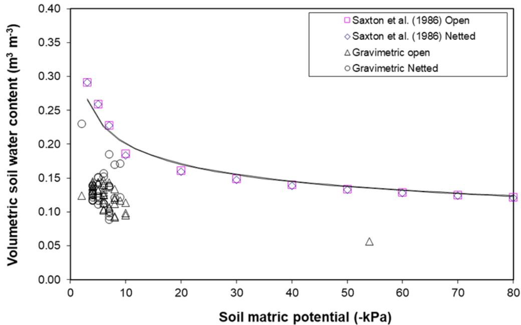
Figure 52 Comparison of estimated soil water retention curves of a 1.2 m sandy soil profile in the open and below net at the 'Rosy Glow' fixed net orchard, with gravimetric samples taken to establish in situ retention curves. The soil water retention curves were estimated from profile averaged soil texture according to Saxton et al. (1986).
