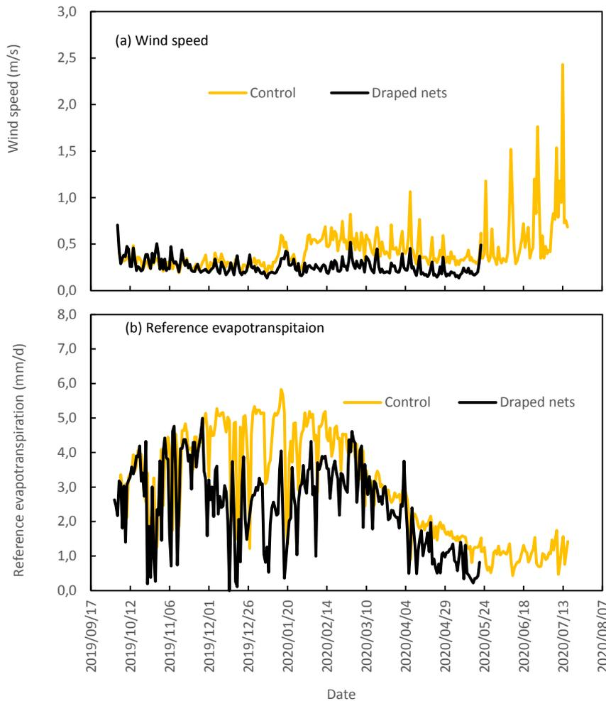
Figure 100 Effect of draped nets on; (a) the wind speed, and (b) reference evapotranspiration.
