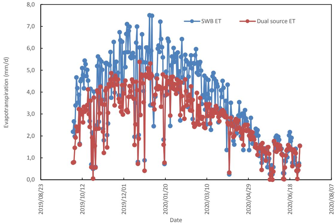
Figure 82 Comparison of the soil water balance with the modelled evapotranspiration under fixed nets.
