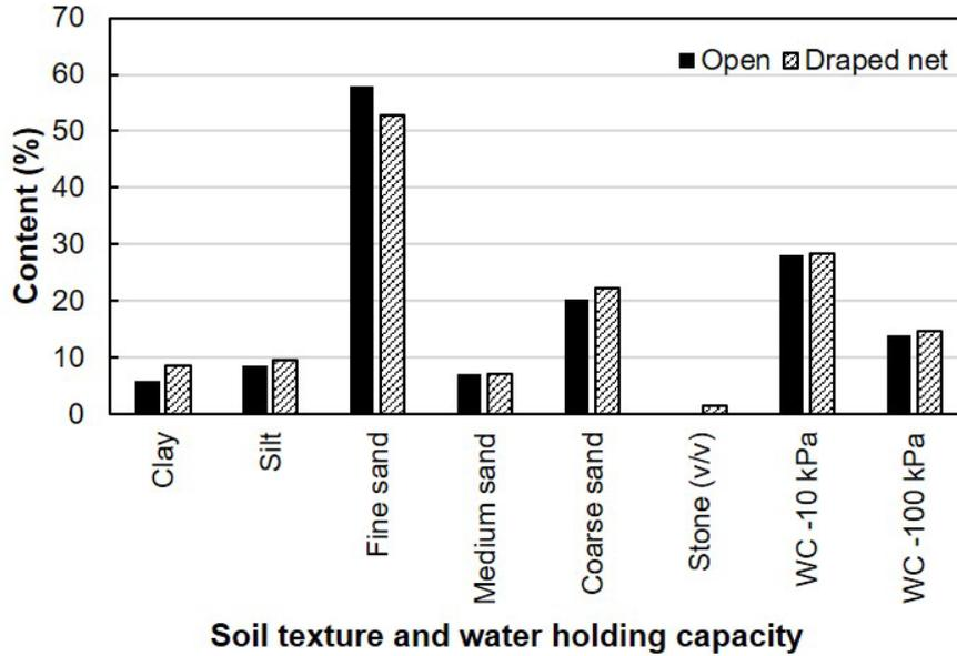
Figure 104 Soil particle size distribution and water content (WC) at -10 kPa and -100 kPa for the open (control) and draped net areas in the 'Golden Delicious Reinders' orchard at Paardekloof in 2019-2020. Soils were sampled in the ridge and data averages represent the soil profile up to a 1.2 m depth.
