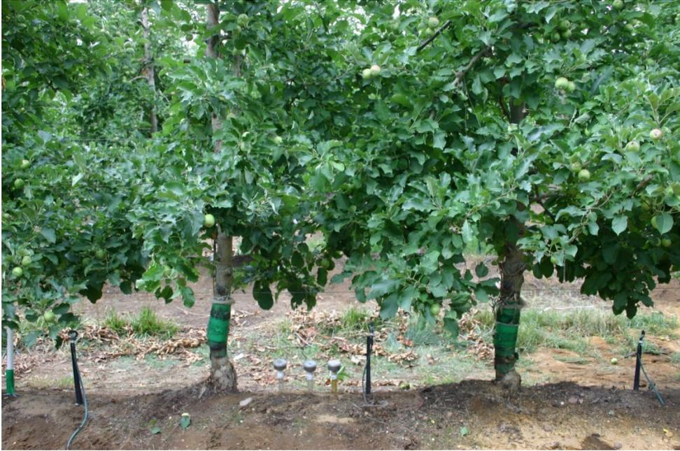
Figure 31 Tensiometers installed in the centre of the ridge between the tree stem and microsprinkler at 300, 600 and 900 mm depths in sandy soil in the 'Rosy Glow' orchard at Paardekloof in 2018.
