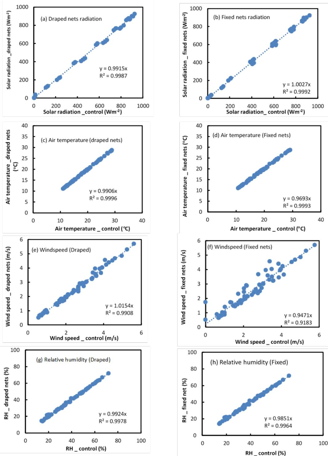
Figure 136 Calibration comparison of the (a) solar radiation, (c) air temperature, (e) wind speed, and (g) relative humidity of the weather station deployed under the draped nets with that in the control treatment. Figures (b), (d), (f) and (h) represents the climate variables for the fixed nets weather station. Data was collected from 26-29 September 2019.
