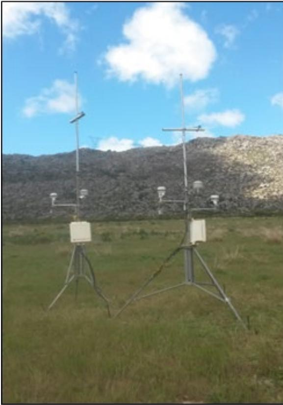
*Figure 23. Cross calibration of the two automatic weather stations to establish systematic errors among the sensors prior to the 2018-2019 season.*
