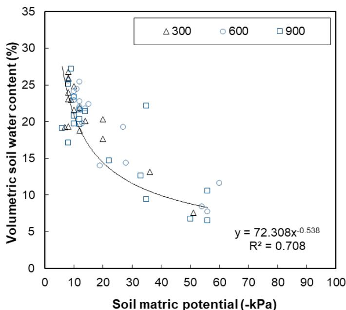
Figure 106 Soil water retention curve determined for a 0.9 m sandy loam to loamy sand soil profile at the 'Golden Delicious Reinders' draped net orchard, with gravimetric samples taken from the open and draped netting sections to establish the *in situ* retention curve.
