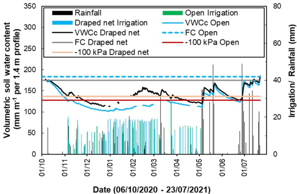
Figure 115 Soil water dynamics for the open and draped net sections from October 2020 until July 2021. Volumetric soil water content for the orchard was averaged taking the tree row, tractor track and cover crop surface area into account. The volumetric soil water content is based on in situ calibration and are for two replicates. The field capacity (FC) was determined in situ and the -100 kPa values are derived from soil particle size analysis (Bemlab).
