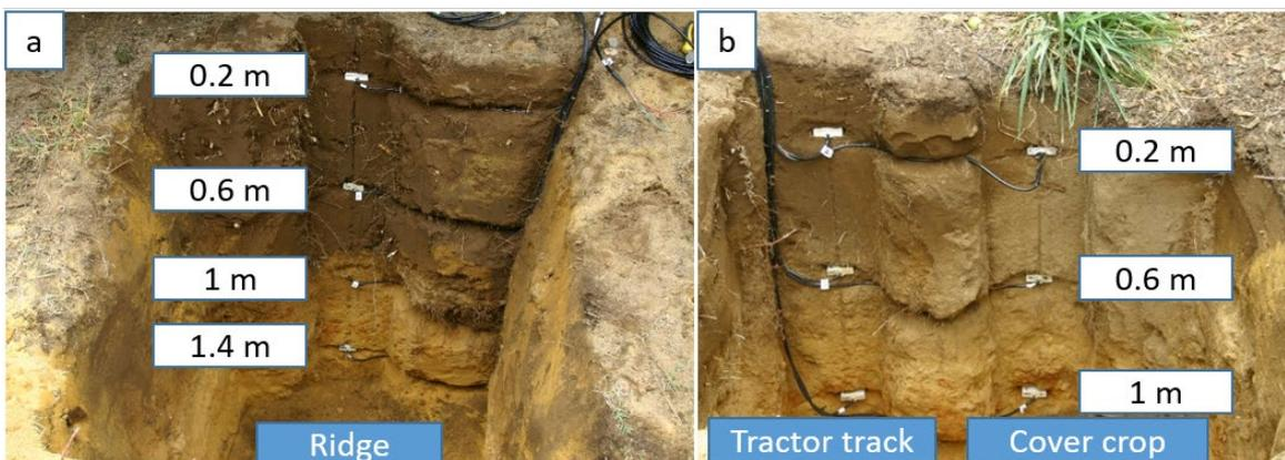
Figure 33 Soil water balance equipment installed in (a) the ridge and (b) the tractor track and cover crop in sandy soil in a ridged 'Rosy Glow' orchard at Paardekloof in 2018-2019. The installation depths of the CS650 and/ or CS616 sensors in the ridge, tractor track and work row area with cover crop are indicated.
