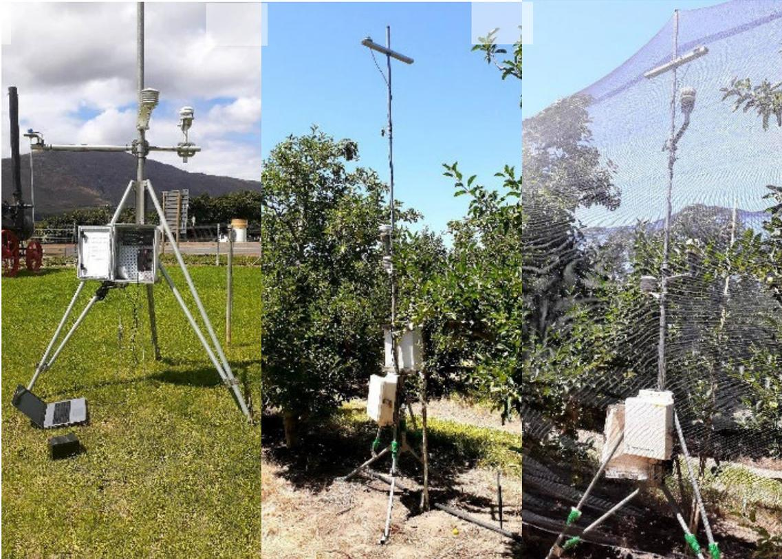
Figure 28. Automatic weather stations measuring basic weather elements: Left: at the Vilko hardware store site just outside Villiersdorp, about 2 km from the orchard; Middle: in the control treatment rows of the study orchard; Right: under the draped netting in the study orchard.
