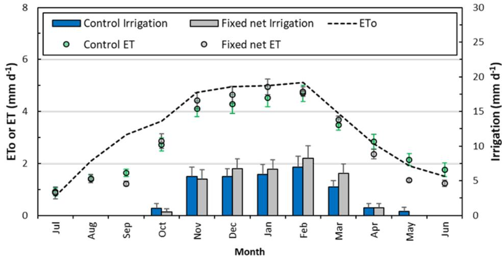
Figure 72 Monthly averaged Penman-Monteith reference evapotranspiration ( $ET_0$ ), 'Rosy Glow' orchard evapotranspiration (ET) and irrigation applied in the open (Control) and below fixed net at Paardekloof. Error bars indicate the standard error.
