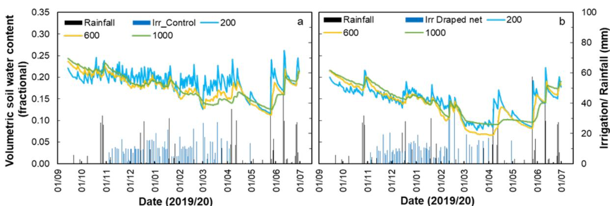
Figure 108. Soil water content (midnight) dynamics for the 'Golden Delicious Reinders' (a) control treatment and (b) draped net treatment averaged over orchards areas at the 200 mm, 600 mm and 1000 mm depths for the period 14/09/2019-30/06/2020 during the 2019-2020 season.
