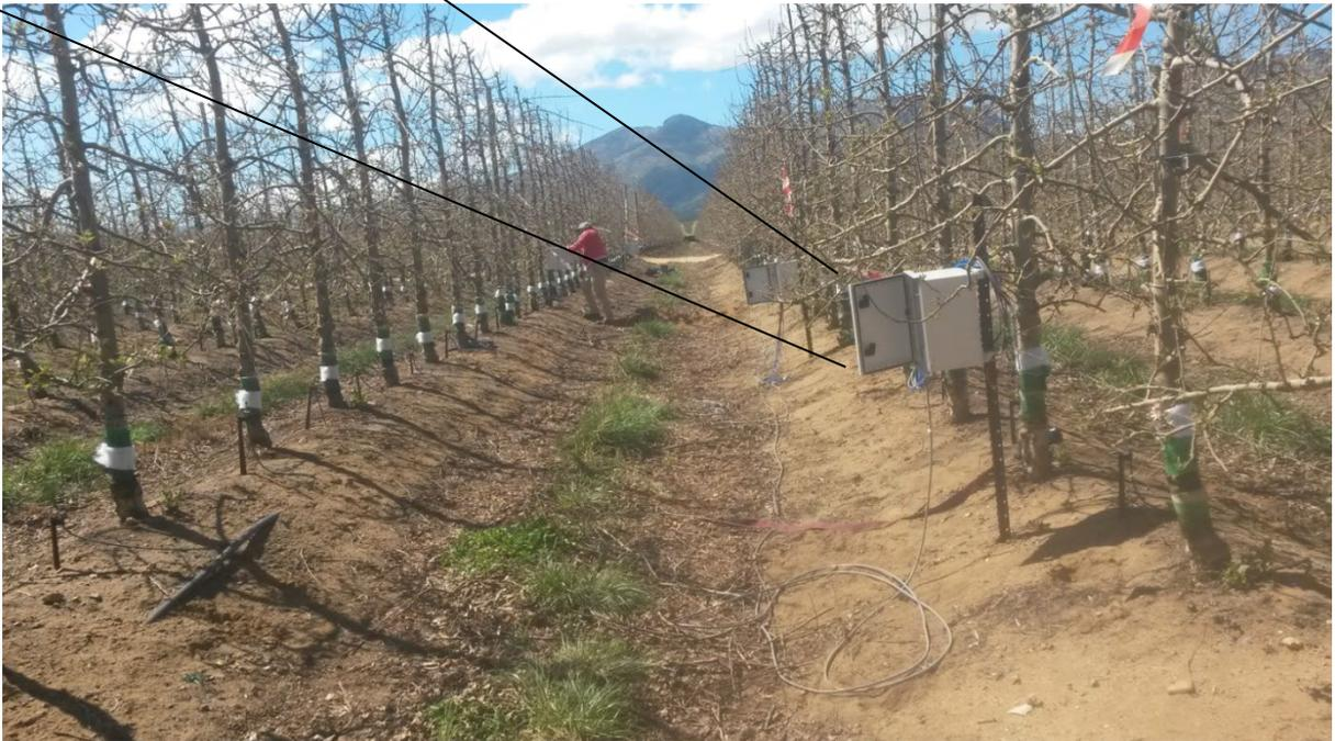
*Figure 39 The improved heat pulse velocity sap flow system being used to monitor actual water use by the trees (transpiration,  $T$ ) in the open and fixed shade netting trial. The insert shows an individual tree box.*
