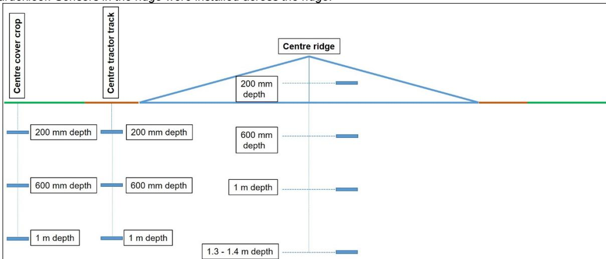
Figure 138 Illustration of the position and depths of the CS650 and/ or CS616 sensors (blue blocks) installed in soil relative to ridged 'Rosy Glow' and 'Golden Delicious Reinders' trees at Paardekloof.
