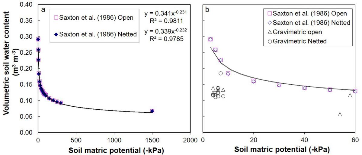
Figure 51. Comparison of a) soil water retention curves of a 1.2 m sandy soil profile in the open and under net at Paardekloof and b) estimated curves with gravimetric samples taken to establish *in situ* retention curves. The soil water retention curves were estimated from profile averaged soil texture according to Saxton et al. (1986).
