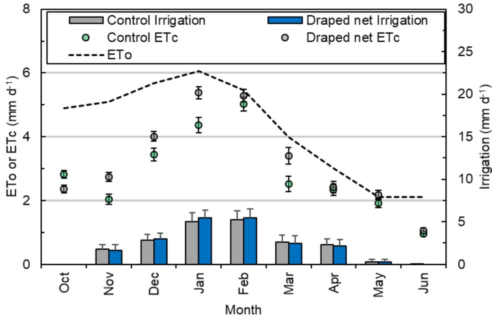
Figure 125. Monthly averaged Penman-Monteith reference evapotranspiration ( $ET_o$ ), 'Golden Delicious' orchard evapotranspiration (ET) and irrigation applied in the open (Control) and below draped net at Southfield. Error bars indicate the standard error.
