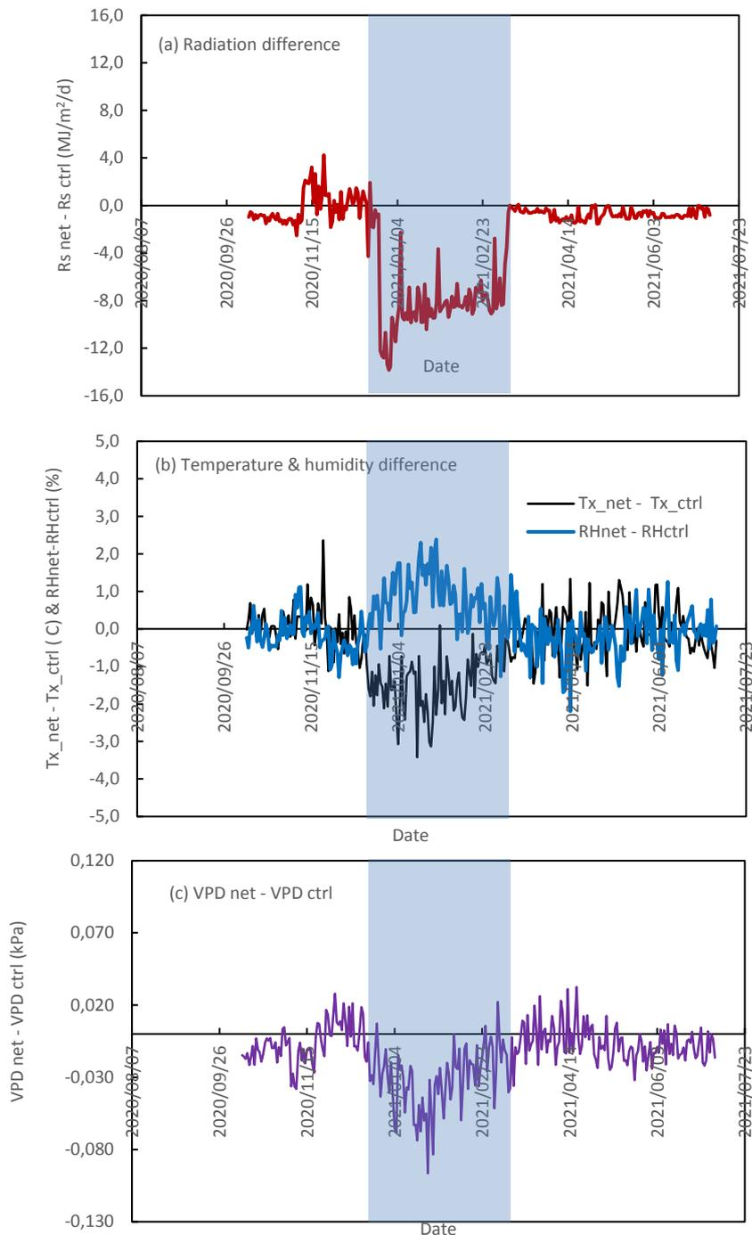
Figure 102 Differences in the microclimate between the draped nets and control treatments representing (a) the solar radiation, (b) air temperature and relative humidity, and (c) vapour pressure deficit of the air.
