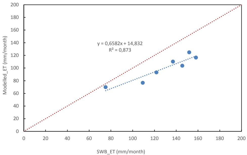
Figure 83 Comparison of monthly total evapotranspiration determined using the soil water balance approach and modelled using the dua source model.
