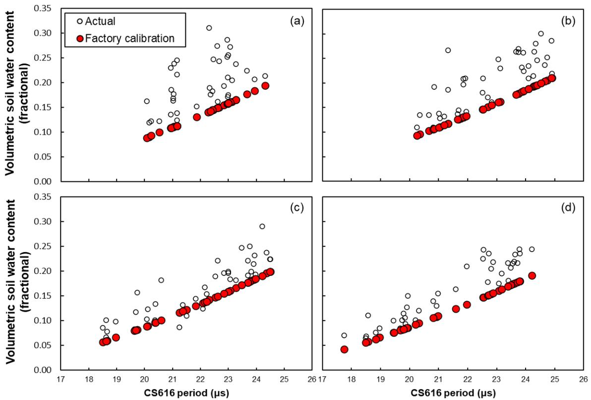
Figure 143 Comparison of CS616 factory calibrated soil water content and actual volumetric soil water content sampled simultaneously for various CS616 periods at the control treatment soil water balance replicate 1 (a) and 2 (b) and for the draped net soil water balance replicate 1 (c) and 2 (d) in the 'Golden Delicious Reinders' orchard at Paardekloof.
