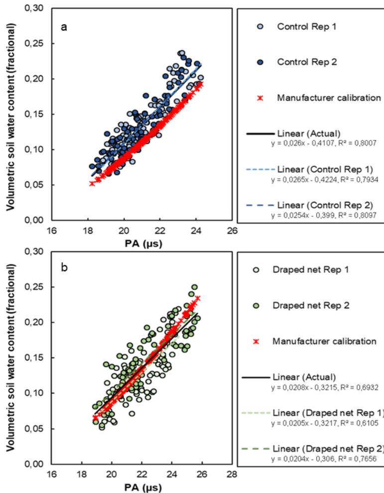
Figure 145 Comparison of CS616 factory calibrated soil water content and actual volumetric soil water content sampled simultaneously at various CS616 periods at (a) soil water balance replicate 1 and 2 for the control treatment (n=170) and (b) soil water balance replicate 1 and 2 for the draped net treatment (n=162).
