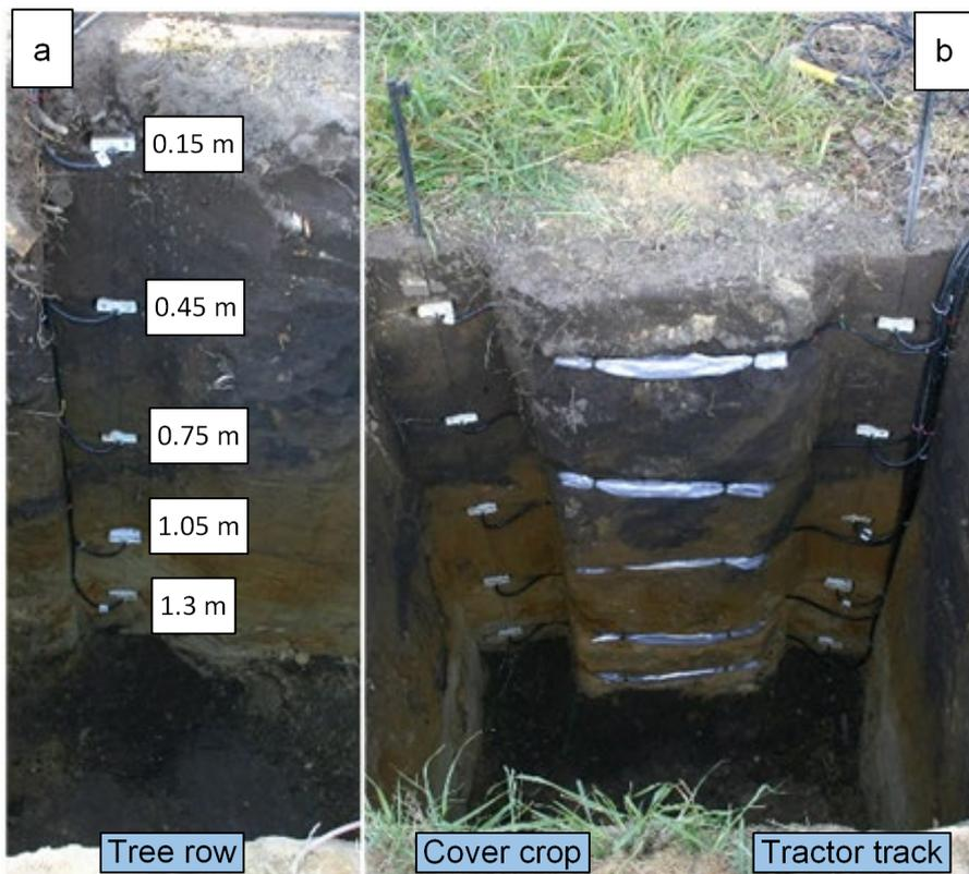
Figure 38. Soil water balance equipment installed in (a) the tree row and (b) the work row with cover crop and tractor track in sandy loam soil in a 'Golden Delicious' orchard at Southfield in 2020-2021. The installation depths of the CS650 and/or CS616 sensors in the tree row, cover crop and tractor track area are indicated in (a).
