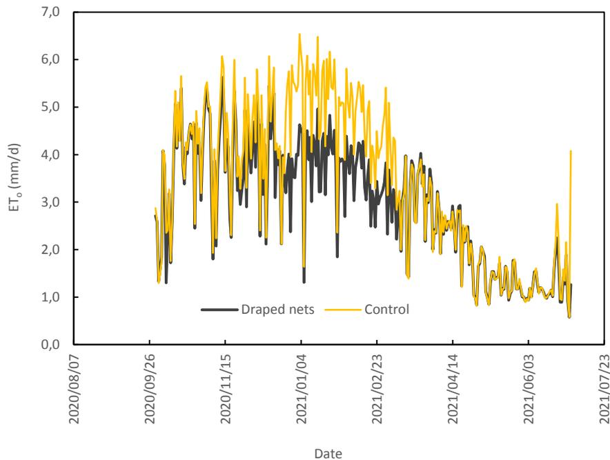
Figure 103 Effect of the draped nets on the reference evapotranspiration at Southfield.
