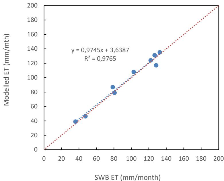
Figure 79 Monthly orchard water requirements determined by the dual source ET model and the soil water balance approach at the fixed nets site.
