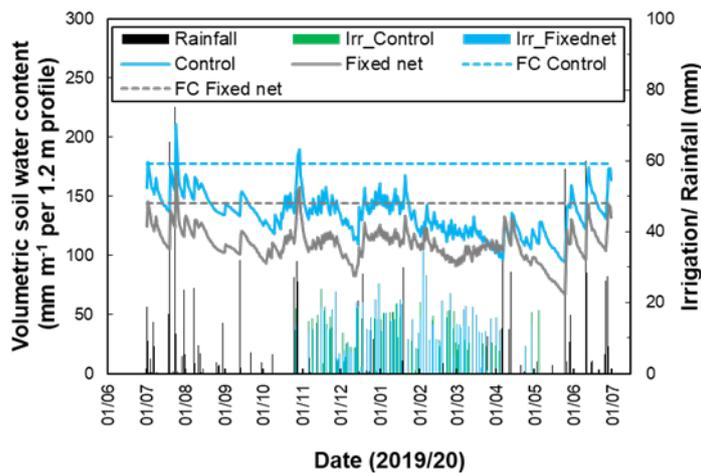
Figure 59 Soil water content (midnight) dynamics, rainfall and irrigation applied for the ‘Rosy Glow’ control and fixed net treatments for the period 01/07/2019–30/06/2020 during the 2019–2020 season. The field capacity (FC) values determined from hourly soil water content graph trends are also indicated.
