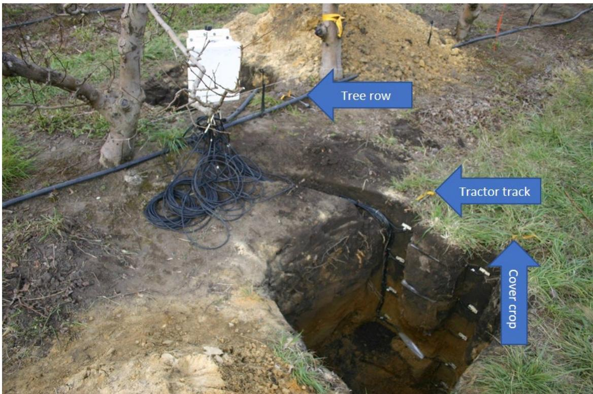
Figure 37. Installation positions of CS650/CS616 sensors in sandy soil in the 'Golden Delicious' orchard at Southfield in 2020-2021. White rope and yellow labels on the soil surface indicate the relative positions of the sensors.
