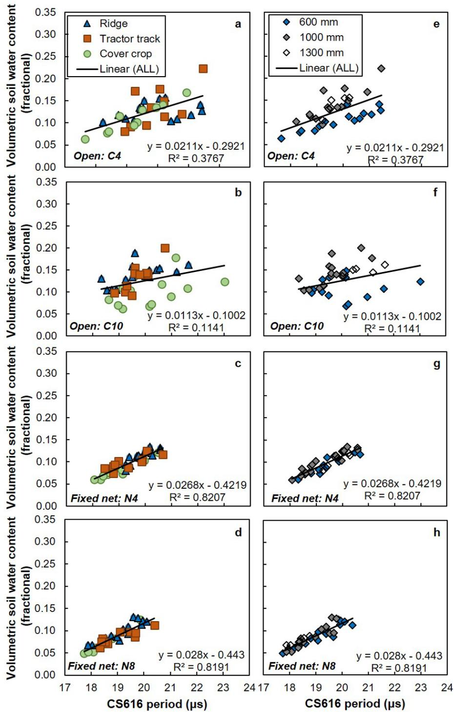
Figure 142 Comparison of gravimetrically sampled volumetric soil water content to the CS616 soil water content sensor period ( $\mu\text{s}$ ) for orchard areas combined (a-d) and over measurement depths (e-h) per soil water balance site (C4, C10, N4, N8) for the open (a, b, e, f) and fixed net (c, d, g, h) sections of the 'Rosy Glow' orchard during 2018-2019 and 2019-2020.
