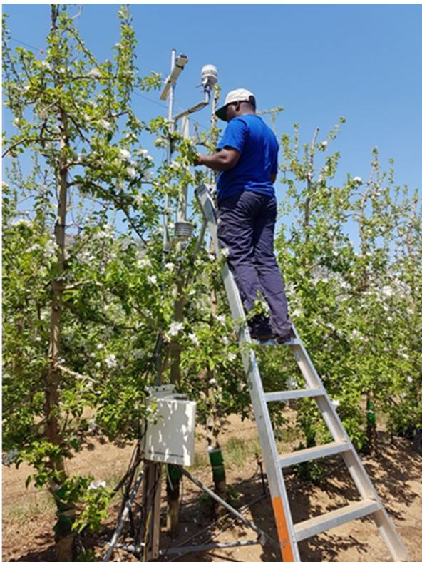
Figure 25 Automatic weather station measuring basic weather elements in the open orchard. Installation is being conducted by the PhDAgric student, Mr Edward Lulane, on 9 October 2018 (full bloom).
