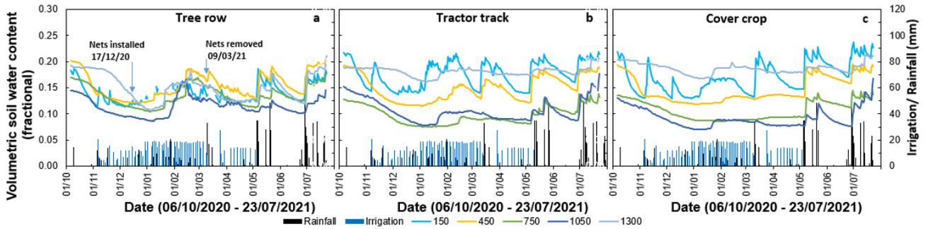
Figure 114 Soil water dynamics for the tree row (a), tractor track (b) and cover crop (c) in the draped net section of the orchard from October until July 2021. Volumetric soil water content for the different soil depths (mm) is based on in situ calibration and are for two replicates.
