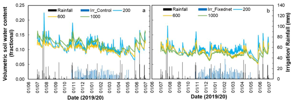
Figure 58 Soil water content (midnight) dynamics for the 'Rosy Glow' (a) control and (b) fixed net treatments averaged over orchards areas at the 200 mm, 600 mm and 1000 mm depths for the period 01/07/2019-30/06/2020 during the 2019-2020 season.
