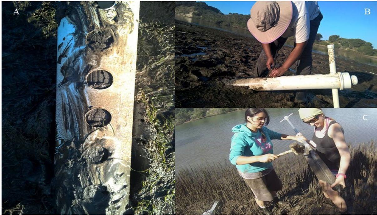
**Plate 3.1.1.** **A)** An example of an extracted sediment core using a PVC pipe with pre-drilled holes. **B)** Extracting a subsample from the core using a syringe. **C)** A sediment core extracted from a mangrove plot using a Russian Peat Corer. Photos: S. Mbense and J. Raw, 2017.
