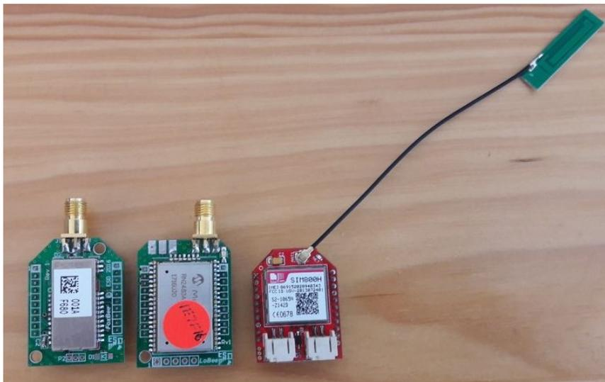
**Figure 4.6:** The different communication modules developed. The one on the left is for the SigFox network, the one in the middle is for the LoRa network and the one on the right is a GSM modem that could be used for GPRS or ThingStream.
