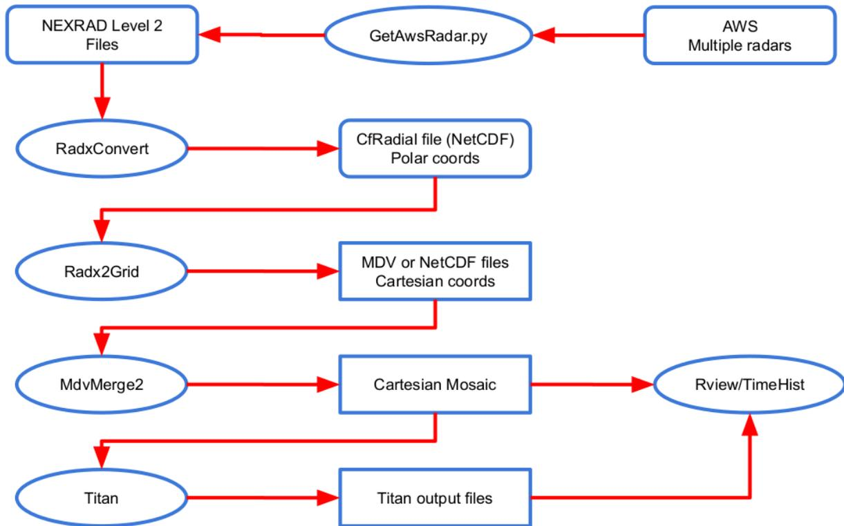
**Figure 4.18: The LROSE process flow, merging different radars**
