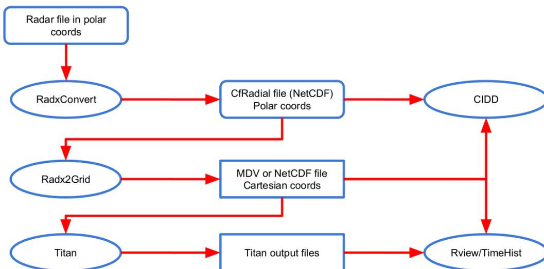
Figure 4.17: The legacy processes used in a typical TITAN application
