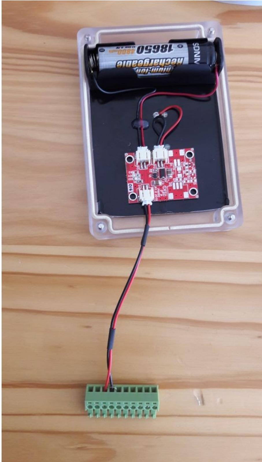
**Figure 4.8:** The low-cost logger power module that features a rechargeable battery and a small solar panel
