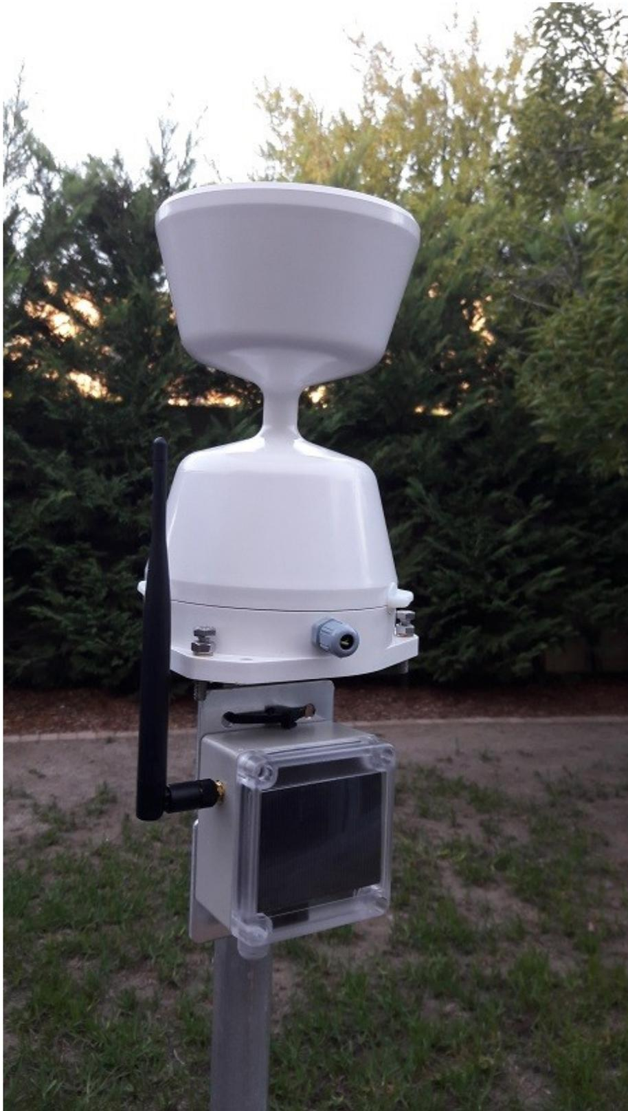
**Figure 4.9:** The lowest-cost logger, modem and low-cost rain gauge developed for the project. This combination costs approximately R5,000.
