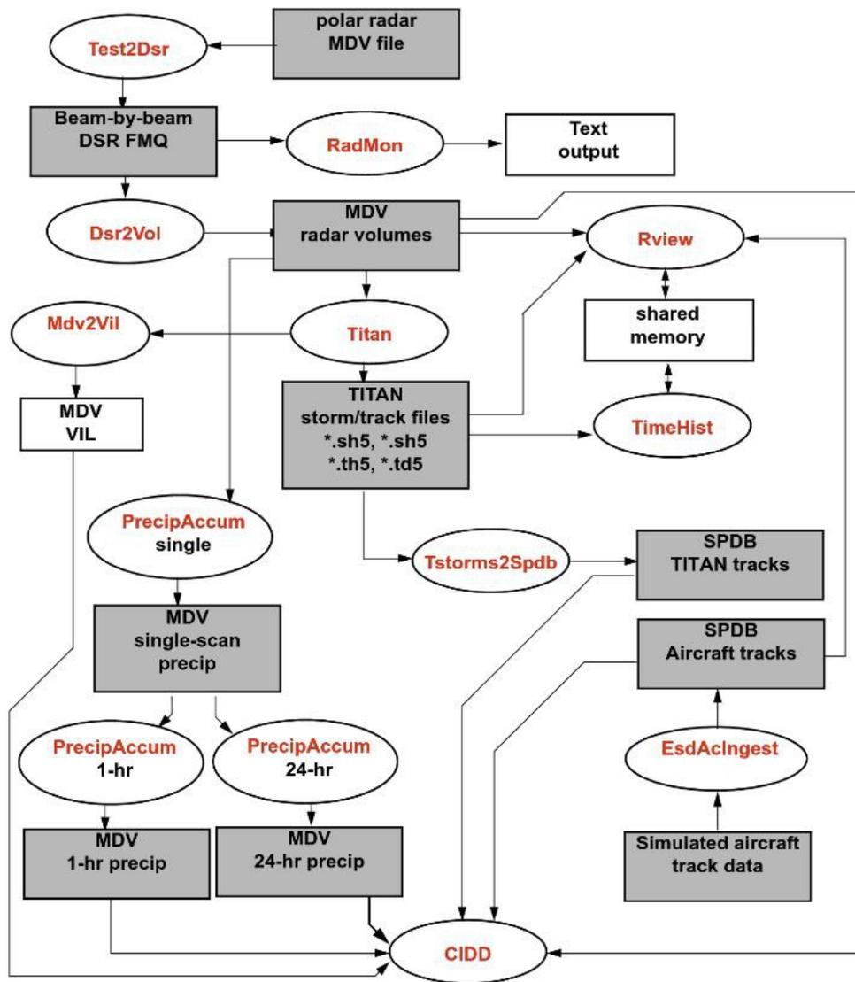
Figure 4.15: The legacy processes used in a typical TITAN application
