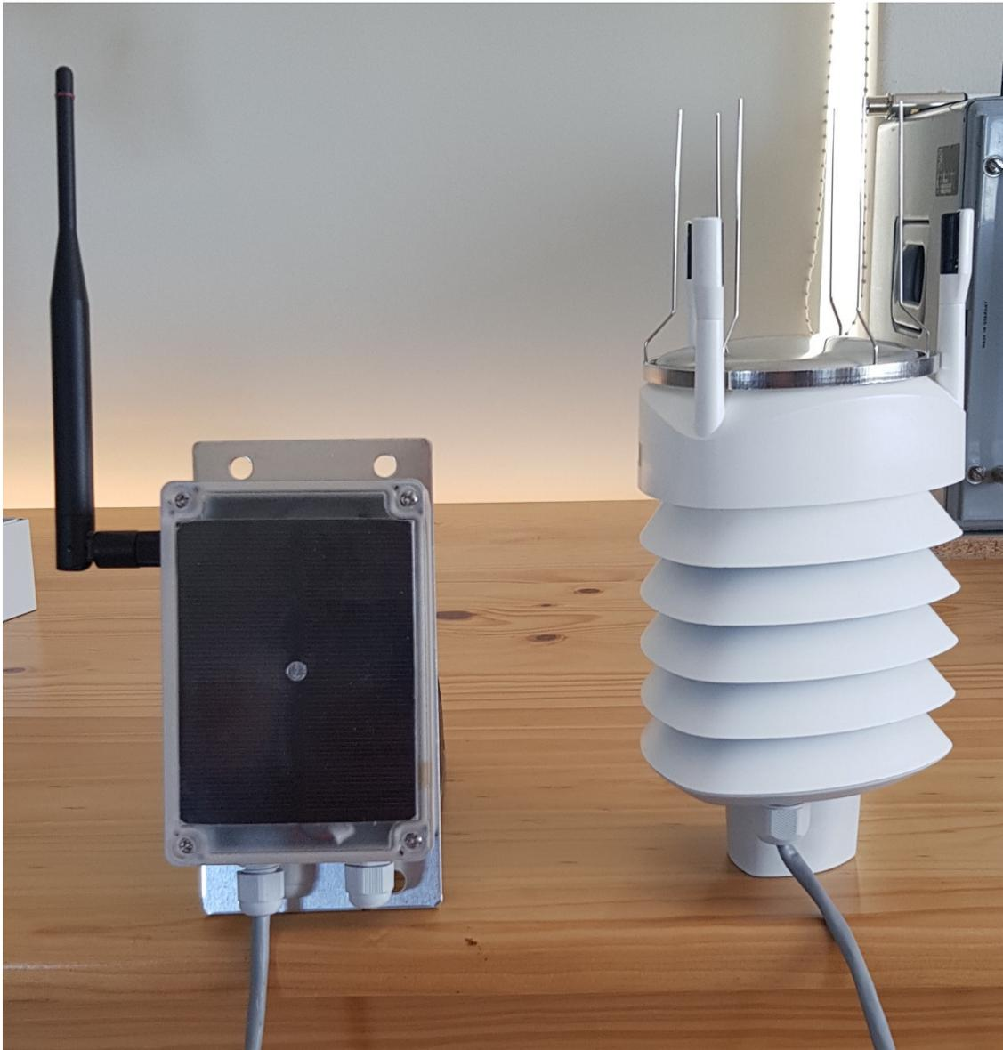
**Figure 4.11: The logger, modem and mid-range weather station developed for the project. This combination uses the Vaisala Multisensor WXT530. The combination costs approximately R50,000.**
