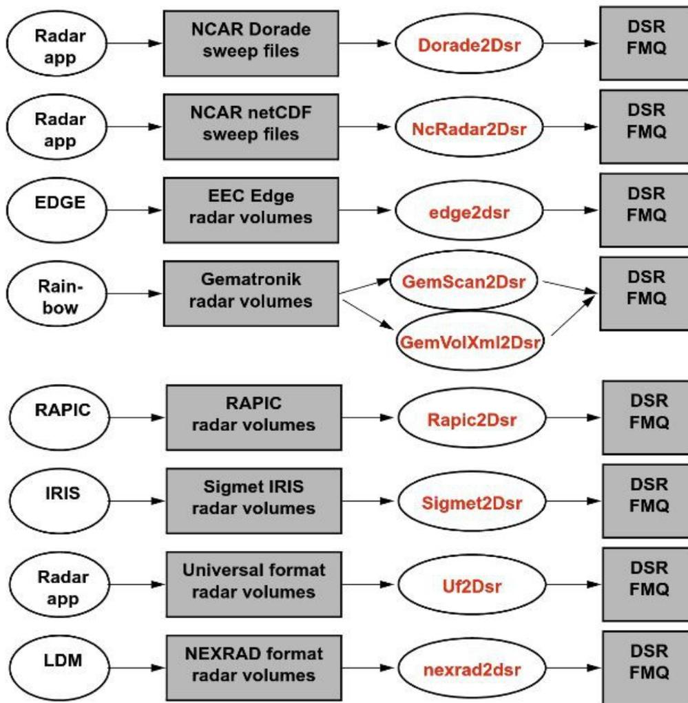
Figure 4.16: The legacy ingest processes used in a typical TITAN application
