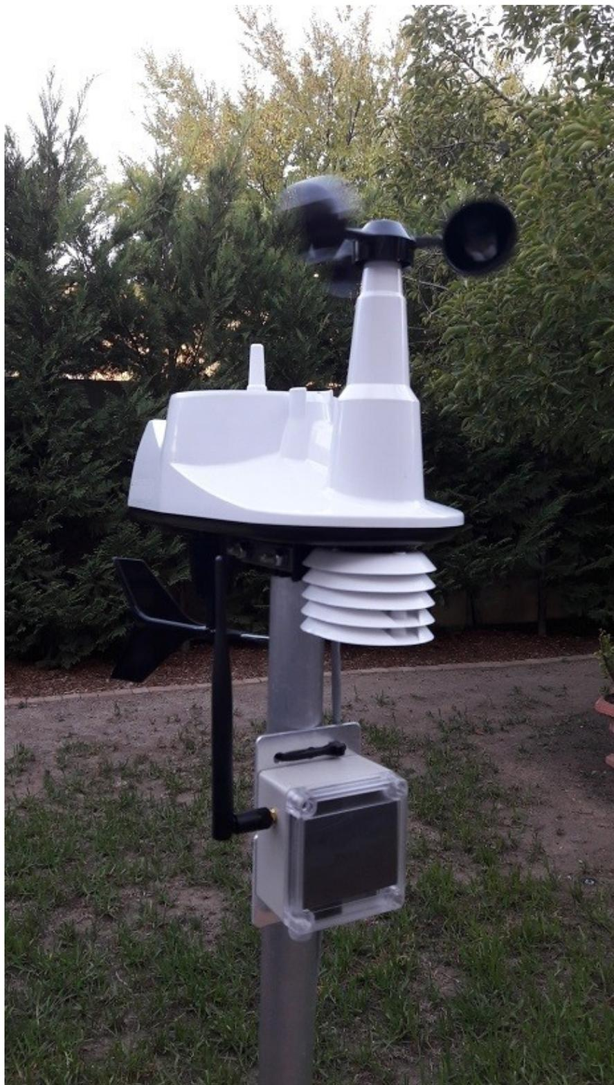
**Figure 4.10:** The logger, modem and low-cost weather station developed for the project. This combination costs approximately R8,000.
