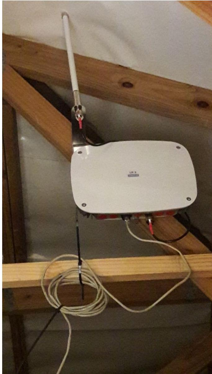
**Figure 4.2: A LORA gateway that creates a network working on near-line-of-sight and covers an area of approximately 60 km in radius, depending on the topography.**
