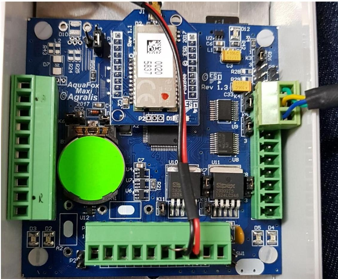
**Figure 4.7: The low-cost logger developed for the project**
