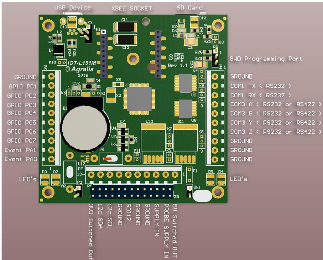
**Figure 4.5: The ESD L151M logger design**
