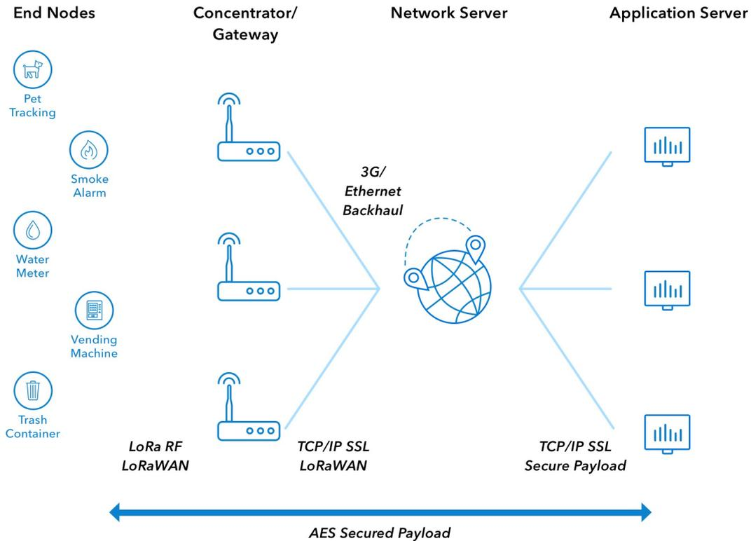
**Figure 4.1: The architecture of a LoRa WAN application (<https://www.thethingsnetwork.org>)**
