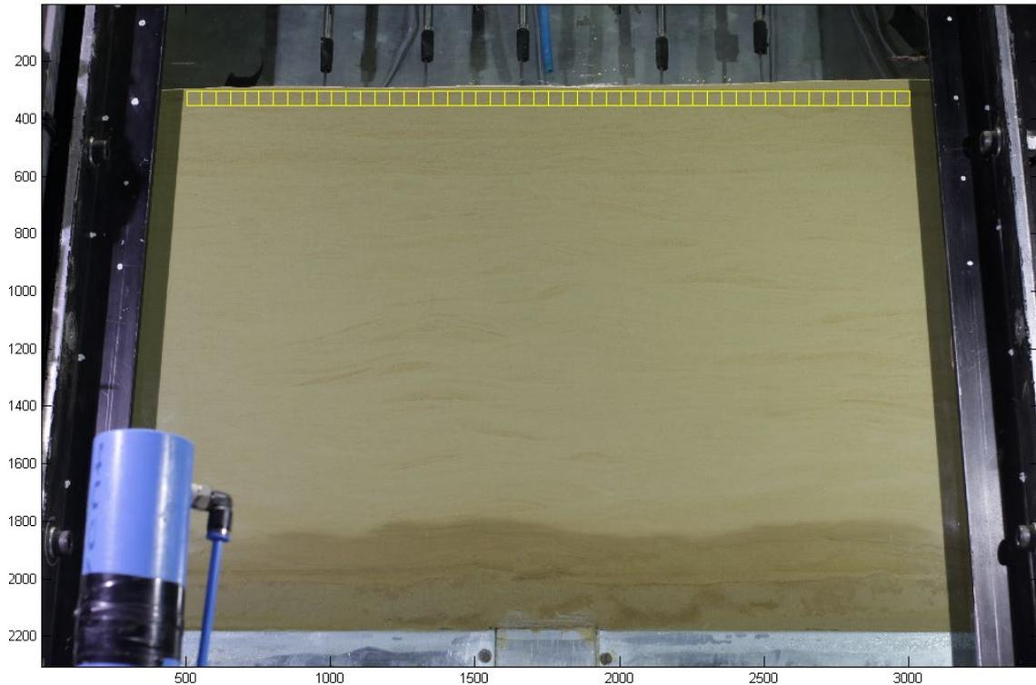
Figure 4-17: Row of patched tracked using PIV to study shape of leakage-induced surface settlement trough
