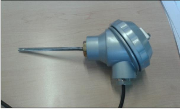
Figure 3-5: RTD 4 - 20 mA corresponding to >0-100°C output
