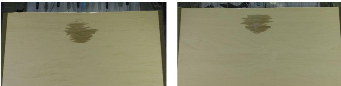
234 ml of water induced by simulated leak.
