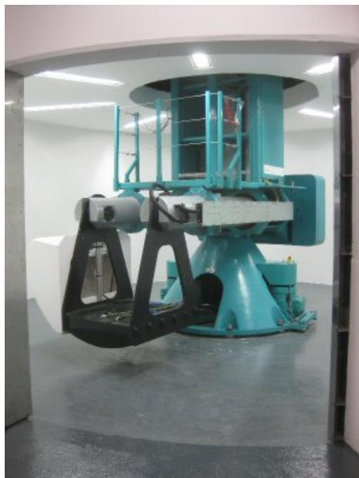
Figure 4-4: Geotechnical centrifuge of the University of Pretoria
