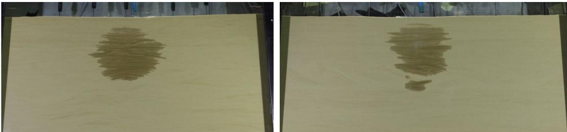
293 ml of water induced by simulated leak.
