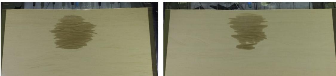
*Figure 4-20: Comparison of spreading of leakage-induced wetted zones under greenfield conditions (left) and with a pipe in the ground (right).*
