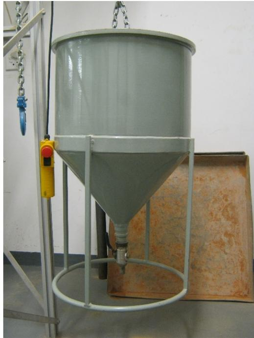
*Figure 4-11: Sand hopper used for placing silica sand in models*
