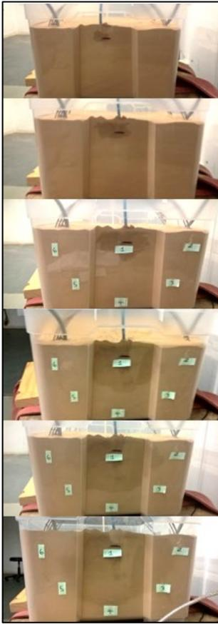
Figure 3-33: Advancing wetting front in laboratory test.
