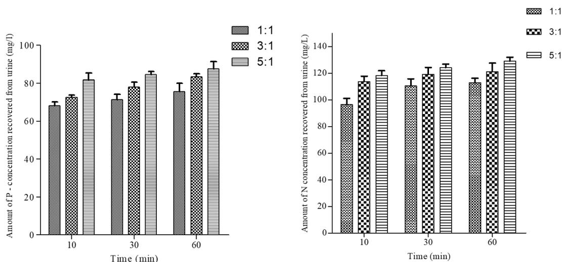
**Figure 10. Phosphorus and Nitrogen recovery from urine at different Mg: P concentrations.**
