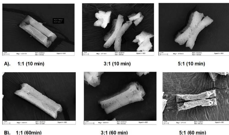
**Figure 12. Scanning electron microscope images showing particle morphology of struvite produced under different molar ratios of Mg:P at A) 10 minutes and B) 60 minute treatments.**
