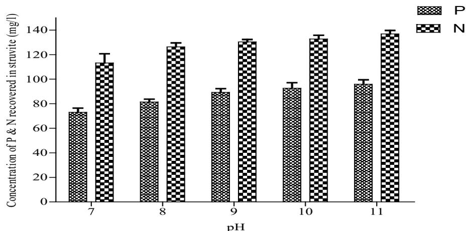
**Figure 11. Phosphorus and Nitrogen recovery from urine at different pH values.**
