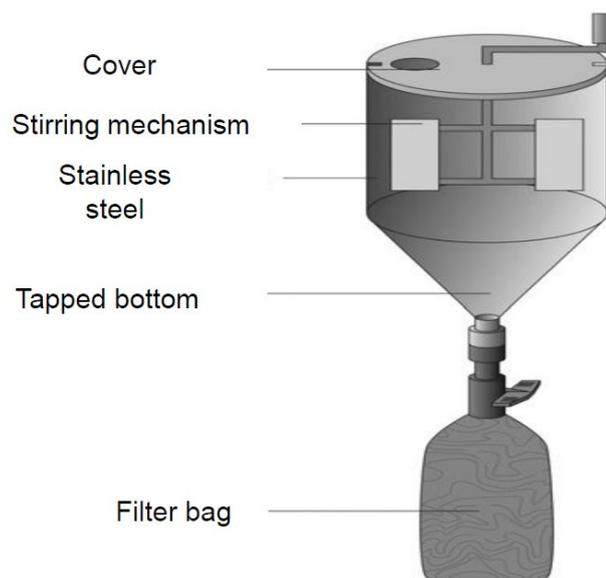
**Figure 1. Representation of the composition of the struvite reactor.**
