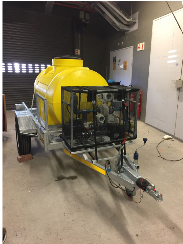
Figure 0.1: The pipe condition assessment equipment
