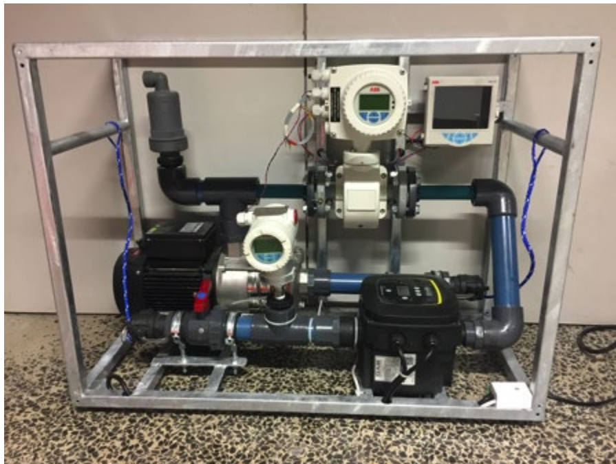
Figure 3.13: Constructed pipe condition assessment equipment
