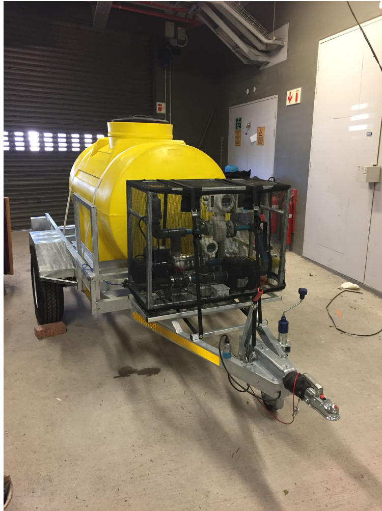
Figure 3.14: PCAE installed on a 1 000 ℓ water trailer
