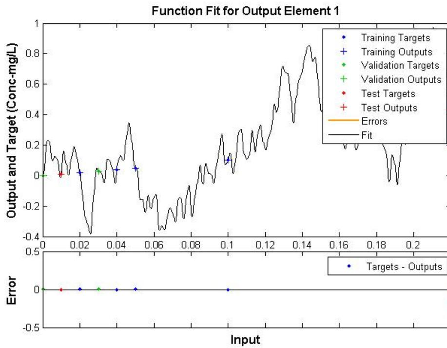
Figure 6.5: Function fit of the variation of the trace metals
