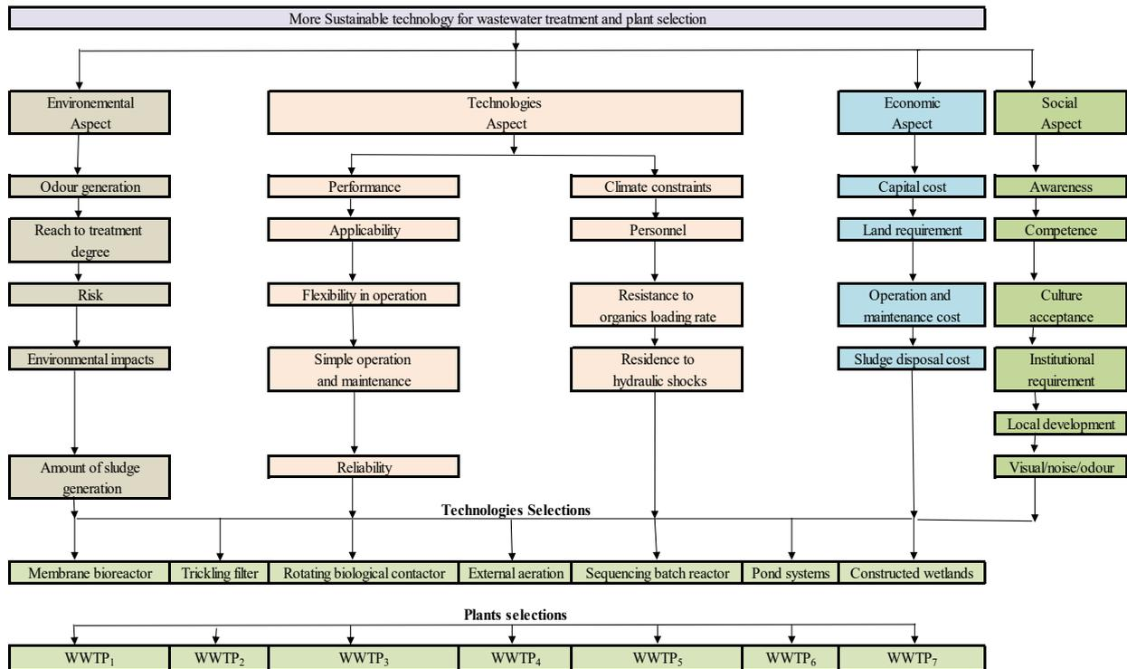
**Figure 3.3:** Multi-criteria decision analysis (MCDA) on the wastewater treatment process
