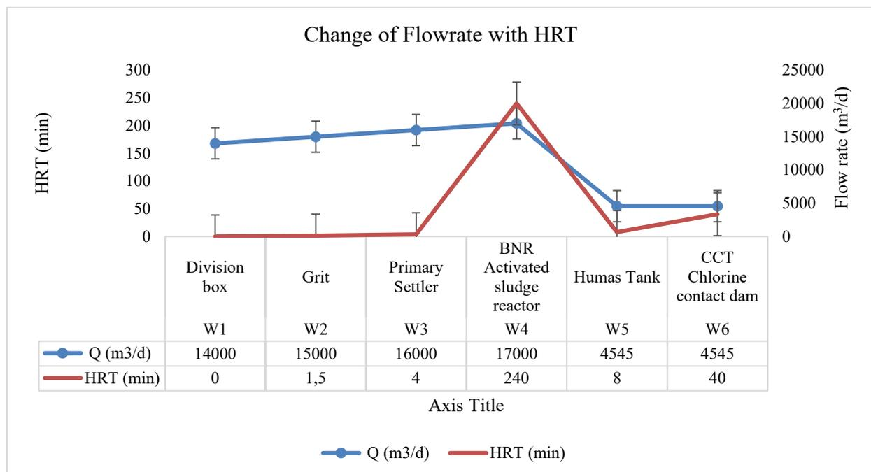
**Figure 4.1:** Change of flow rates with HRT in the activated sludge wastewater treatment plant
