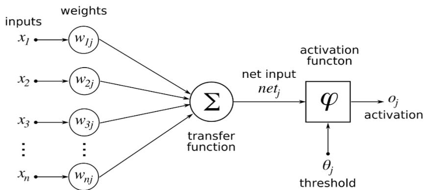
**Figure 6.2:** Schematic of the artificial neural network in AI-modelling using deep learning
