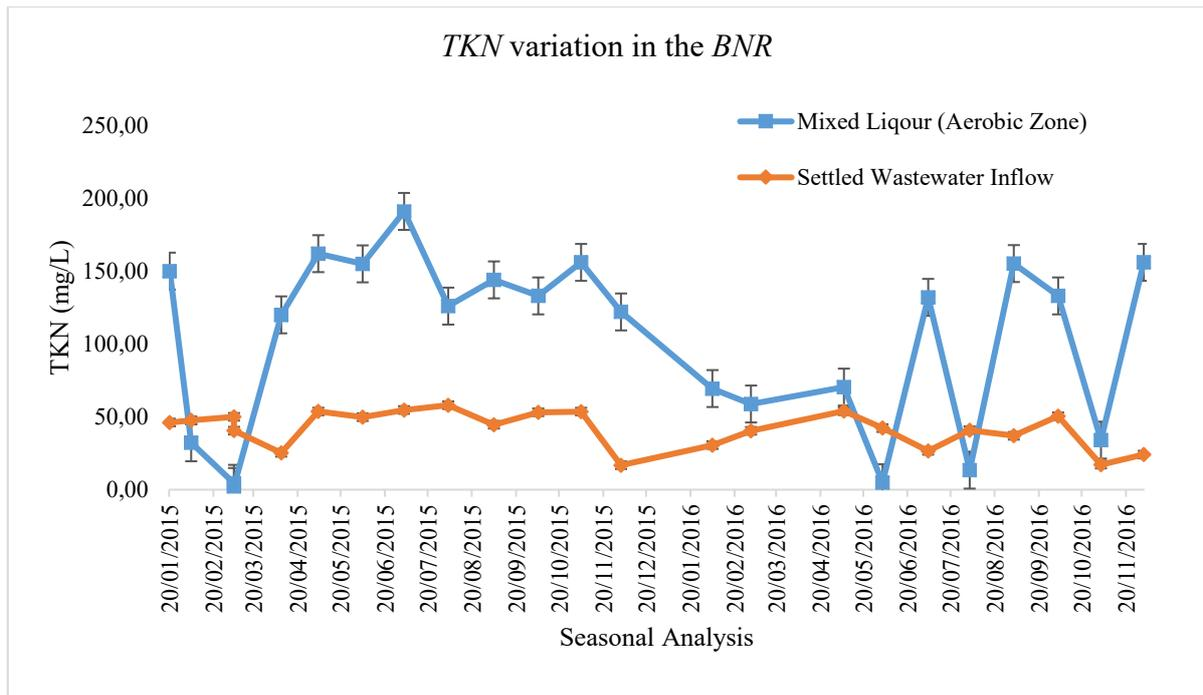
**Figure 4.24:** Variation of the TKN in the biological nutrient removal
