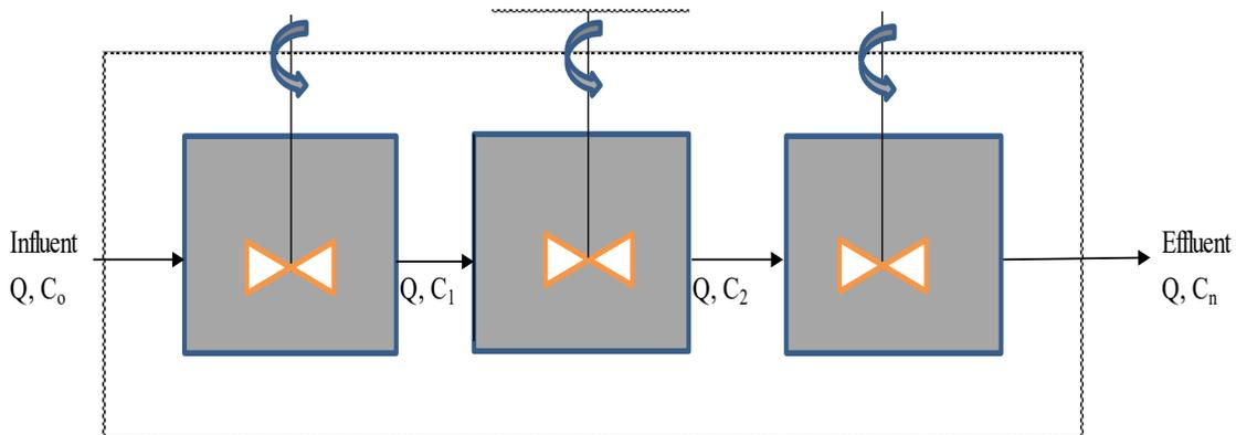
**Figure 5.1:** Completely mixed reactor in series in the WWTP
