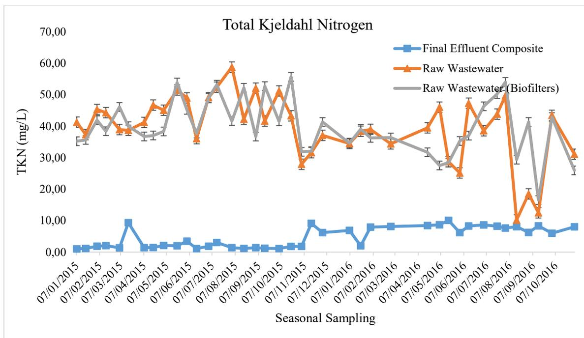
**Figure 4.23:** Seasonal variation of the total Kjeldahl nitrogen in the WWTP
