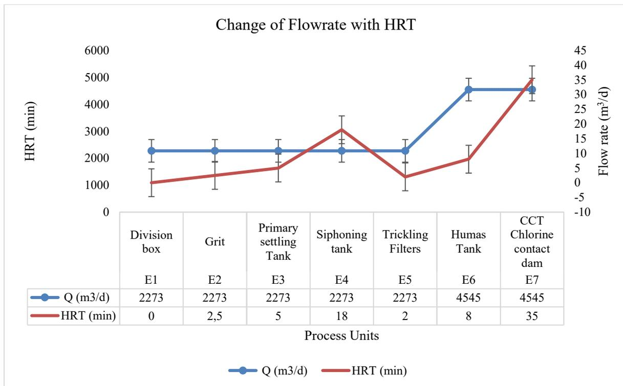
**Figure 4.2:** Change of flow rates and HRT in the biofilm wastewater treatment plant
