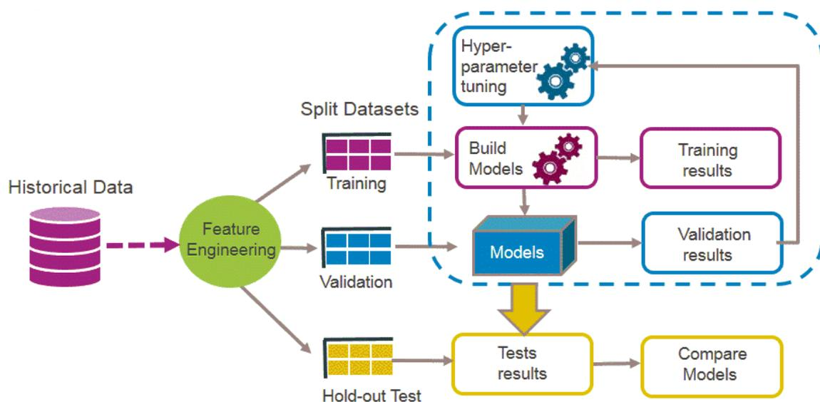
**Figure 6.1:** Flow diagram of the concept of deep learning (*machine learning*) with AI-modelling using artificial neural network
