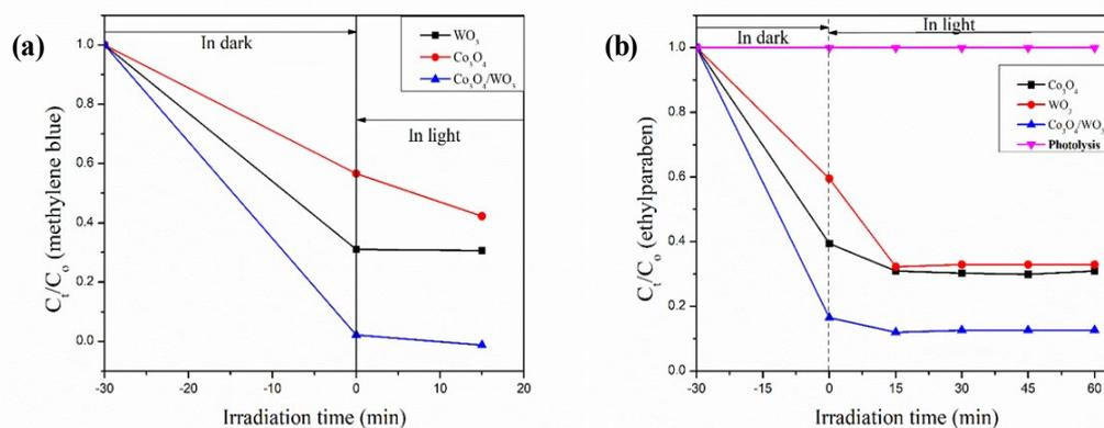
**Figure G1:** Adsorption and photodegradation of ethyl paraben (EP) and methyl blue (MB)  $Co_3O_4$ ,  $WO_3$ , and by Z-scheme  $Co_3O_4/WO_3$  nanocomposite
