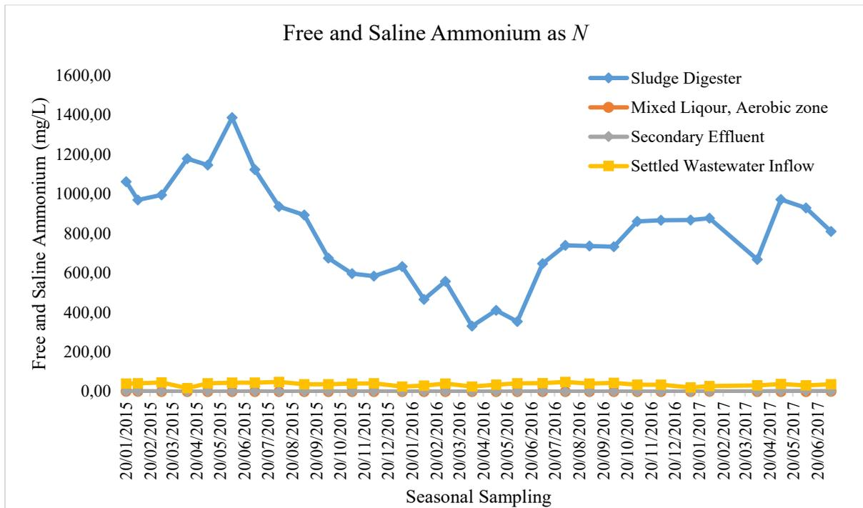
**Figure 4.26:** Seasonal variation of the free and saline ammonium as N for the mixed liquor in the WWTP
