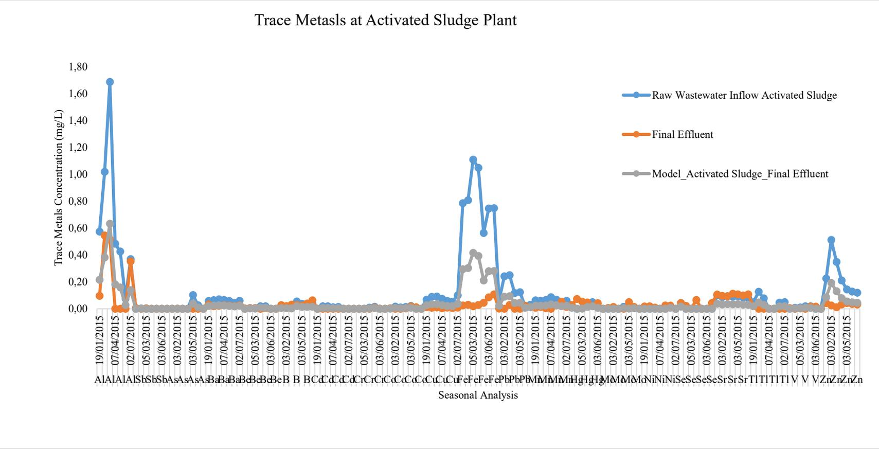
**Figure 5.5:** Daily variation of trace metals contents in the influence of the activated sludge wastewater treatment plants
