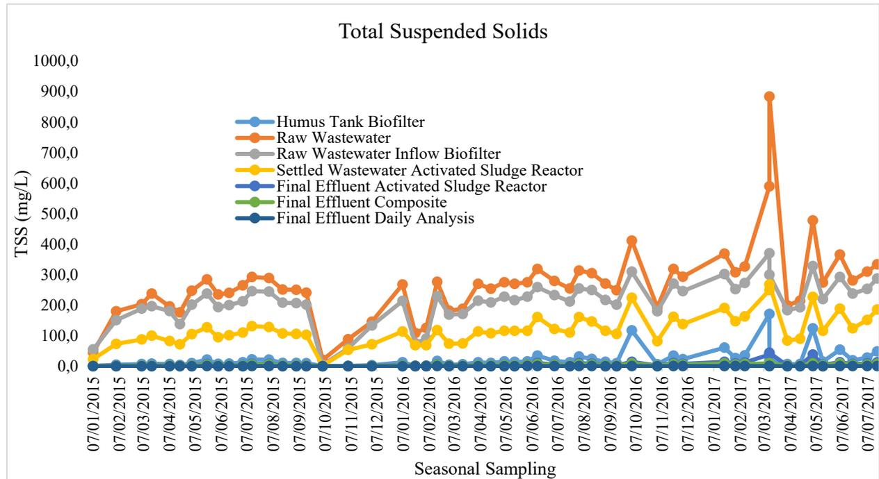
**Figure 4.18:** Seasonal variation of the total suspended solids in the wastewater treatment plant
