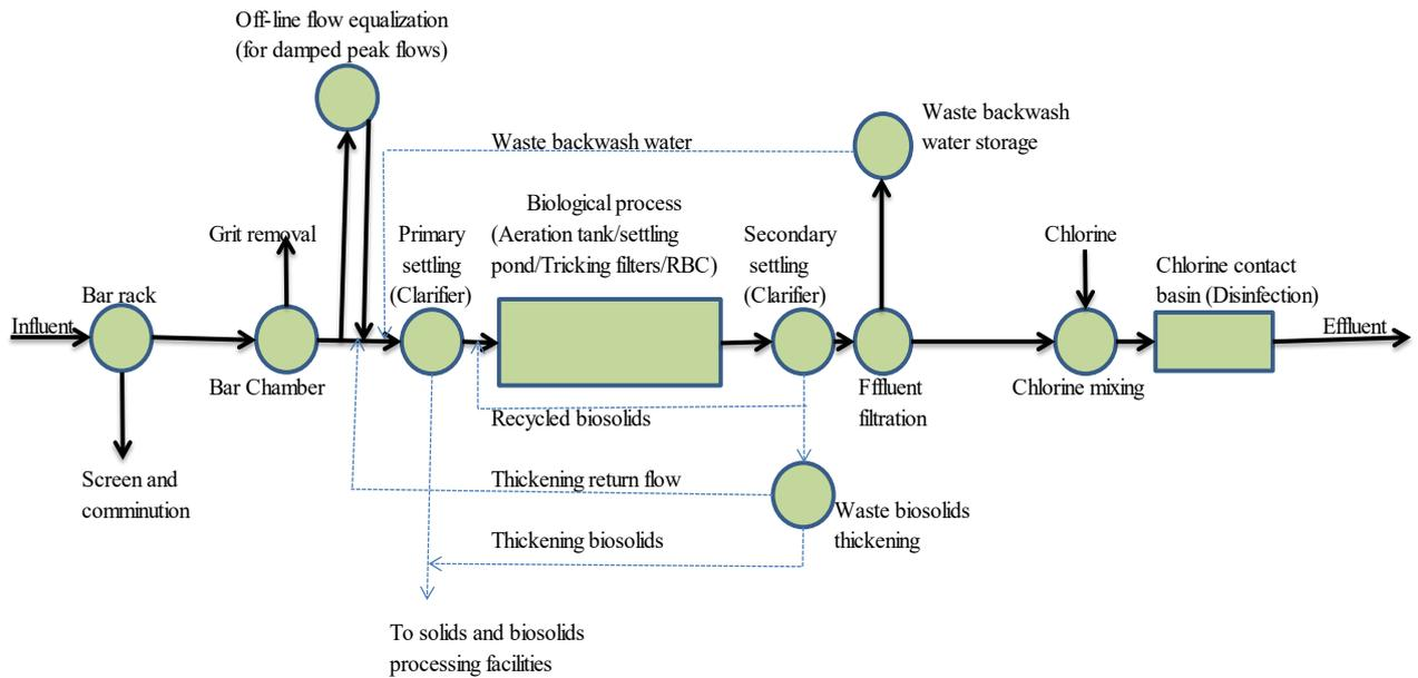
**Figure 2.6:** Flow diagram for unit operation and processes in physical, chemical and biological processes used in wastewater treatment (E. Metcalf).
