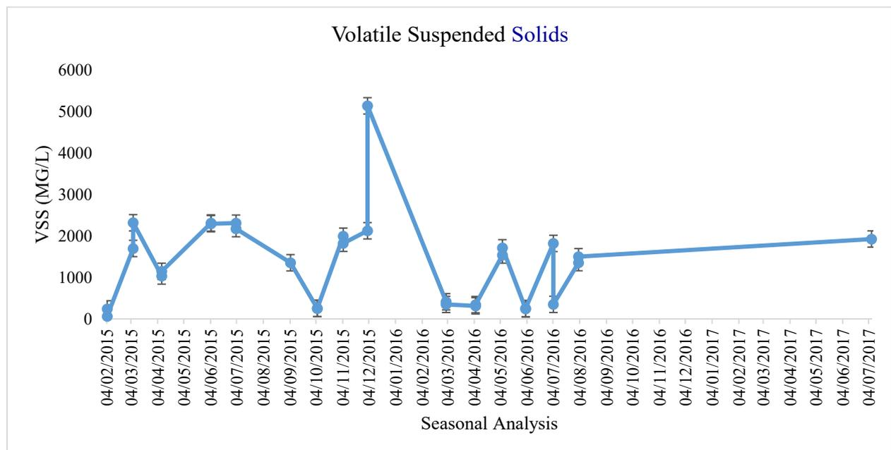
**Figure 4.19:** Seasonal variation of the volatile suspended solids-mixed mixed liquor of the *WWTP*.
