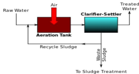
*Figure 2.5: General schematic diagram of an activated sludge process*
