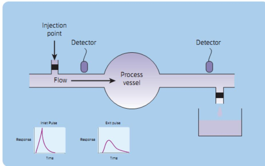
*Figure 2.8 Principle of tracer residence time distribution (RTD) (de Souza Jr & Lorenz; IAEA, 2011a).*
