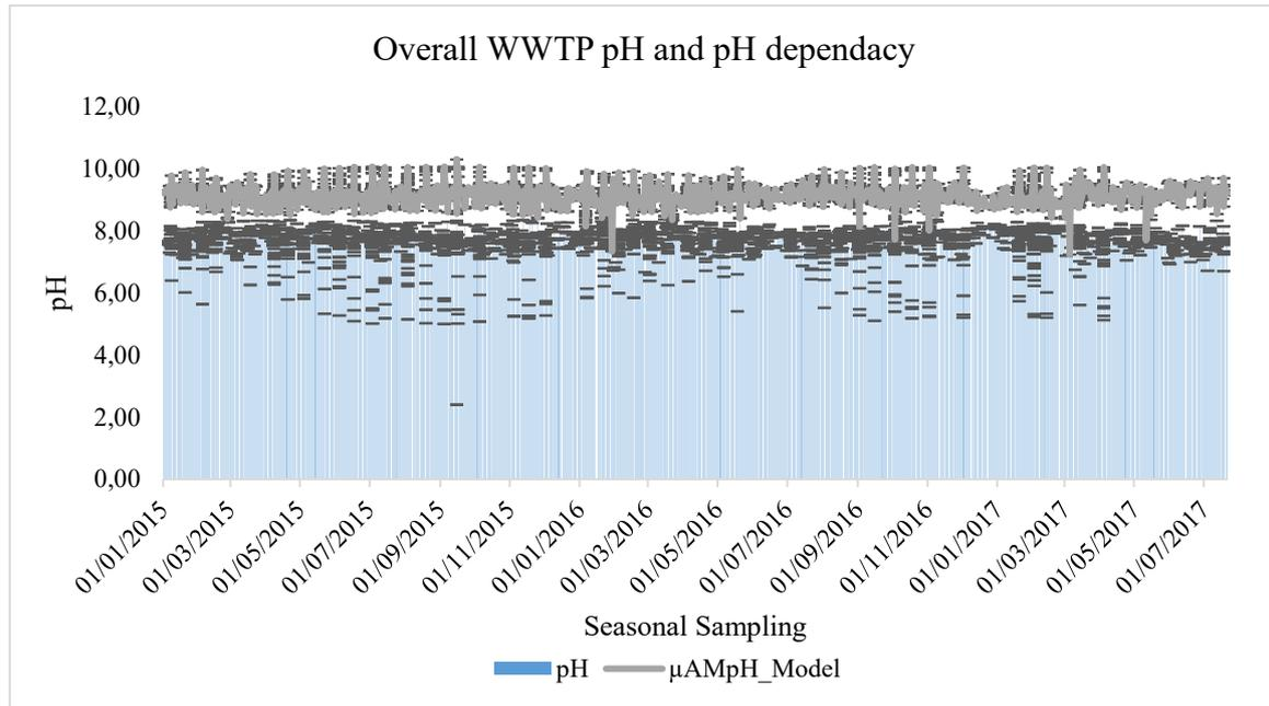
**Figure 4.7:** The seasonal variation of the  $pH$  and  $pH$  dependency in the wastewater treatment process
