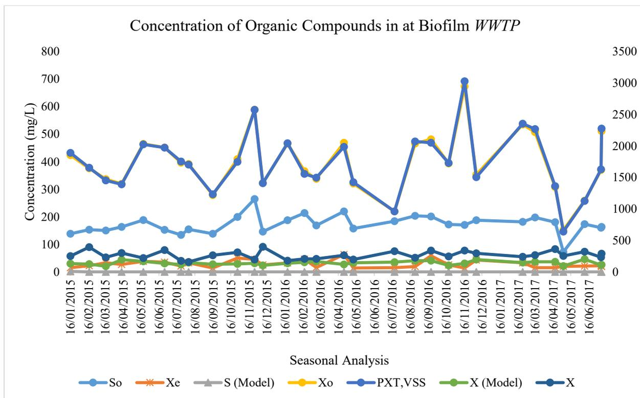
**Figure 4.15:** Modelling of organic compounds in the biofilm of the *WWTP*
