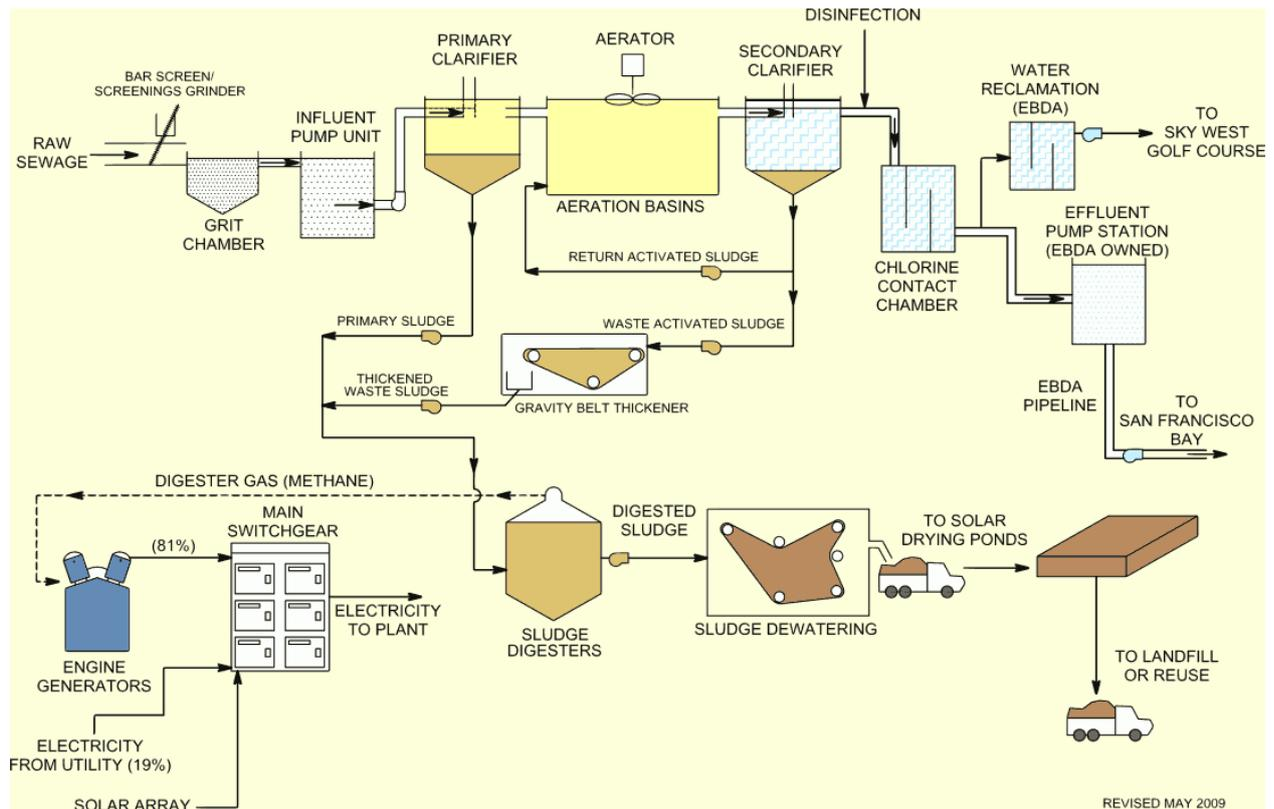
**Figure 2.4:** General wastewater treatment process units operation (E. Metcalf).
