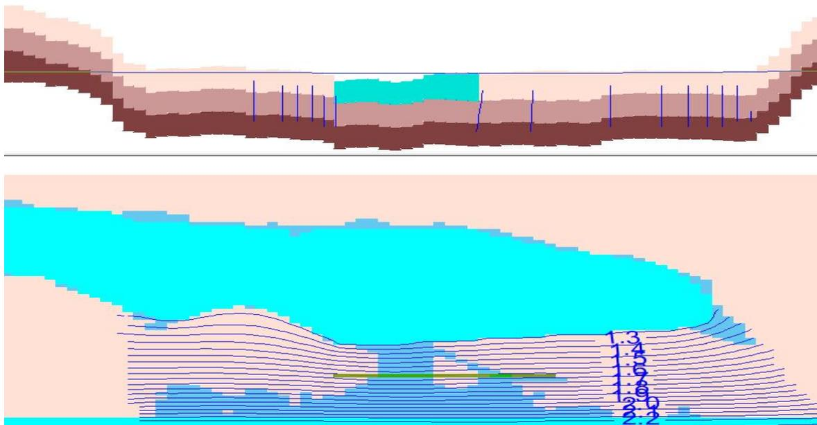
Figure 3-13: The model configuration for estimating the groundwater fluxes through the mouth with varying tidal action.
