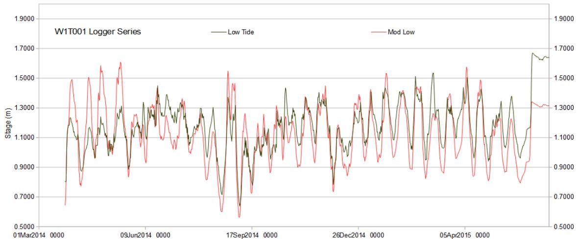
**Figure 3-11: W1T001 logger series showing the diurnal Minimum (Low tide) and the modified low tide estimated from a direct proportion of the High Tide (H-H/5)**
