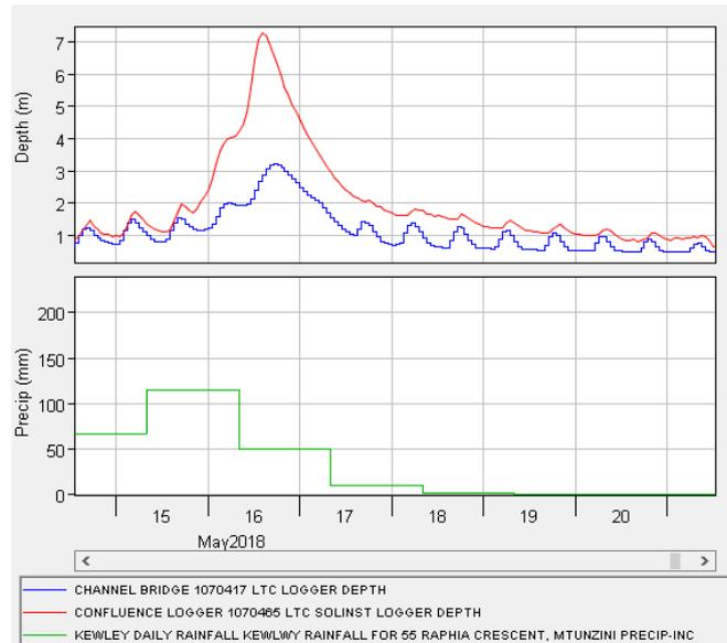
**Figure 3-2: The rainfall (lower graph) and the simultaneous measurements of the water level (upper graph) at the confluence of the two tributaries in the upper estuary (red line) and near the mouth (blue line) near the discharge point.**
