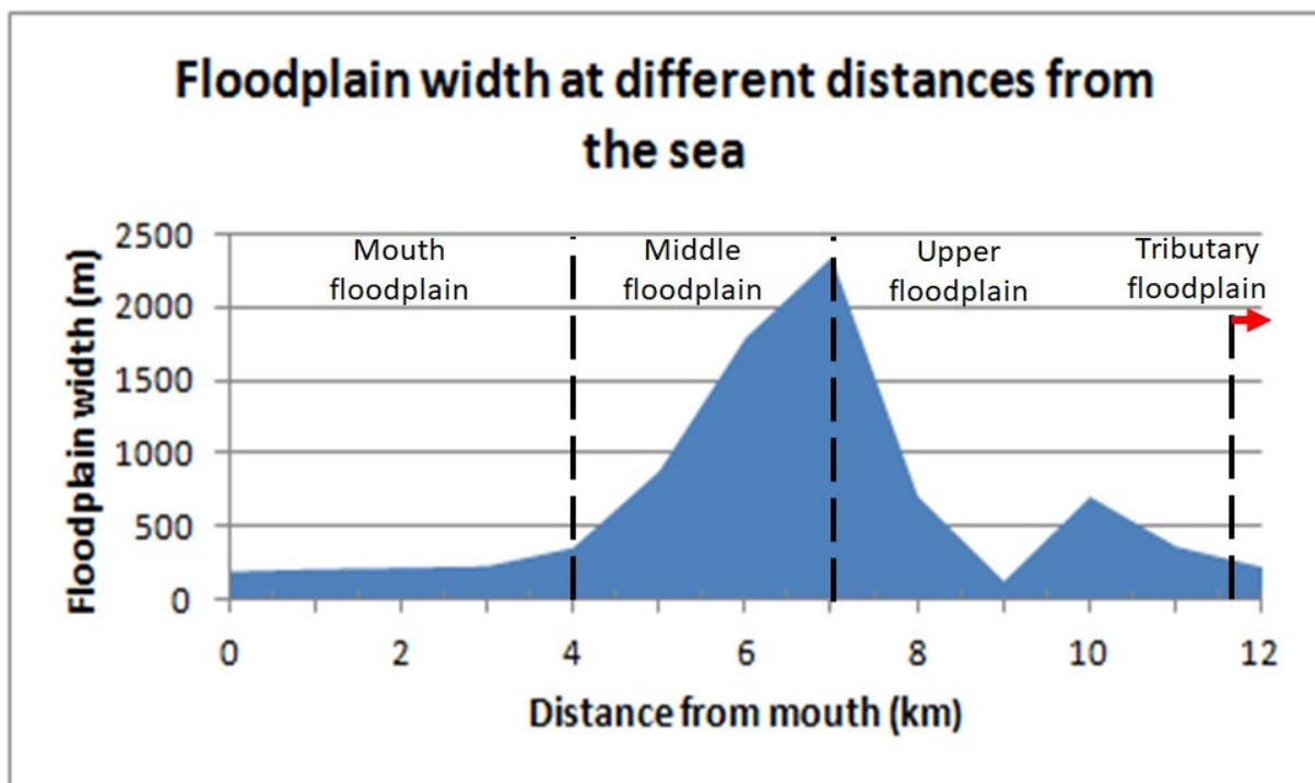
Figure 7-1: The floodplain width relative to distance from the mouth.
