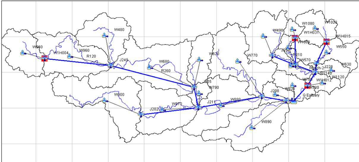
Figure 2-14: Sub-catchments network generated in HEC-GeoHMS
