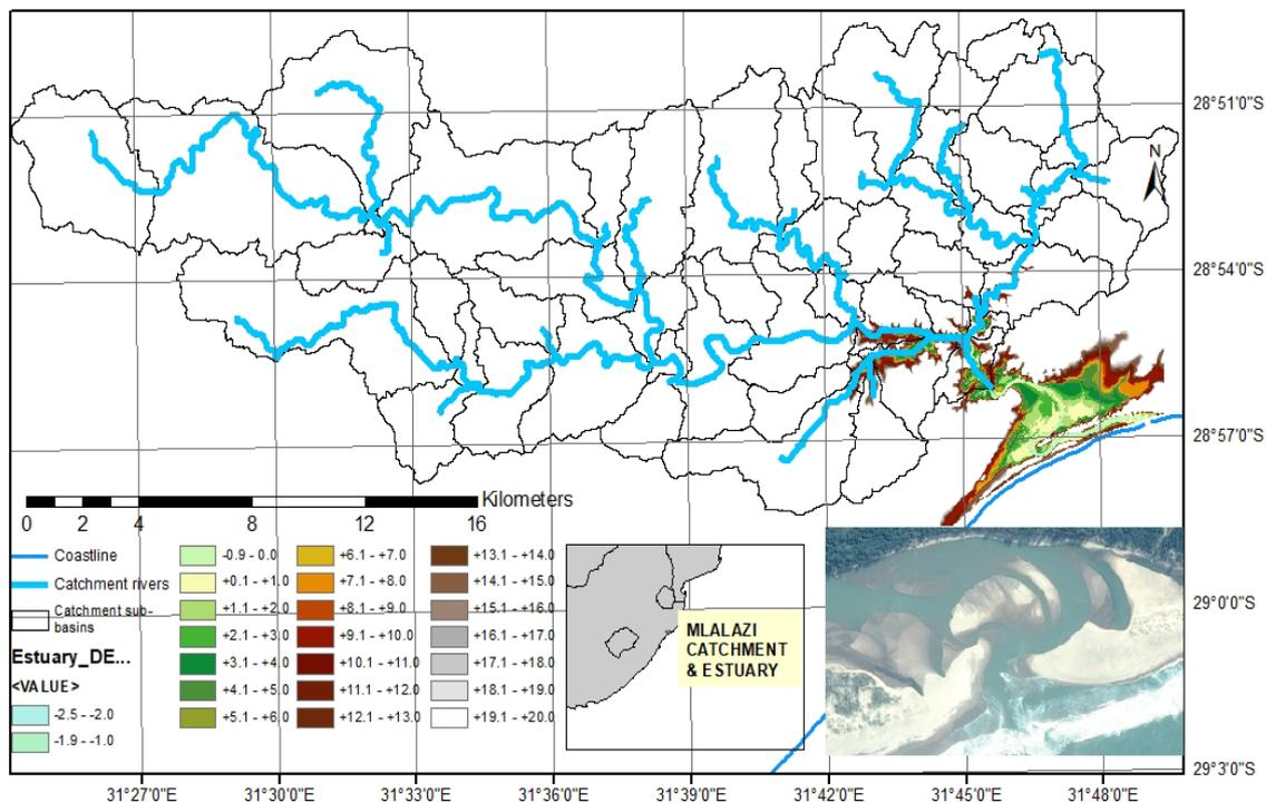
**Figure 2-1.** The location of the Mlalazi study site comprising the runoff catchment represented by the black polygons and river network that discharge directly into the estuary. The Digital Elevation Model (DEM) of the estuary and floodplain is shown by the coloured contours. Also included is a Google Earth image of the mouth illustrating the mobile sandy berm that has a controlling influence on the estuary hydrodynamics.
