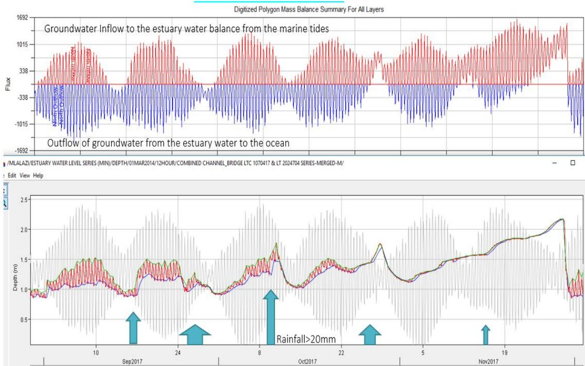
**Figure 3-14:** (A) The simulated groundwater fluxes out of the estuary (to the south) and the corresponding groundwater inflow during the marine high tides (blue). (B) The lower graph shows the estuary water level tides (red) and their high and low sequence in relation to the marine tides (grey series).
