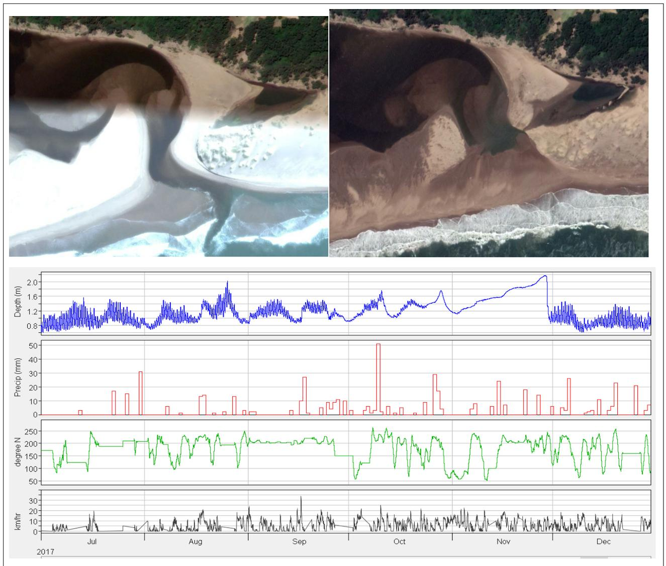
Figure 4-2: Conditions associated with the mouth closure during Nov 2017.
