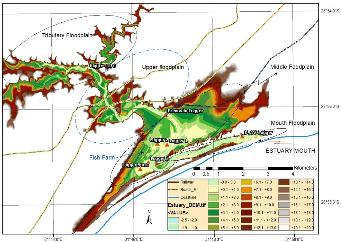
**Figure 2-10: The derived Digital Elevation Model (DEM) of the Mlalazi Floodplain with selected infrastructures. The Estuary floodplain has been divided into four regions where the hypsometric conditions are significantly different. The red triangles show the location of stage monitoring sites.**
