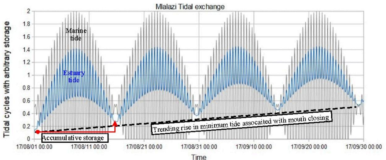
Figure 8-5: A model simulation of the marine tide (grey) and estuary tide (blue) assuming the indicated level of storage within the estuary between flood and ebb tides leading to the systematic reduction in the tidal range associated with the rising mouth elevation without fluvial interruptions.
