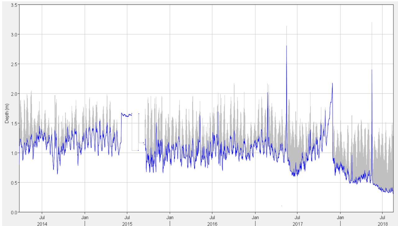
**Figure 3-16:** The water level measurements for the Mlalazi Estuary. The blue line shows the low tide. The grey lines show the hourly tidal range. The early period represents “drought” conditions when there were few large fluvial events. From 2017 there was a significant increase in rainfall and the occurrence of extreme storm events.
