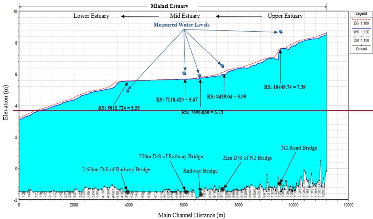
**Figure 2-22: The simulated water table profile along the estuary channel downstream of the confluence of the Mlalazi and Ntuze tributaries at the peak of the 1987 storm events shown by the blue shading..**
