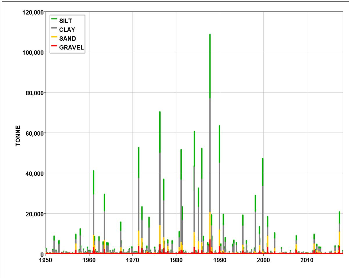
Figure 2-19: Simulated sediment yield grainsize distribution (tonne/day)
