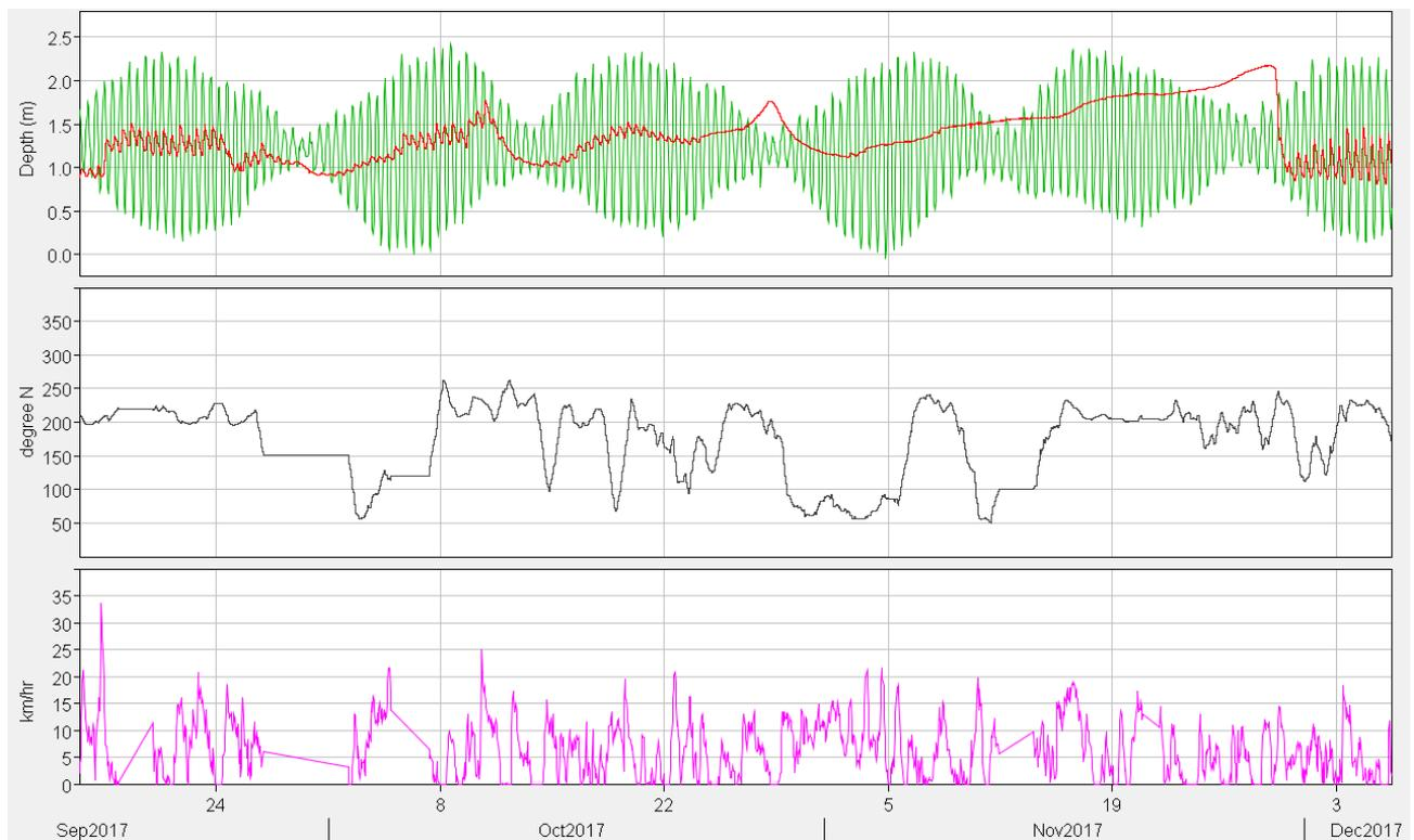
**Figure 3-17: The marine tides and estuary water level (Upper graph), the smoothed wind direction (middle graph) and the hourly wind speeds during the period leading up to the mouth closure in Nov 2017.**
