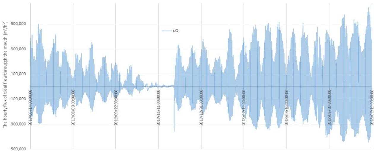
Figure 3-12: The calculated hourly flux ( $\text{m}^3/\text{hr}$ ) through the mouth channel from May 2017.
