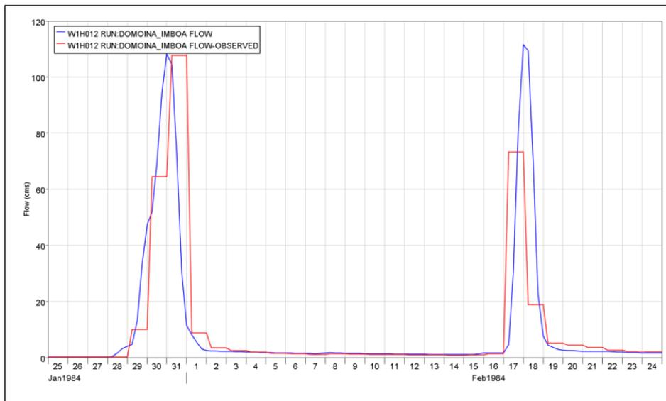
Figure 2-15: Observed (red) and simulated (blue) hydrographs for two storm events
