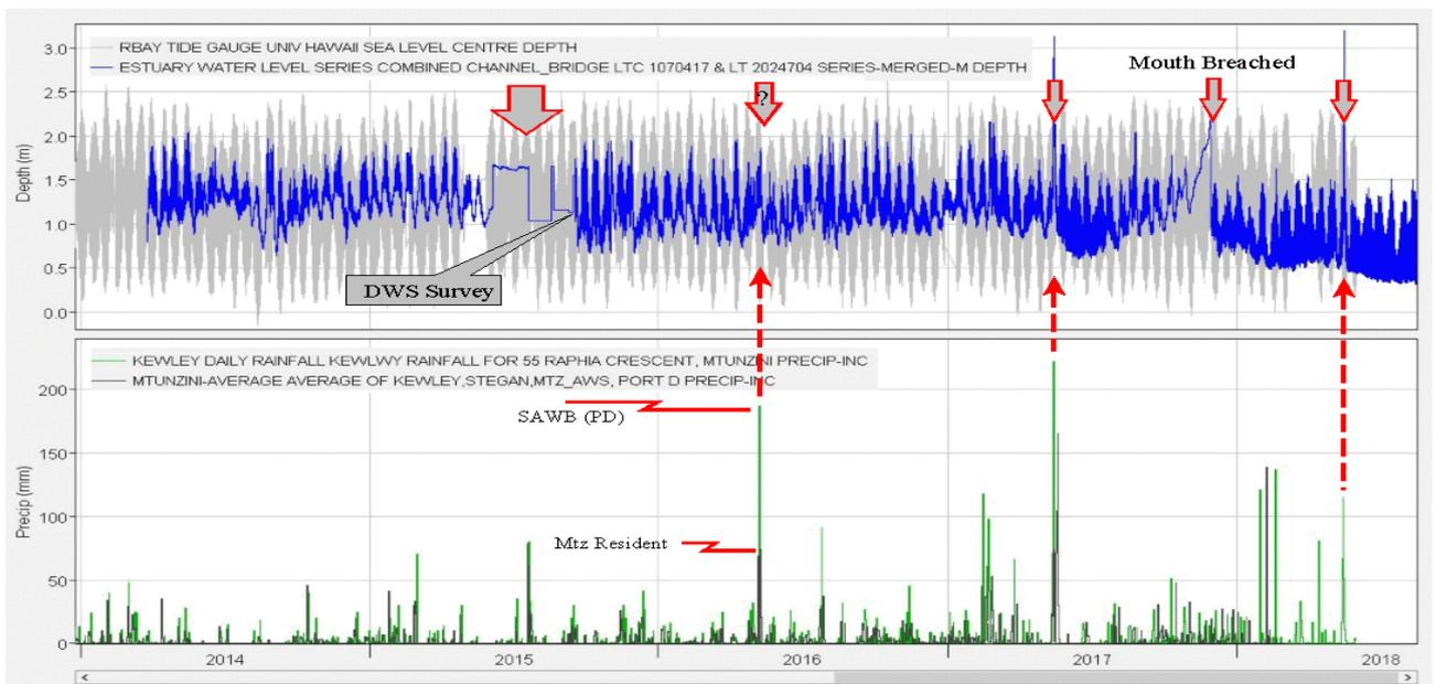
**Figure 2-20: The combined logger water level series for all the available logger downstream of the Railway Bridge. Also shown in the lower plot are the rainfall series the lower sections of the catchment.**
