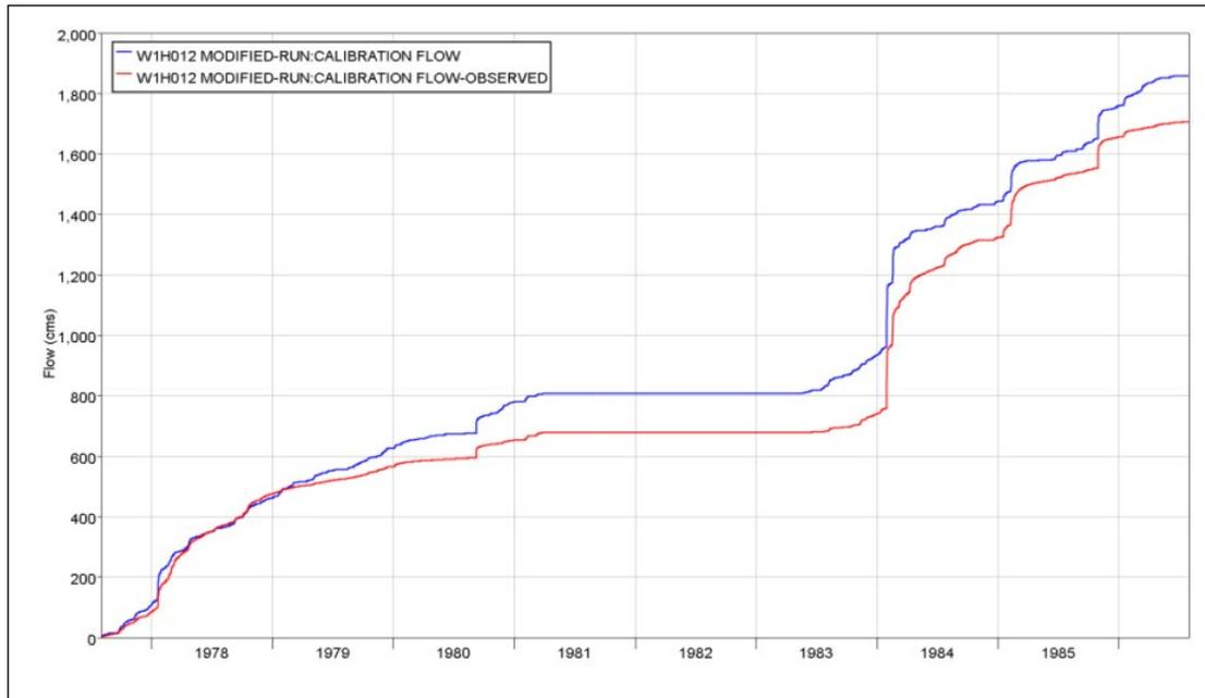
Figure 2-16: Calibration period cumulative observed (red) and simulated (blue) flows
