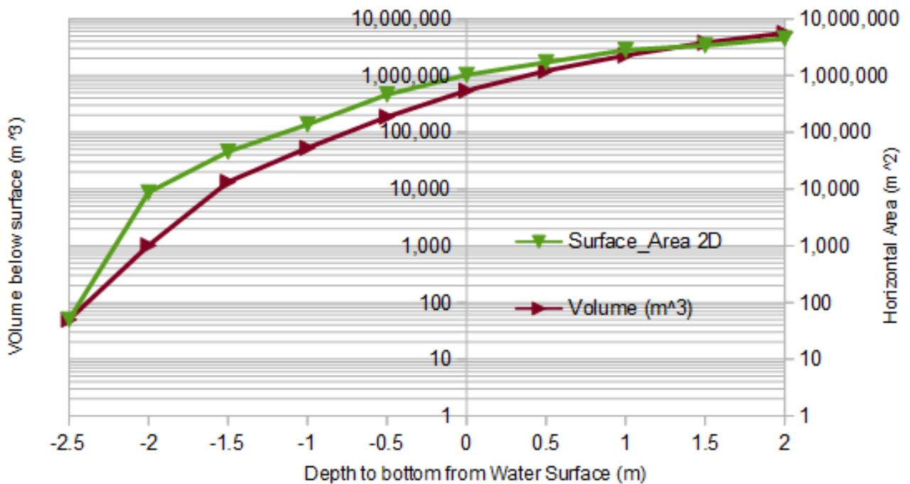
Figure 2-12: The hypsometric curves for surface area and volume for the channel below the 2 m contour.
