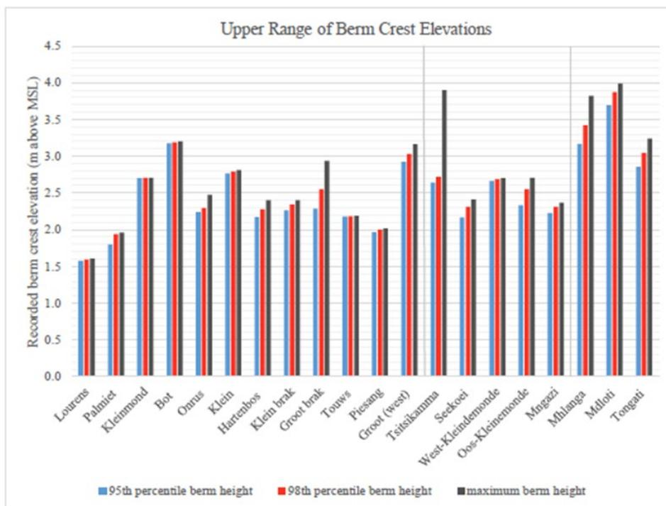
**Figure 7-3: The upper ranges of recorded berm crest elevations of selected South African TOCEs (from: Booyen, 2017)**
