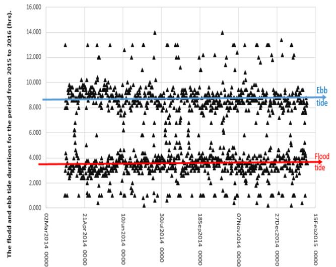
Figure 3-8: The duration of the flood and ebb tide at the mouth taken from the W1T001 logger series.
