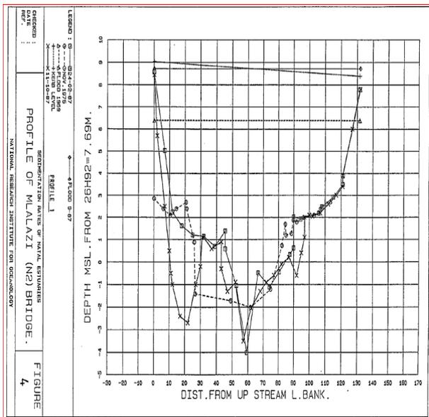
Figure 2-9: Water level and cross-sectional profile at the old N2 road bridge survey during several major flood events by Badenhorst *et al.* (1989).
