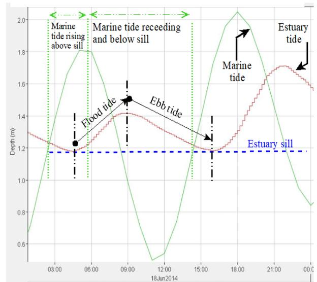
**Figure 3-7:** The marine and estuary tidal cycle showing the flood and ebb tide features in relation to the marine tide.
