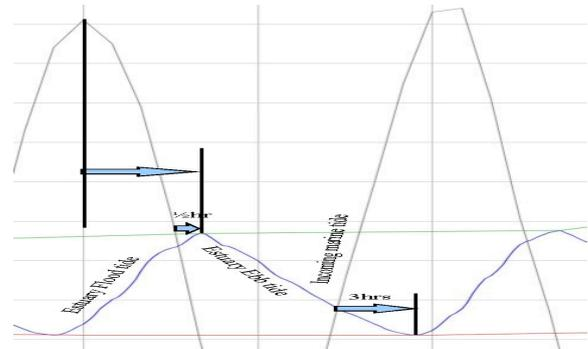
**Figure 3-6:** An example of the simultaneous marine and estuary tidal variation across the mouth. The lower arrows show the lag for the corresponding water level elevation in the marine and estuary tide across the mouth. The estuary tide would be expected to turn when the elevations were the same.
