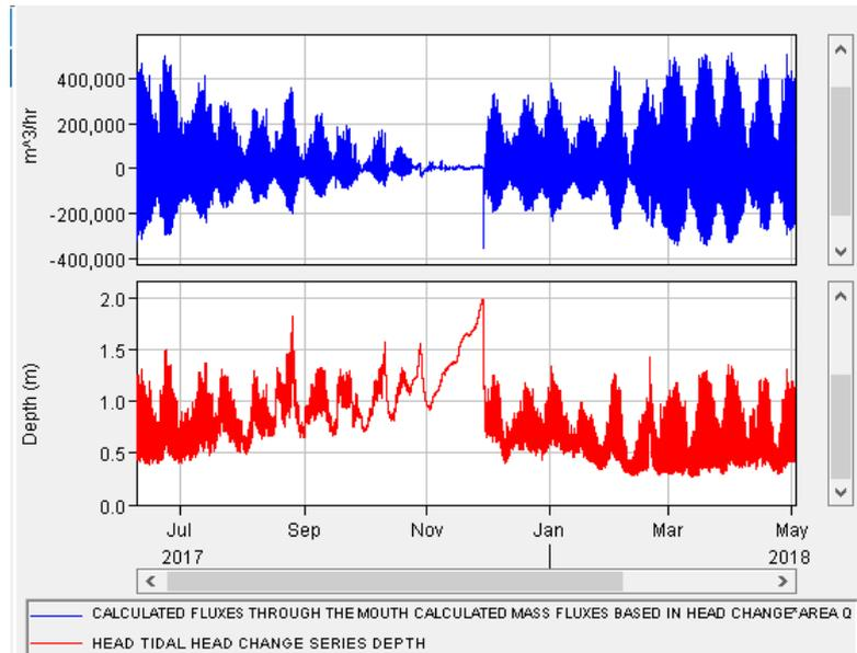
**Figure 2-13:** The measured tidal range (red graph) before and after the mouth closure in December 2017 used to calculate the flow rate ( $\text{m}^3/\text{hr}$ ) through the mouth (blue graph).
