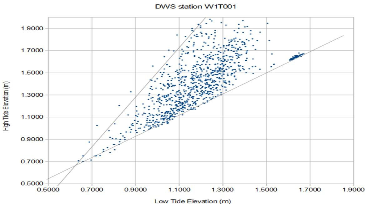
Figure 3-10: Scatter plot of the high and low diurnal tidal elevation for W1T001. The grouping of points at the low tide elevation of 1.6 m correspond to the period the mouth was closed.
