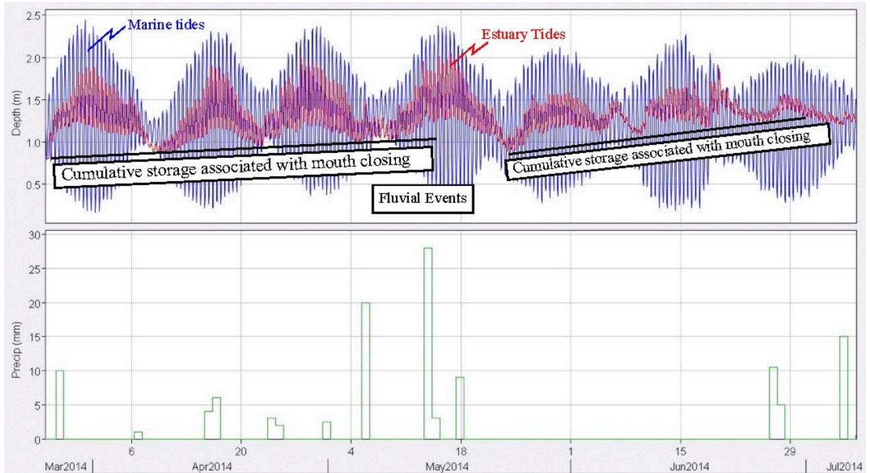
**Figure 8-6: Observations of the marine (blue) and Estuary (red) tidal interaction during 2014 showing the trends in estuary storage resulting in rising levels of the minimum low tide that is assumed to be associated with the mouth elevation. The rising trend in storage (mouth elevation) is interrupted by fluvial events shown by the rainfall record in the lower graph.**
