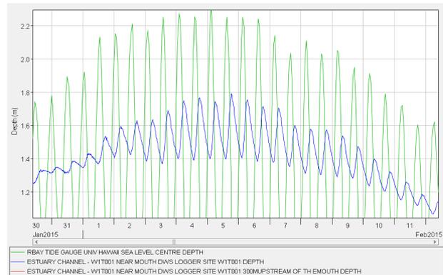
**Figure 3-4: Water level measurements of the marine and estuary tides over a complete lunar cycle showing the lag and attenuation of the marine wave through the mouth.**
