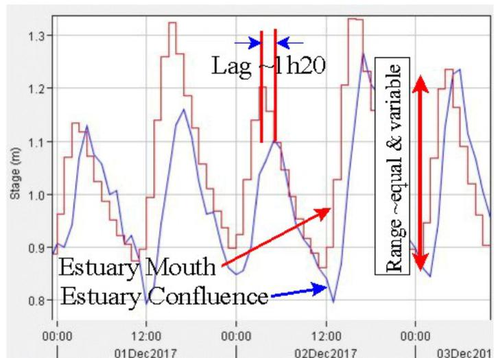
**Figure 3-3: The water level measurement near the mouth (red line) and at the confluence of the tributaries (Blue line) illustrating the magnitude of the lag and attenuation during the wave propagation from the mouth to the top of the estuary.**
