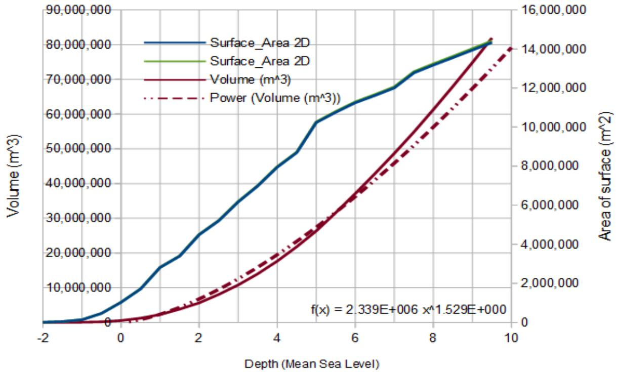
Figure 2-11: The Hypsometric curve for the entire floodplain and estuary channel
