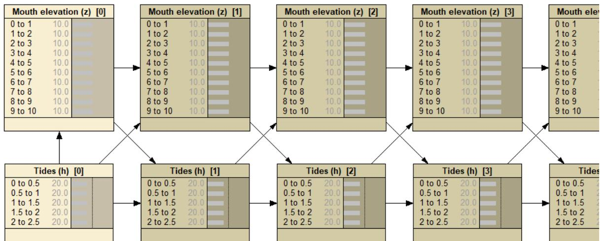
Figure 8-2: A simplistic model of the changing mouth conditions in incremental time steps in Netica.
