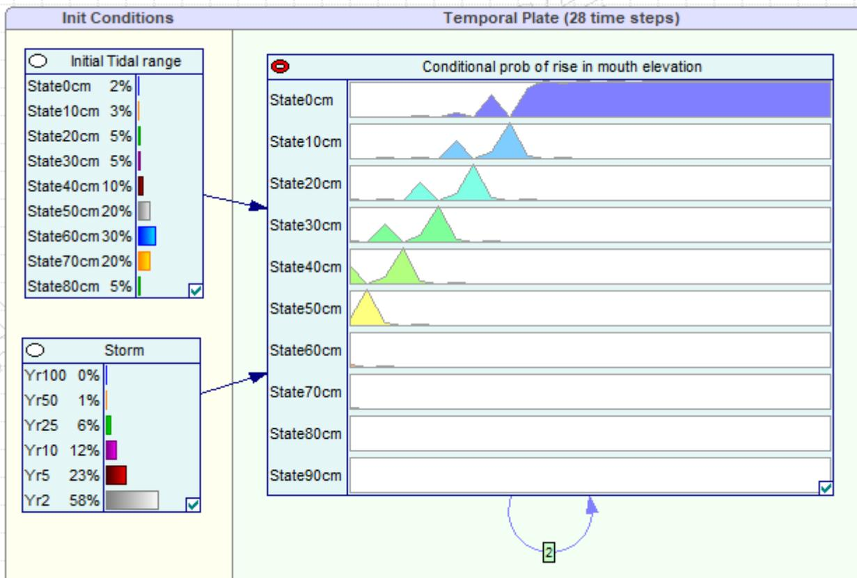
Figure 8-3: The model configuration in GeNIe for the state of the mouth during the 28 step sequence starting with initial conditions of tidal range and storm event.
