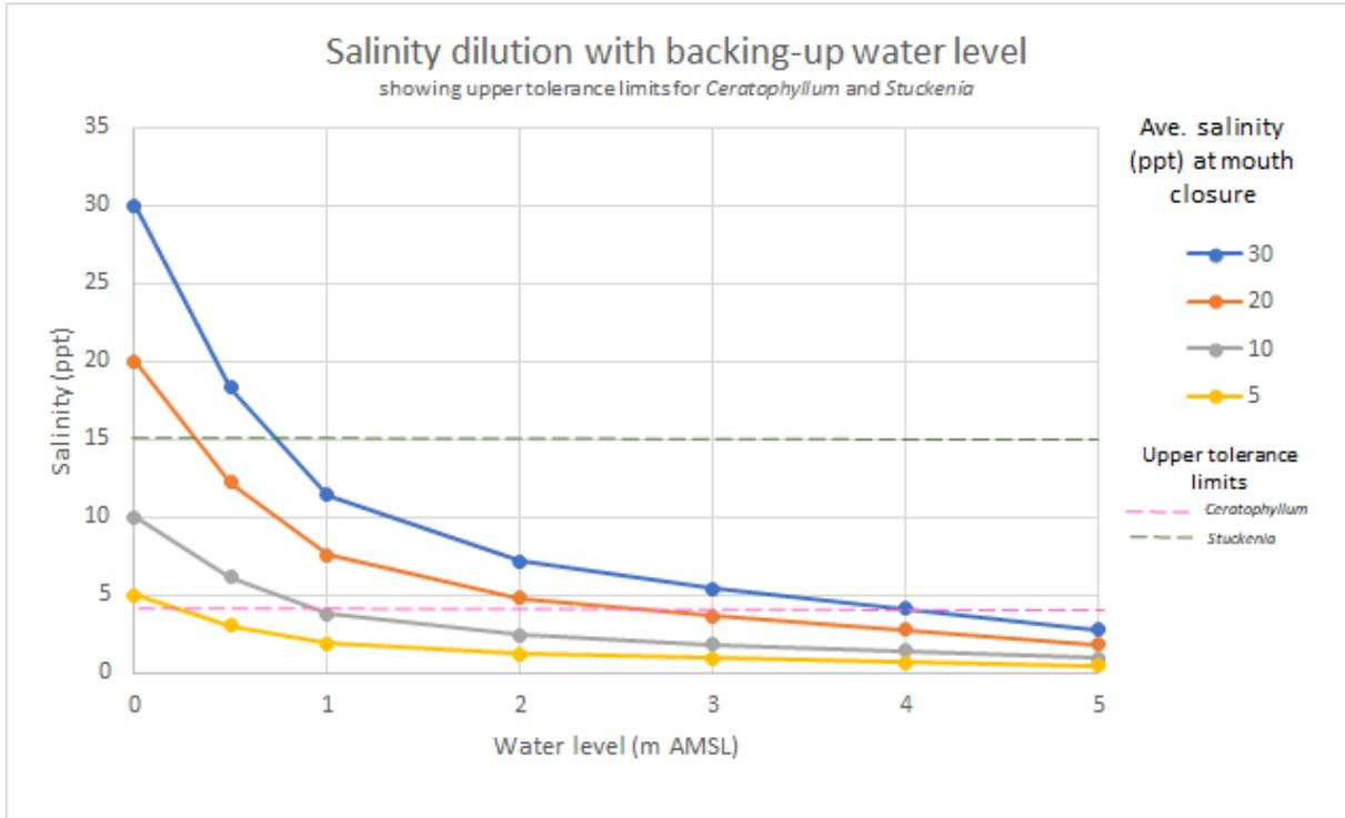
Figure 6-5: The graphs calculated using salinity dilution at different estuary volumes – using different mean salinity values at the time of mouth closure. The assumption is made that water level is at MSL on closure. Also shown on the graph are upper tolerance limits for *Ceratophyllum* and *Stuckenia*. This graph assumes complete mixing of the water, a situation that is unlikely to occur.
