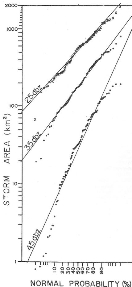
**Figure 2-4: Probability Density Function for storm Areas defined by three radar reflectivity levels (Kelbe, 1984)**
