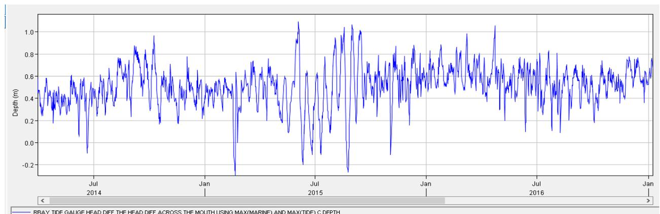
**Figure 3-5: The level of attenuation of the marine tide entering the estuary for the observation period from 2014-2016. Some of the extreme values were due to fluvial events.**
