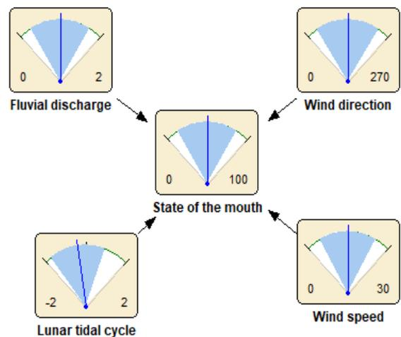
**Figure 8-1: Simplistic graphical representation (using Netica) of joint probabilistic model of the main conceptualised factors controlling the mouth state. Arrows indicate the joint probabilities.**
