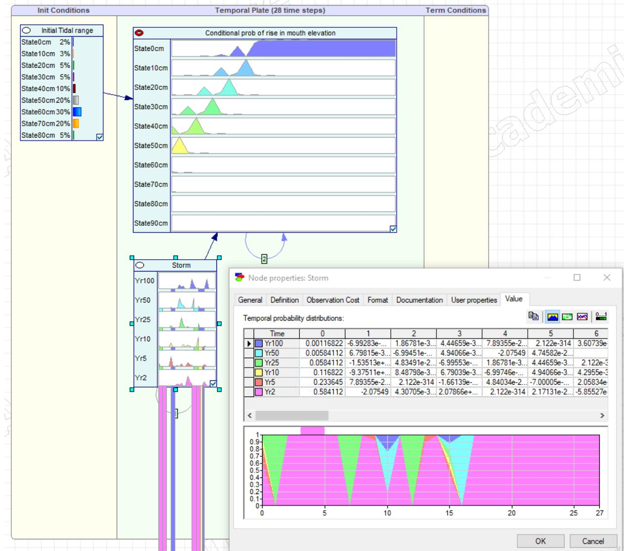
Figure 8-4: The DBN in GeNIe showing the attempt to include a stochastic storm sequence linked to the mouth state. Also shown is the conditional probability table for the time steps in the storm node.
