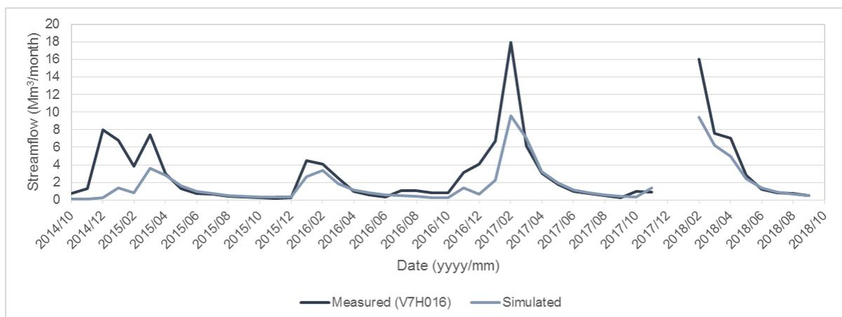
**Figure C-19: Gauge V7H016 – comparison of measured and simulated monthly streamflow volumes**
