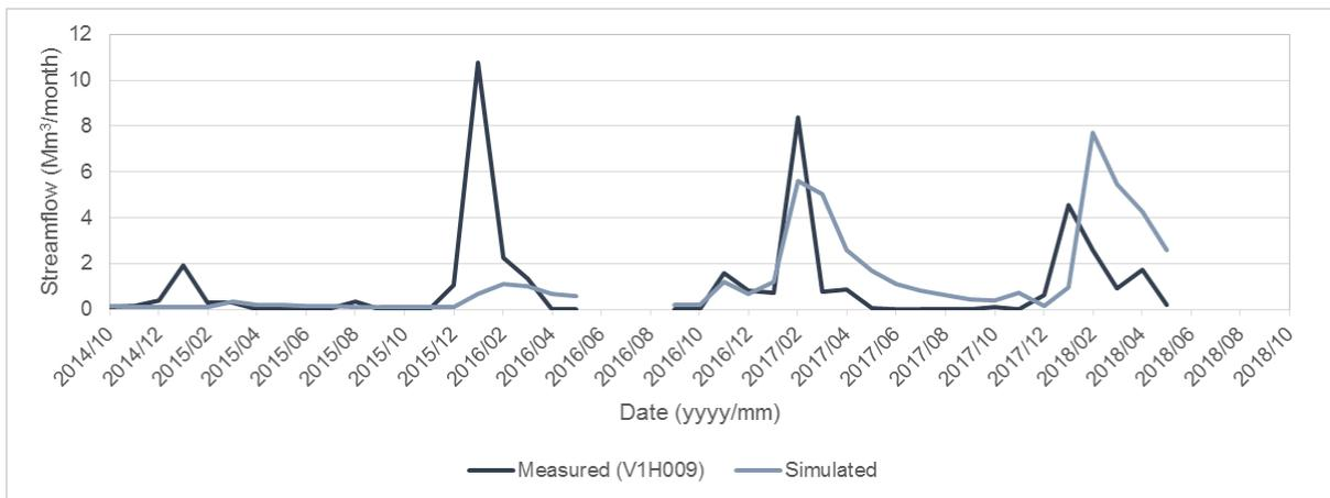
**Figure C-11: Gauge V1H009 – comparison of measured and simulated monthly streamflow volumes**
