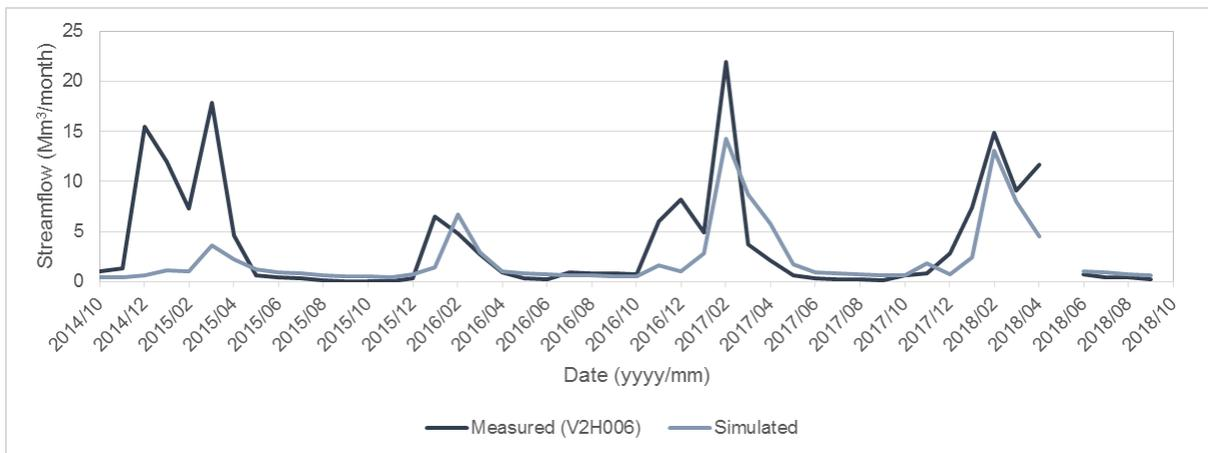
**Figure C-14: Gauge V2H006 – comparison of measured and simulated monthly streamflow volumes**
