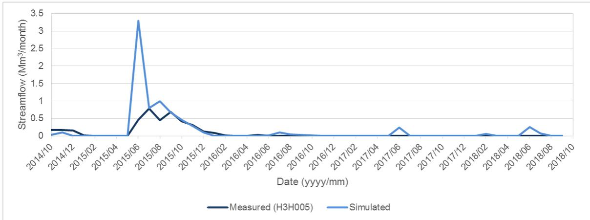
**Figure C-26: Gauge H3H005 – comparison of measured and simulated monthly streamflow volumes**
