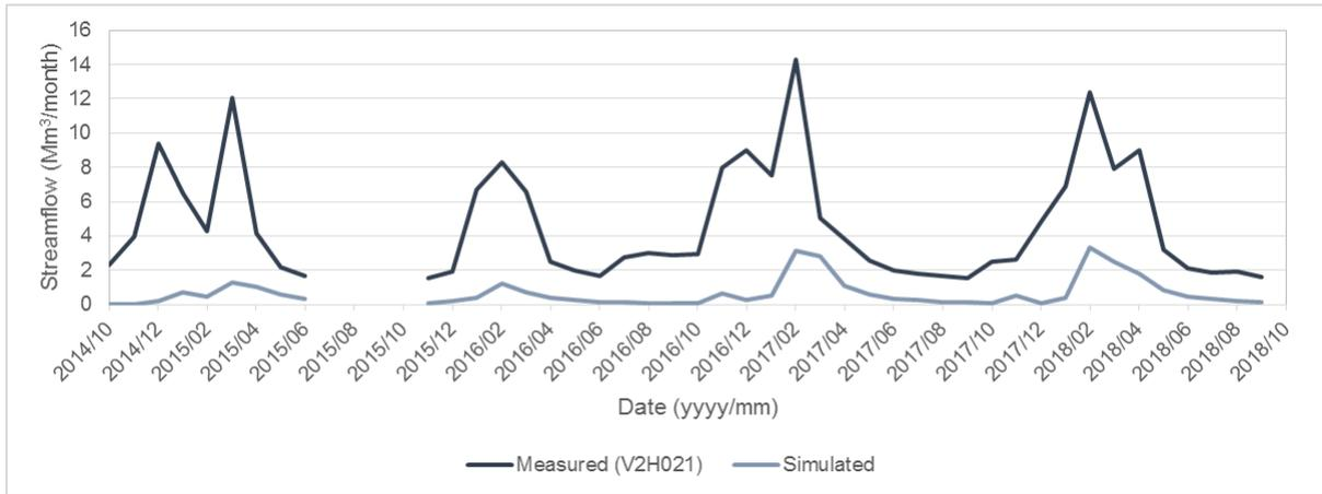
**Figure C-13: Gauge V2H021 – comparison of measured and simulated monthly streamflow volumes**
