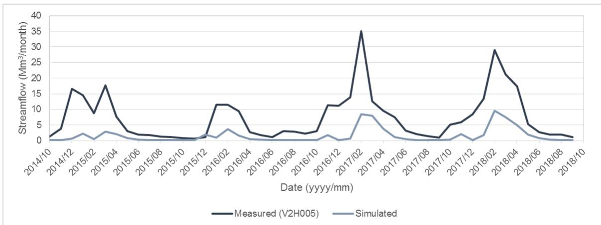
**Figure C-12: Gauge V2H005 – comparison of measured and simulated monthly streamflow volumes**
