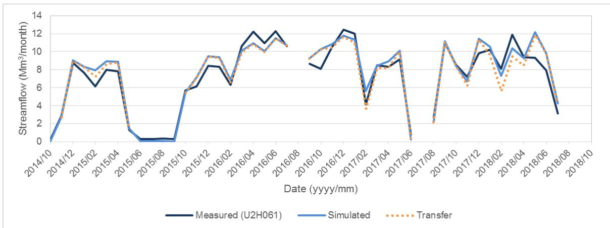
**Figure C-2: Gauge U2H061 – comparison of measured and simulated monthly streamflow volumes**
