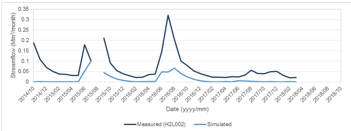
**Figure C-22: Gauge H2L002 – comparison of measured and simulated monthly streamflow volumes**
