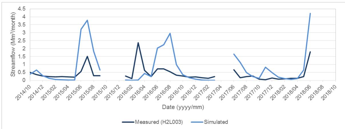
**Figure C-24: Gauge H2L003 – comparison of measured and simulated monthly streamflow volumes**
