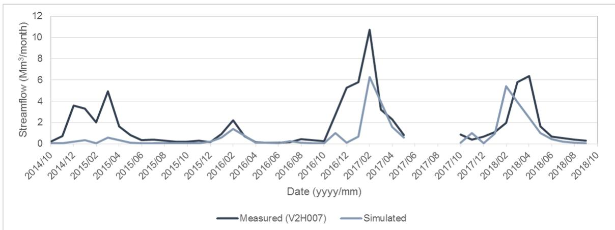
**Figure C-15: Gauge V2H007 – comparison of measured and simulated monthly streamflow volumes**
