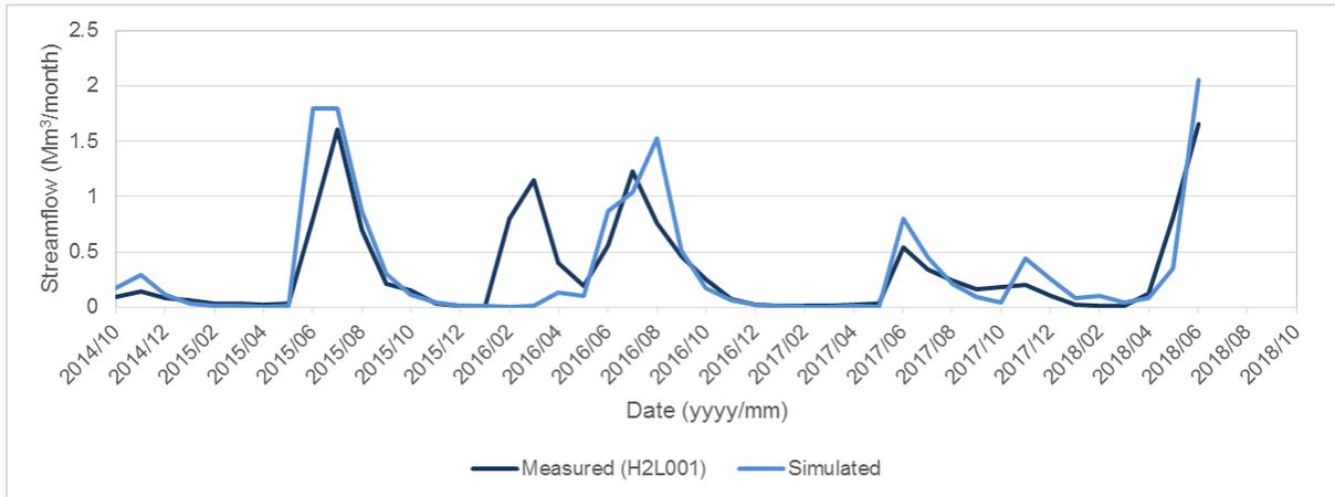
**Figure C-23: Gauge H2L001 – comparison of measured and simulated monthly streamflow volumes**
