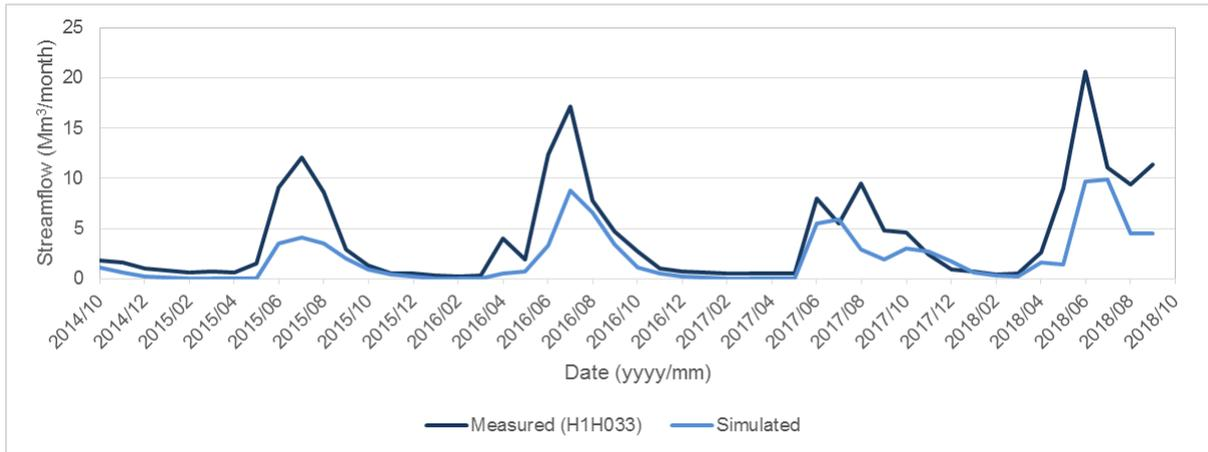
**Figure C-20: Gauge H1H033 – comparison of measured and simulated monthly streamflow volumes**
