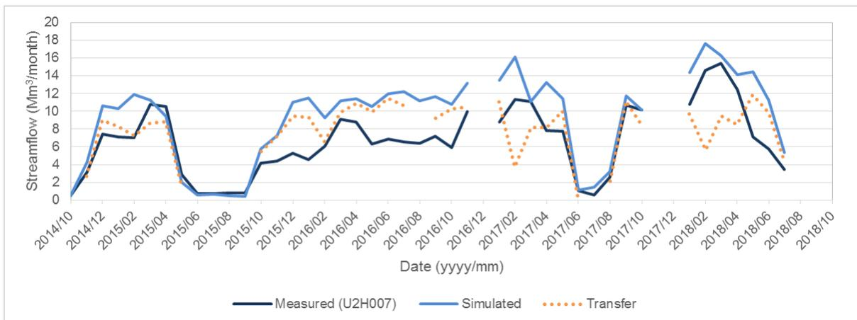
**Figure C-3: Gauge U2H007 – comparison of measured and simulated monthly streamflow volumes**
