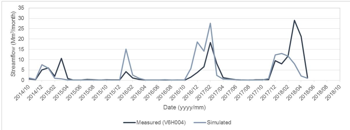
**Figure C-16: Gauge V6H004 – comparison of measured and simulated monthly streamflow volumes**
