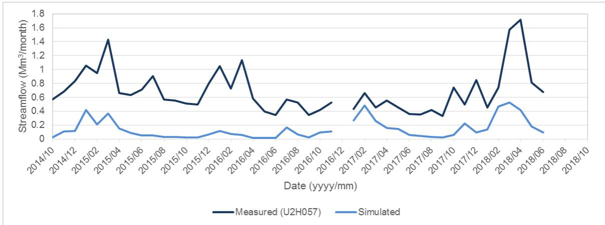
**Figure C-7: Gauge U2H057 – comparison of measured and simulated monthly streamflow volumes**
