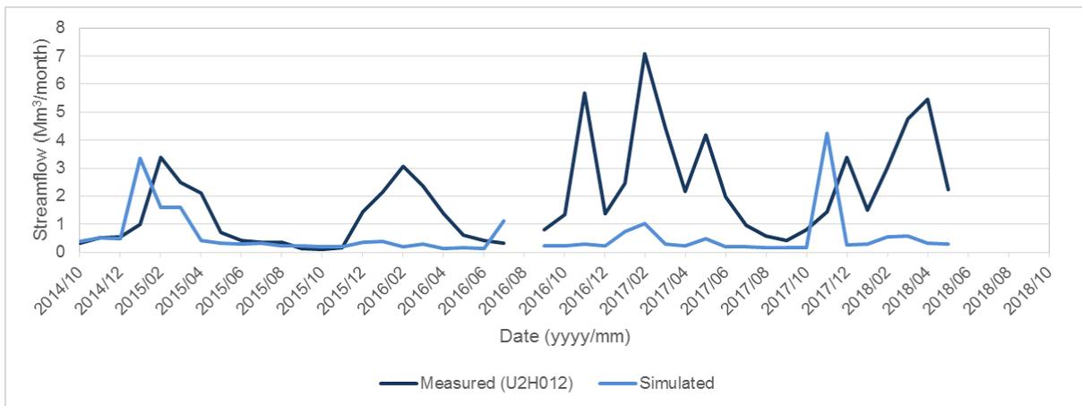
**Figure C-5: Gauge U2H012 – comparison of measured and simulated monthly streamflow volumes**
