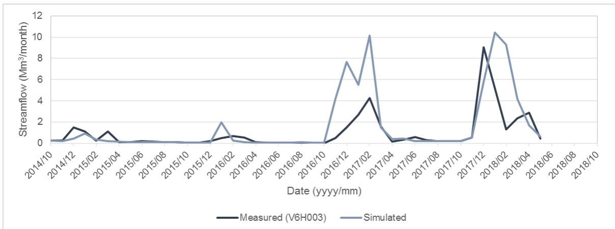
**Figure C-17: Gauge V6H003 – comparison of measured and simulated monthly streamflow volumes**
