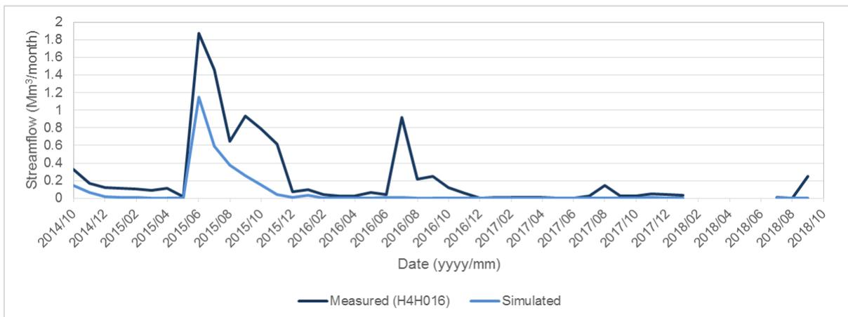
**Figure C-28: Gauge H4H016 – comparison of measured and simulated monthly streamflow volumes**
