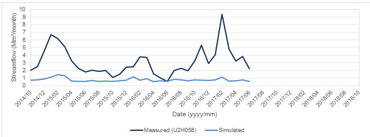
**Figure C-8: Gauge U2H058 – comparison of measured and simulated monthly streamflow volumes**
