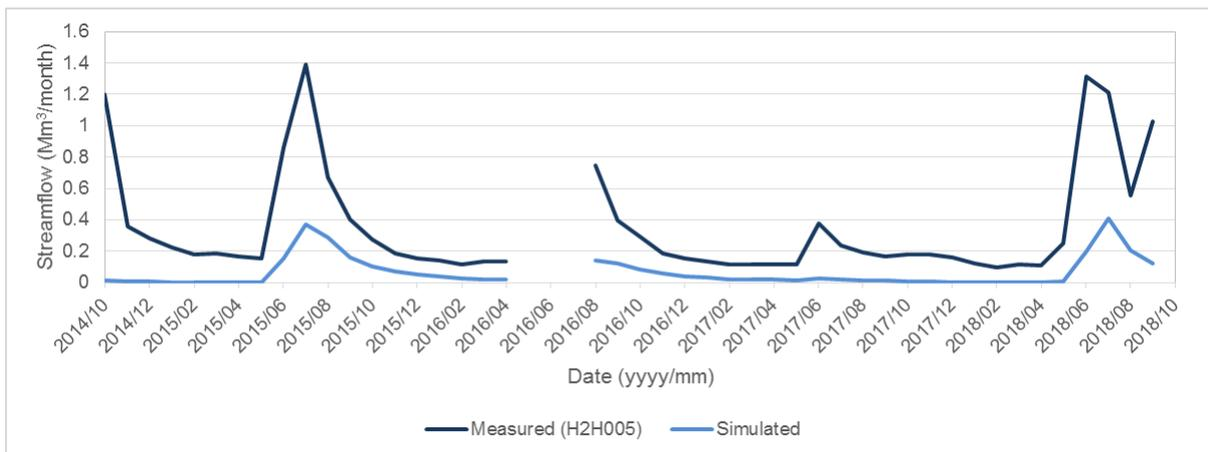
**Figure C-25: Gauge H2H005 – comparison of measured and simulated monthly streamflow volumes**
