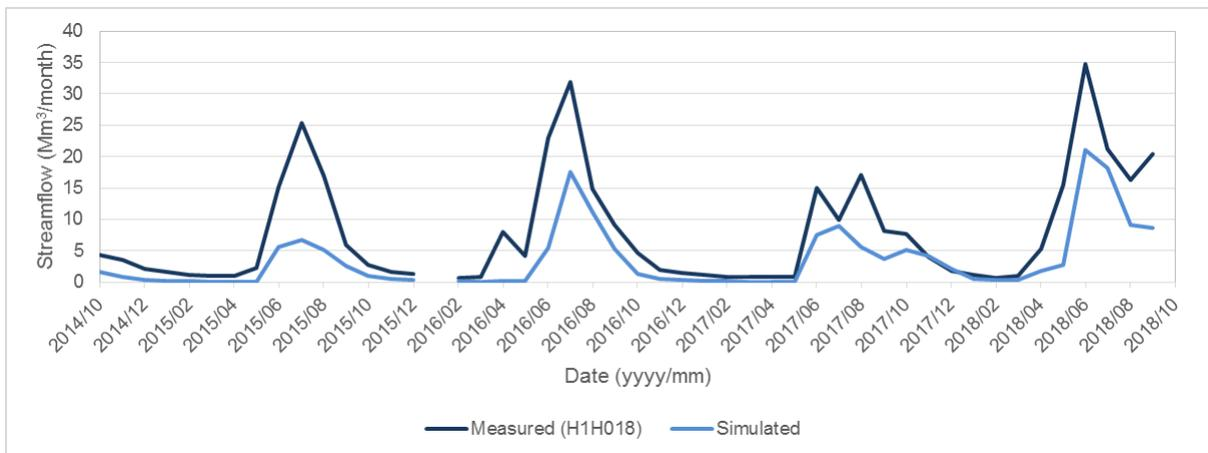
**Figure C-21: Gauge H1H018 – comparison of measured and simulated monthly streamflow volumes**
