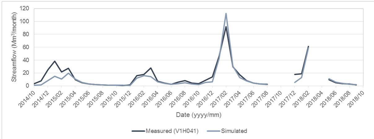
**Figure C-10: Gauge V1H041 – comparison of measured and simulated monthly streamflow volumes**
