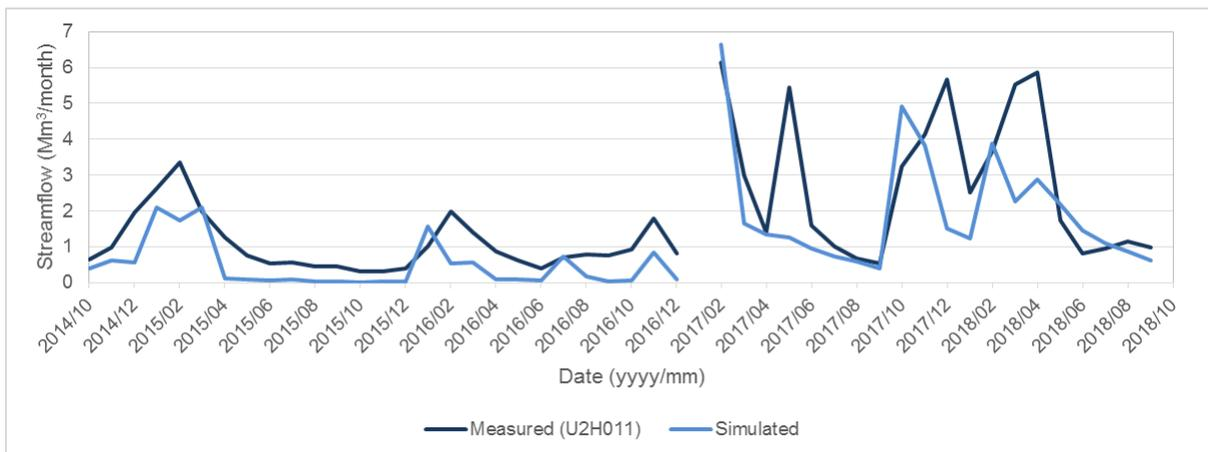
**Figure C-6: Gauge U2H011 – comparison of measured and simulated monthly streamflow volumes**
