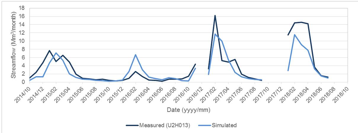
**Figure C-1: Gauge U2H013 – comparison of measured and simulated monthly streamflow volumes**
