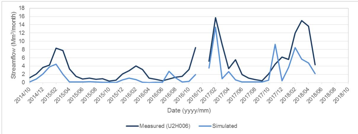
**Figure C-4: Gauge U2H006 – comparison of measured and simulated monthly streamflow volumes**
