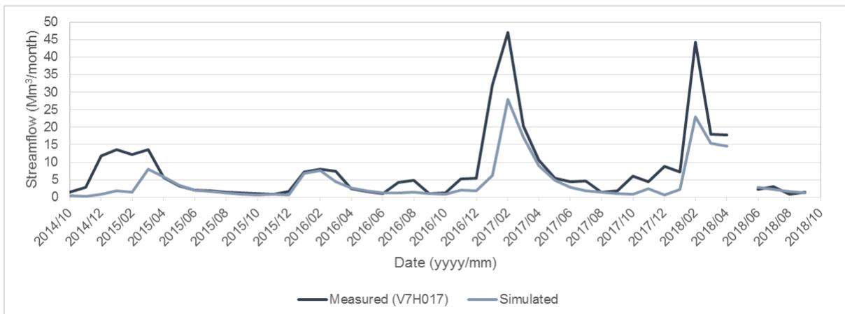
**Figure C-18: Gauge V7H017 – comparison of measured and simulated monthly streamflow volumes**
