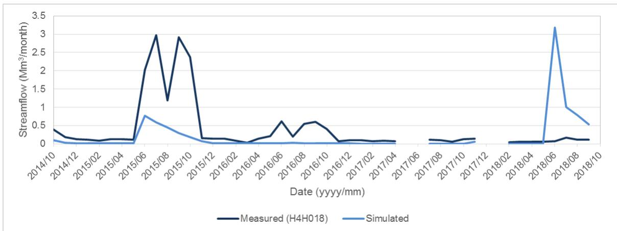
**Figure C-27: Gauge H4H018 – comparison of measured and simulated monthly streamflow volumes**
