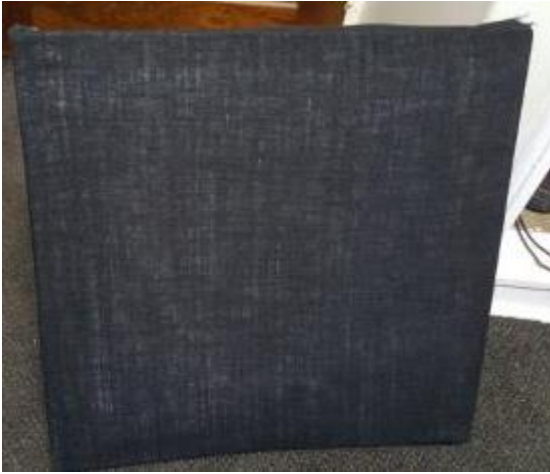
Figure 27: Wick cloth attached to polystyrene base
