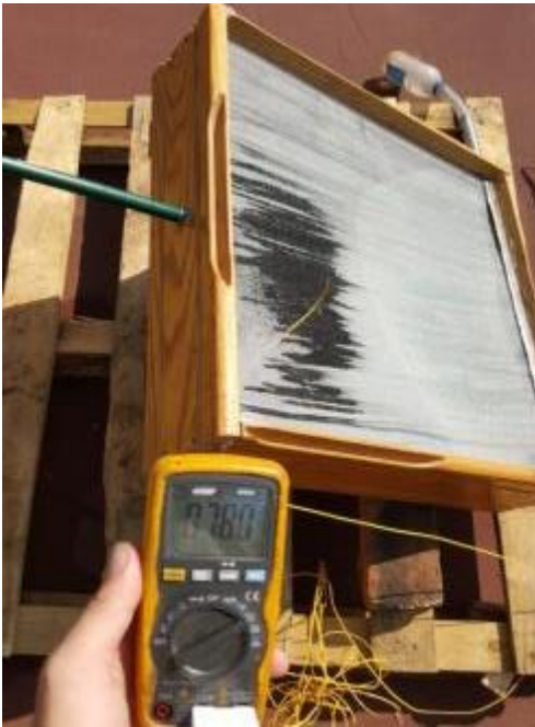
Figure 58: Maximum temperature obtained in the box using a single Perspex sheet
