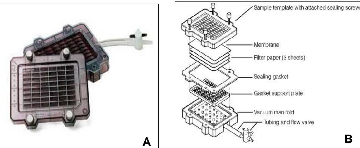
**Figure 4** A) Image of Bio-Dot<sup>®</sup> SF Microfiltration apparatus and B) components and assembly guide for the apparatus. (Images adopted from Bio-Rad instruction manual)
