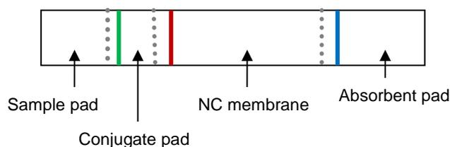
**Figure 5** Schematic diagram of LFIA strip assembly (top view); Overlap
