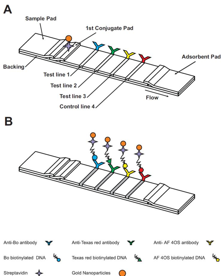
**Figure 3** Schematic representation of the lateral flow immunoassay test with colloidal gold nanoparticles before (A) and after (B) use.
