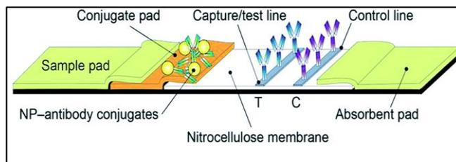
**Figure 1** Diagram showing the configuration of lateral flow immunoassay (taken from Petryayeva and Algar, 2015).
