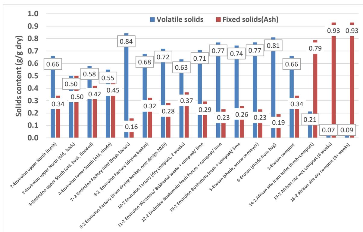
**Figure 14.18: Summary of volatile solids and ash content of the analysed solid samples.**
