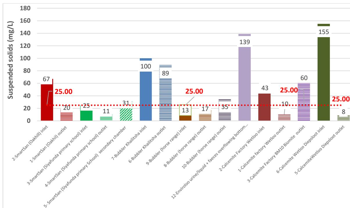
Figure 14.16: Suspended solids content of the analysed water-borne technologies.
