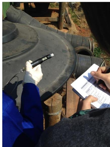
Taking temperature measurements with thermocouple and datalogger
