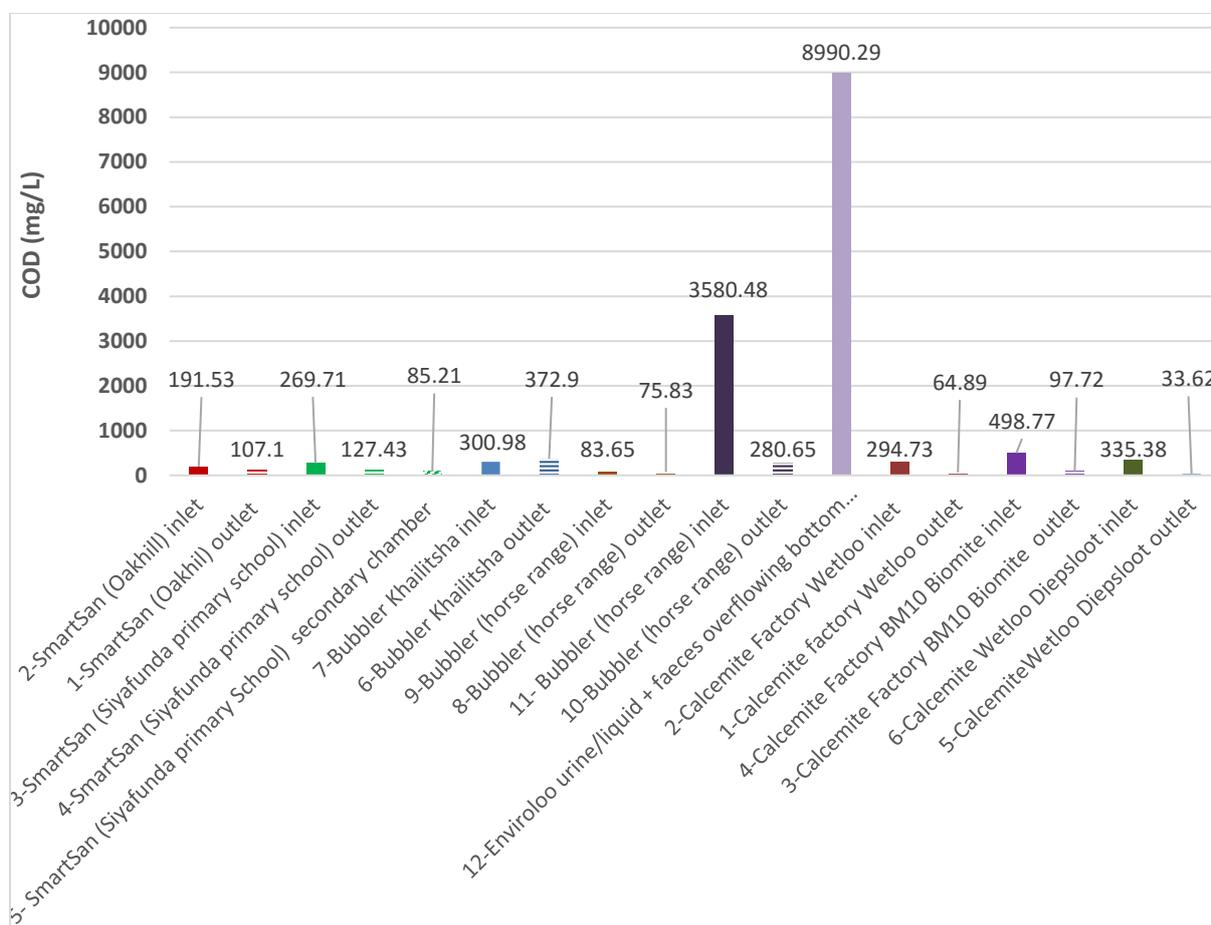
Figure 14.3: Chemical Oxygen Demand for collected liquid samples - 1.
