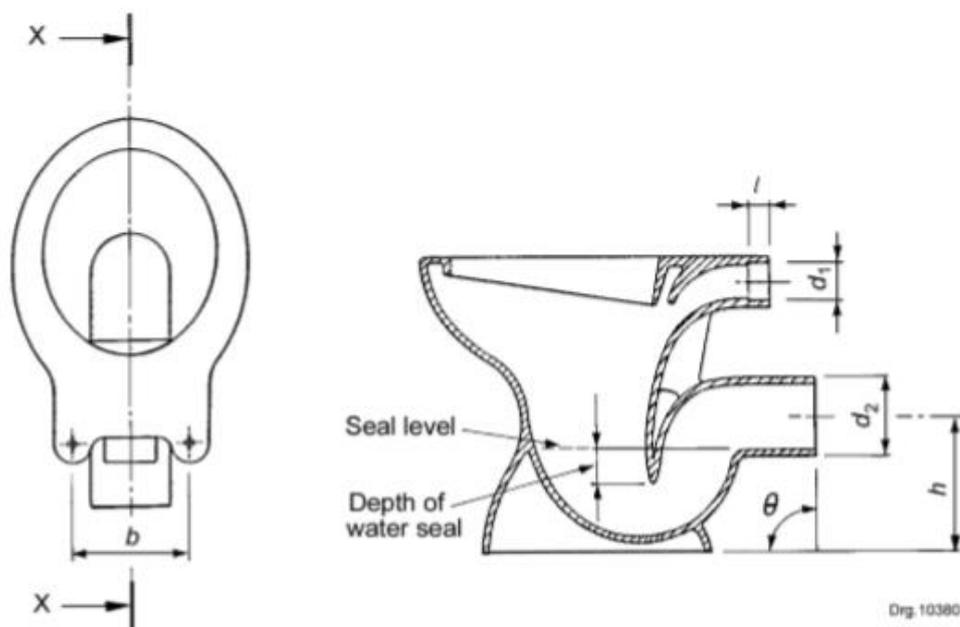
Type A pan (with seat fixing holes)
