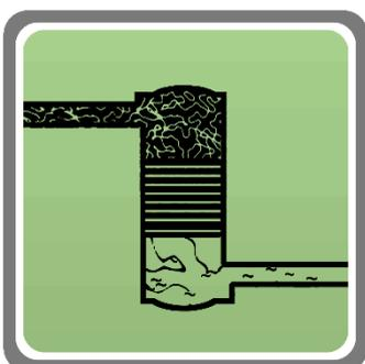
The process of treating the faecal waste for subsequent use or disposal. This will primarily involve the removal of faecal coliforms but may also include trash removal and dehydration processes.
