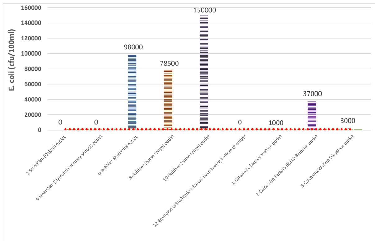
Figure 14.13: E. coli content for liquid outlet samples.
