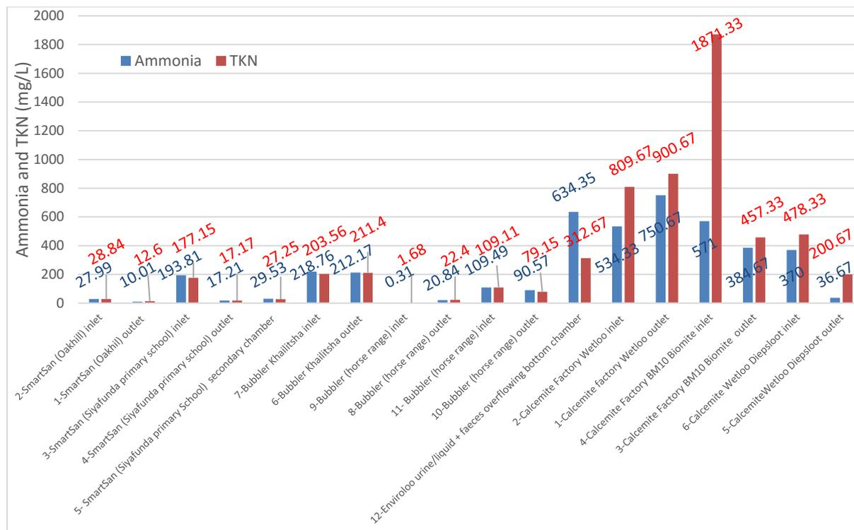
**Figure 14.20: Summary of nitrogen content (ammonia and TKN) of the analysed liquid samples.**
