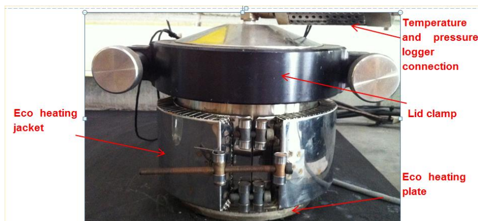
Figure 4.2 Hydrothermal reactor used for the conversion of amorphous \text{TiO}_2 nanoparticles to crystalline \text{TiO}_2 nanoparticles
