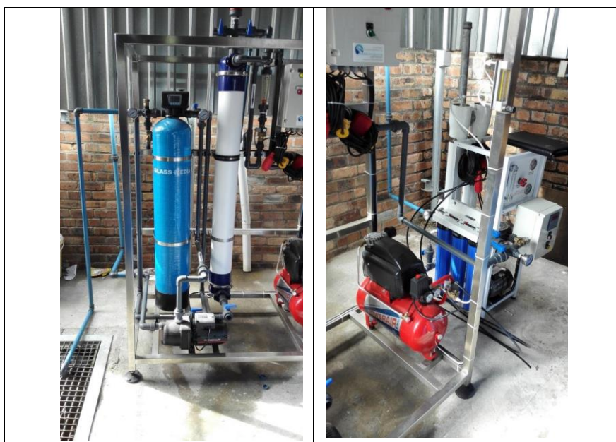
Figure 8.3 UF/NF pilot plant set up at Falke
