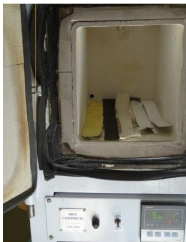
Figure 5.1 Programmable furnace used for the thermal treatment of electrospun PAN mats (stabilisation and carbonisation)
