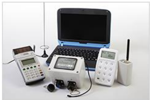
Figure 5-3: Vending and communication infrastructure of USC prepaid metering system (courtesy of Utility Systems)
