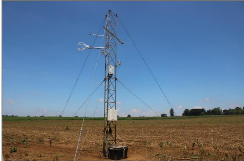
**Figure 39: The newly installed EC150 in a recently planted maize field at Baynesfield**
