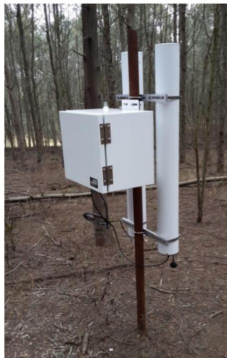
**Figure 15: A CRP installed in the middle of wattle trees at Two Streams Research Catchment**
