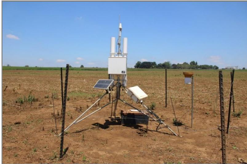
**Figure 41: The CRP and CS616 soil water probes at Baynesfield**
