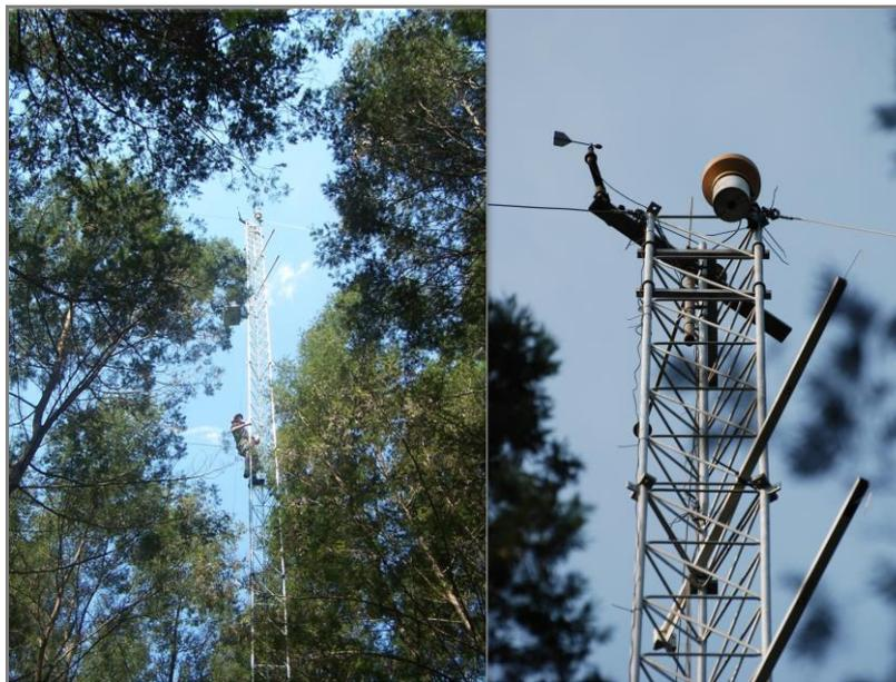
Figure 14: The surface renewal and automatic weather station sensors mounted on the 24 m mast at Two Streams
