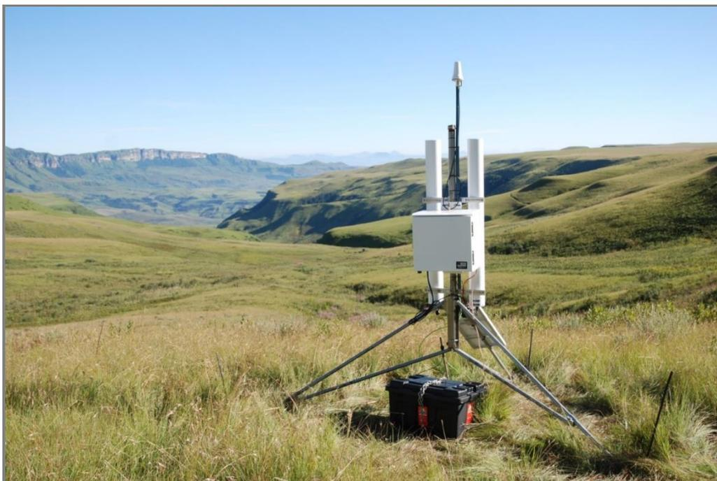
Figure 12: A CRP installed in the middle of Cathedral Peak Catchment VI
