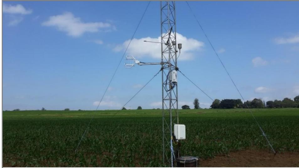
**Figure 6: EC150 open path gas analyser and 3D sonic anemometer installed above the maize canopy at Baynesfield**
