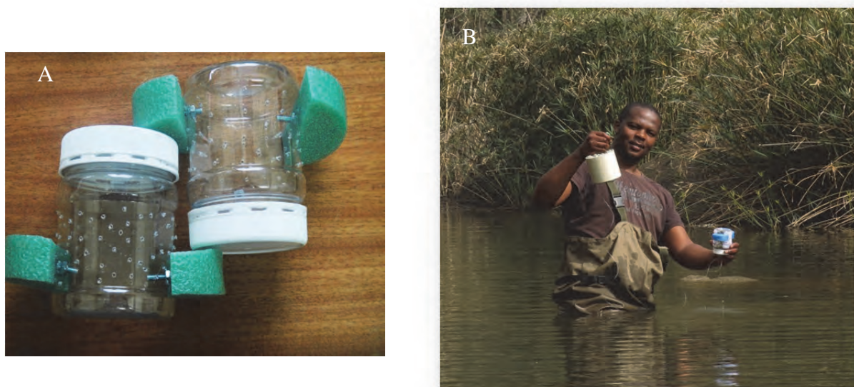
Figure 2: Construction (A) and deployment (B) of floating greenhouse cages for the transplantation of Spirodela sp. plants into the Bushmans-New Years River system.
