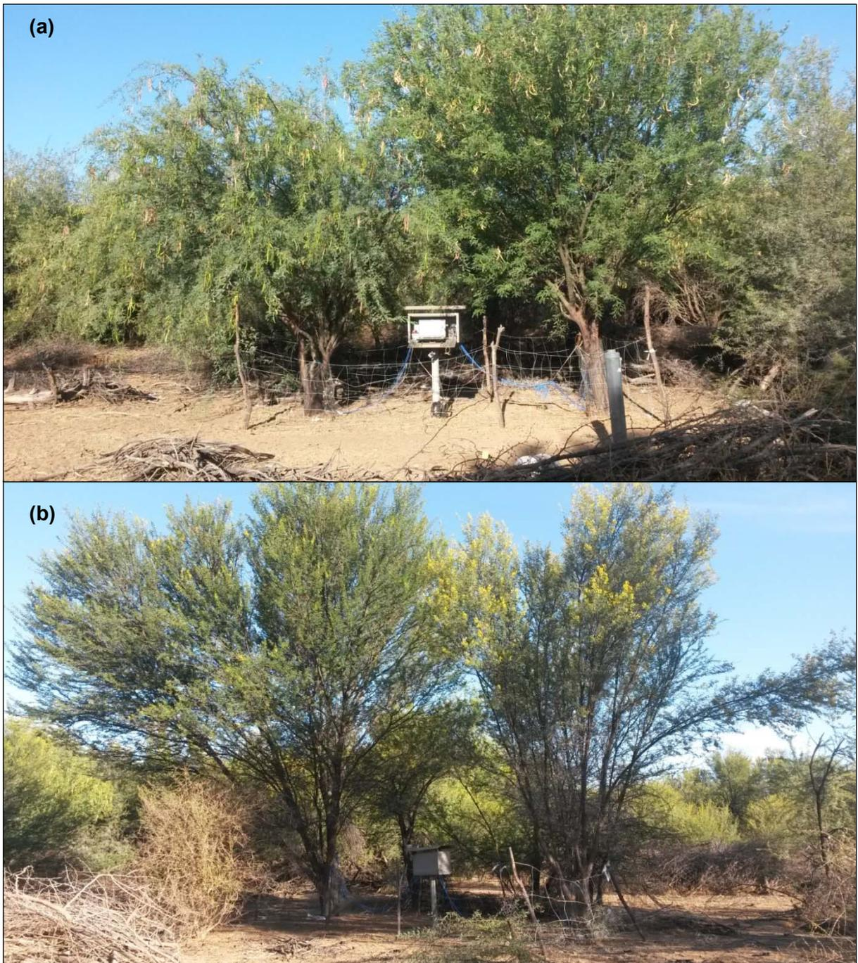
Figure 7. Heat pulse velocity sap flow equipment monitoring transpiration by (a) *Prosopis* invasions and; (b) *V. karroo* trees.
