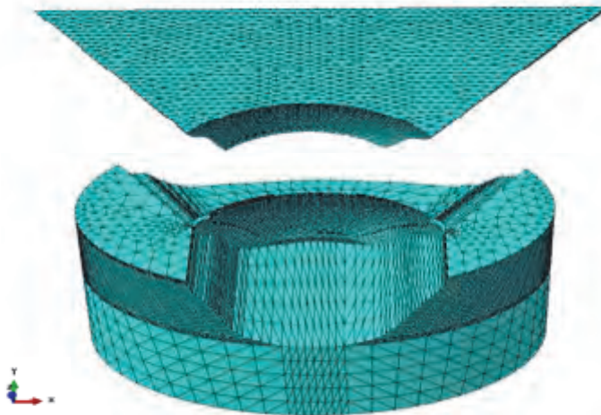
Figure 3.7: Meshed fluid region using AC3D10 quadratic tetrahedral elements and dam-foundation part meshed using C3D10 quadratic tetrahedral elements.
