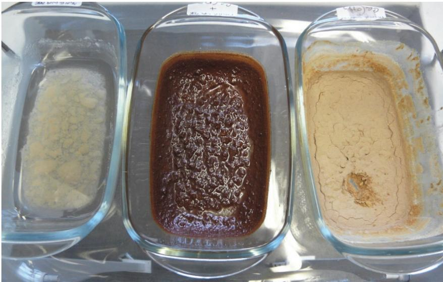
Small basins for mine water neutralisation and evaporation without soil
