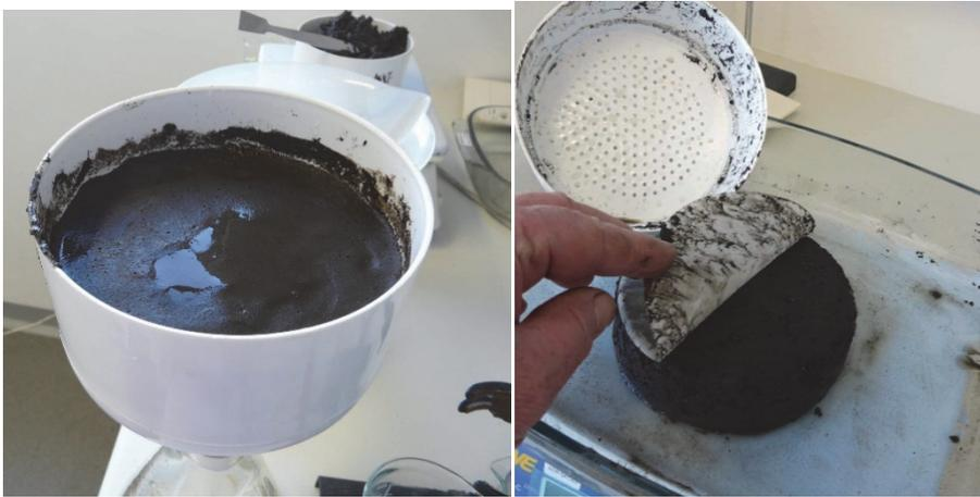
Vacuum extraction of black clay: caking facilitated return to the evaporating basin
