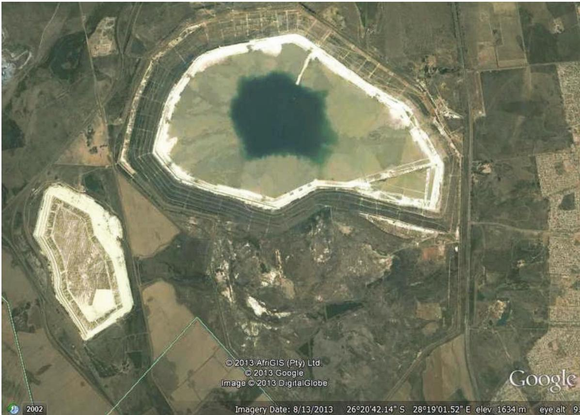
**Figure 2 Ergo's Brakpan Dam tailings storage facility south of Brakpan adjoining the Blesbokspruit and the Heidelberg Road. The top of the dam is 3.5 km wide and has an area of about 600 ha. Slurry is still pumped into the facility from a site adjacent to where underground water will be pumped at Grootvlei near Springs.**
