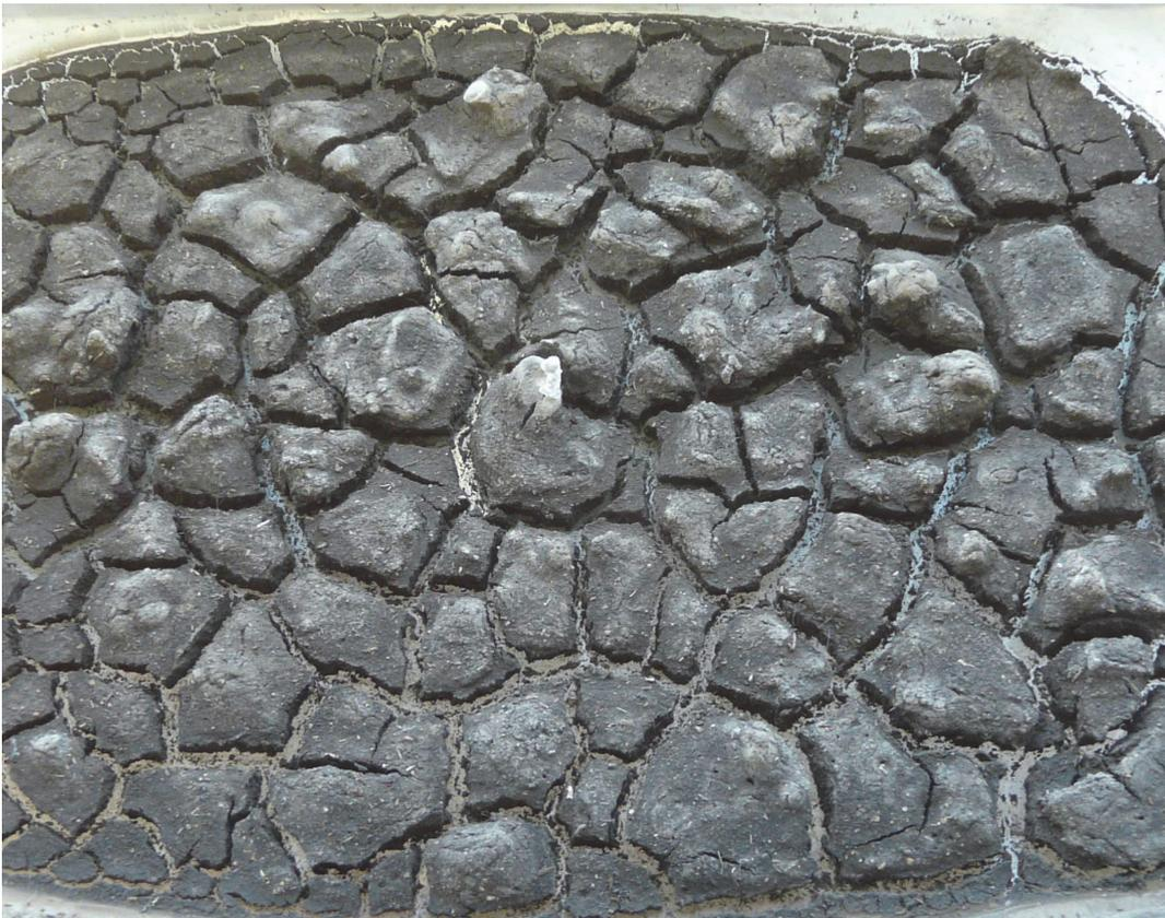
Black clay soil after drying with efflorescence of (mainly) gypsum crystals on peds.
