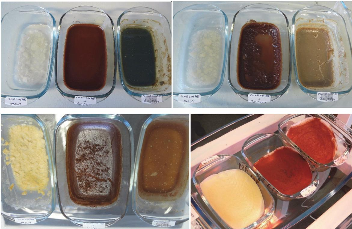
Sequence of residue development during the neutralisation and evaporative concentration of mine water. In each of the four pictures, the basin on the left is untreated mine water, in the middle is neutralised with  $\text{CaCO}_3$  and on the right with  $\text{Ca(OH)}_2$ . These are treatments OMO, OMC and OMH, respectively, as described in Table A1. The full amount of liming material was added to the basins at the start and the mine water was then added and evaporated daily for twenty days.
