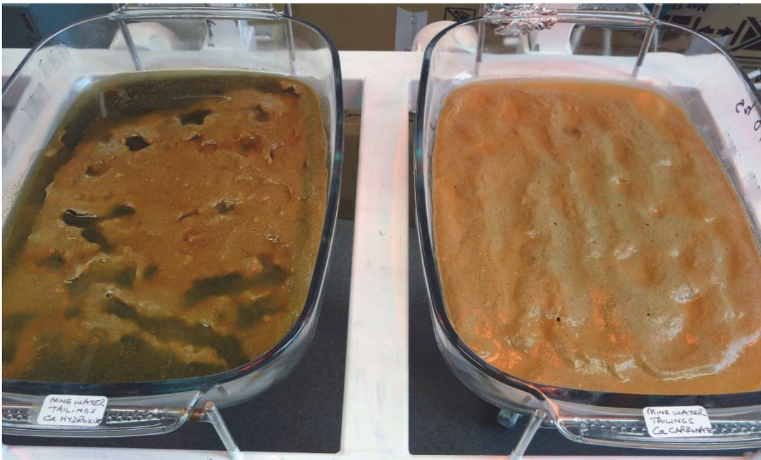
Initial result of mine water addition to tailings limed with  $\text{Ca(OH)}_2$  (left) and  $\text{CaCO}_3$  (right).
