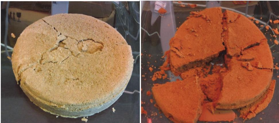
Late stage of treating tailings with alkaline amendment and mine water: no amendment (TMO, left);  $\text{Ca}(\text{OH})_2$  (TMH, right); before (above) and after (below) vacuum extraction of leachate.
