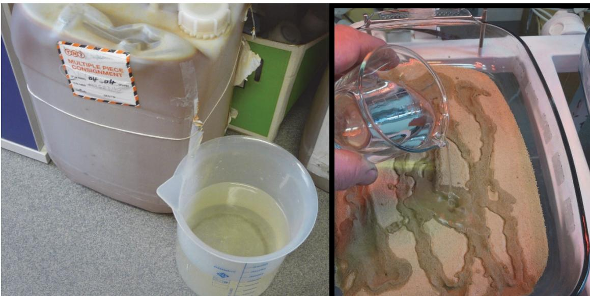
Mine water dispensed from storage tub (left) and added to tailings (right)
