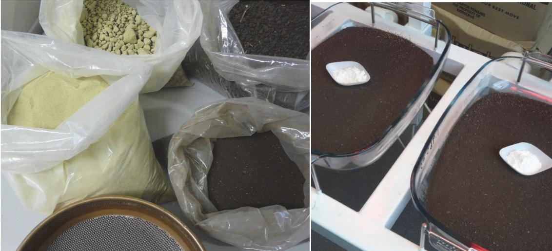
Mine tailings and black clay soil sieved (left) and alkaline treatments applied (right)
