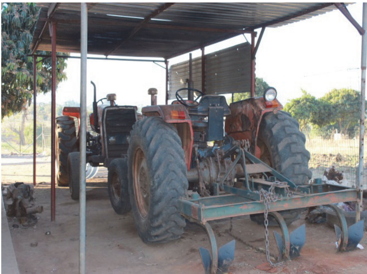
FIGURE 7.7: Phathutshelo's two tractors, one with a ridger attached and the other with a disk plough
