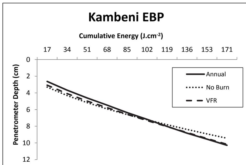
Figure 4.10 Average soil compaction measured using a drop-cone penetrometer on Kambeni EBP
