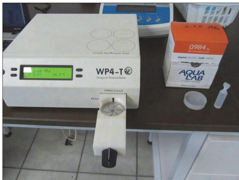
Figure 3.6 Photograph of a WP4-t dewpoint potentiometer used to measure water potential
