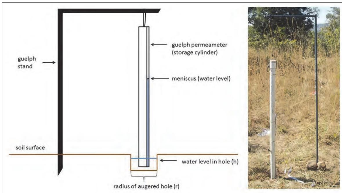
Figure 3.2 An illustration of a Guelph permeameter setup in the field
