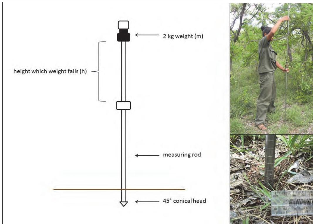
Figure 3.4 The different components of a penetrometer and how it is applied during measurement
