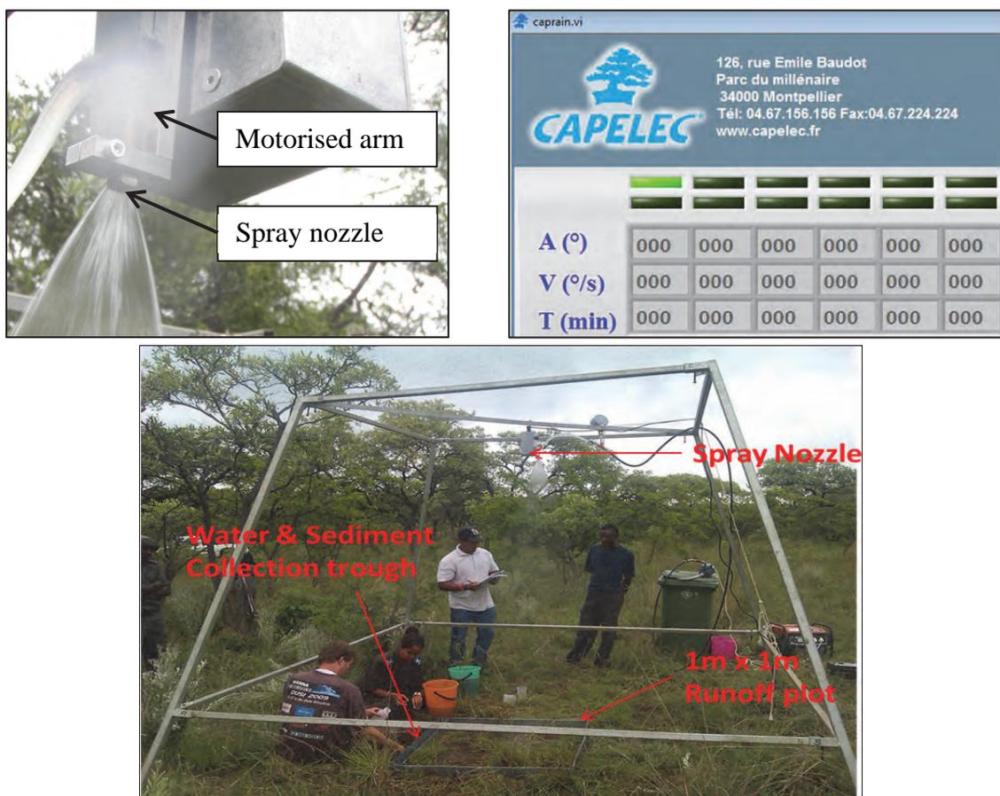
Figure 3.7 Rainfall simulator (top-left); CAPRAIN 1700 Computer program (top-right); field set-up (bottom)
