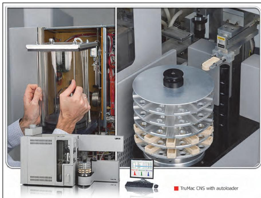
Figure 3.5 The Leco TruMac Series used to measure percentage total carbon to infer soil organic matter content (LECO Corporation [www.leco.com](http://www.leco.com))
