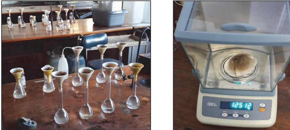
Figure 3.10 Filtration of samples (left) and weighing of the filtered samples (right)
