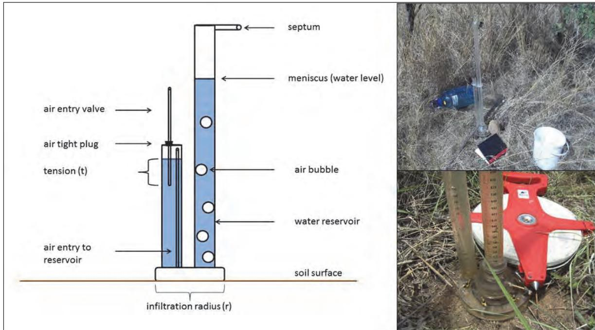
Figure 3.1 The various components of a tension disc infiltrometer and how it is used in the field
