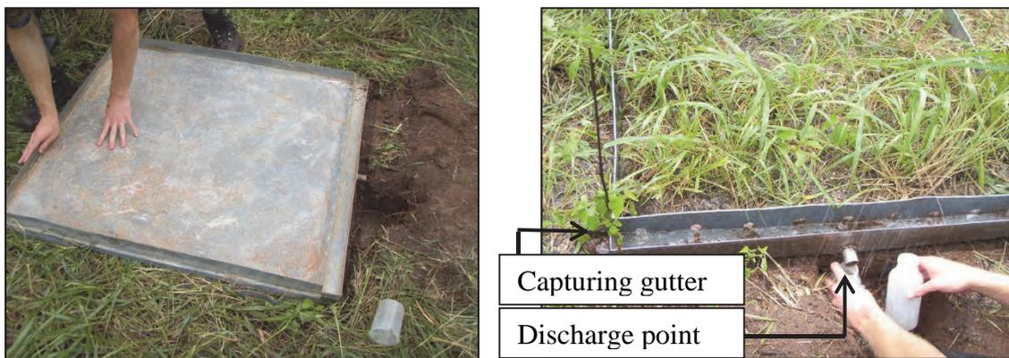
Figure 3.8 Calibration frame (left) and runoff plot (right)
