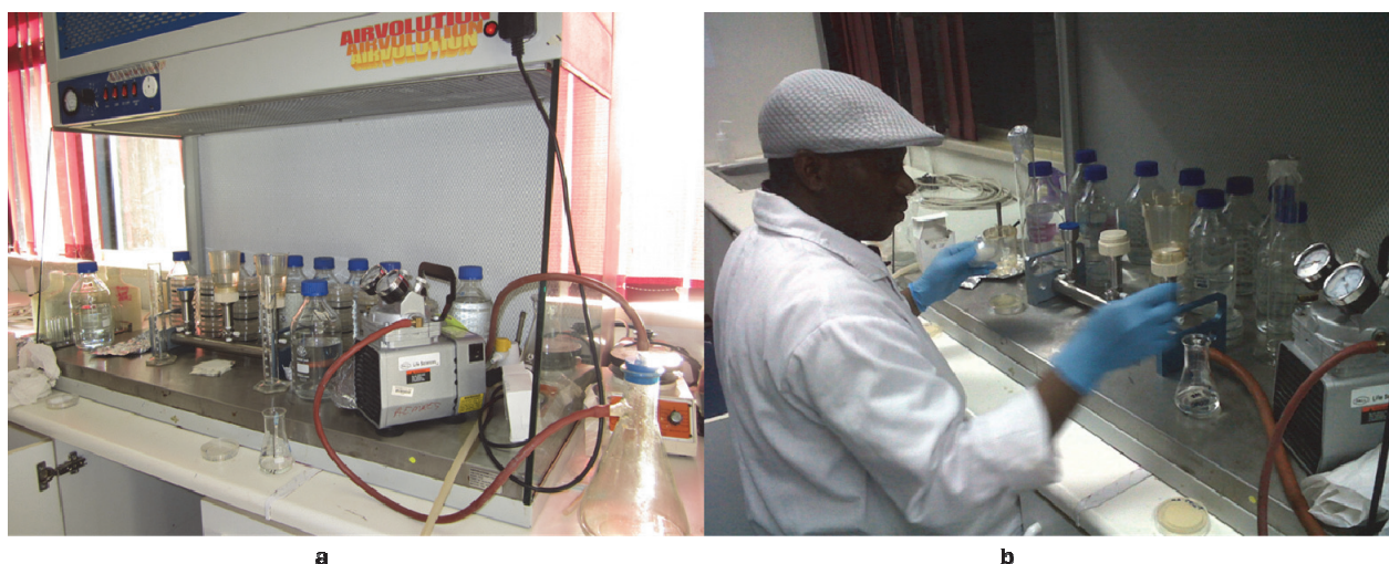
Figure 5.1: (a) Equipment setup for the membrane filtration assay and (b) A student uses the membrane filtration technique to process wastewater samples for bacteriological analysis
