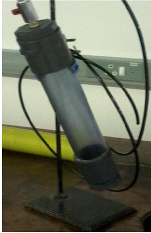
FIGURE 6. CAPILLARY EXTRUDER
