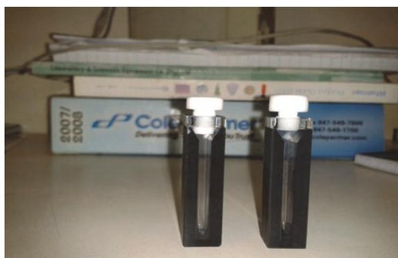
**Figure 3.1: Cuvettes pieces used in UV-vis analysis of samples**
