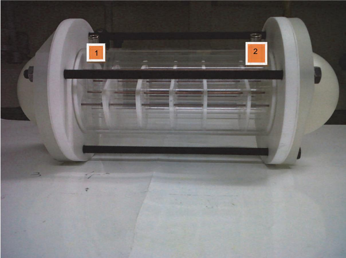
**Figure 4.24: New constructed EHD reactor**
