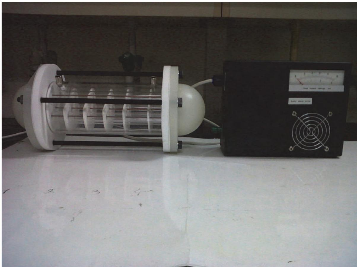
**Figure 4.27: New power supply and AC convertor to drive the EHD reactor**
