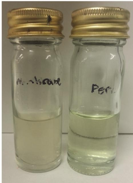
Figure 30: Photograph showing the difference between the sample from the membrane reactor (left) and the membrane permeate (right) collected during operation at a HRT of 1 day
