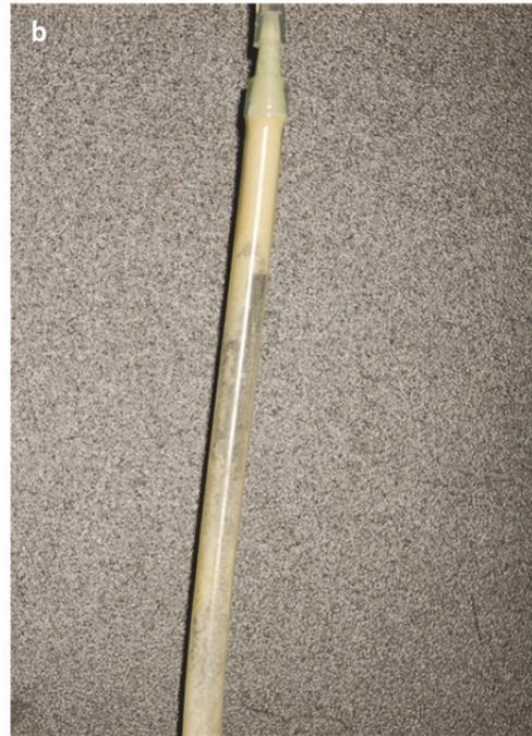
Figure 31: Photographs showing (a) the deposition of elemental sulphur in the peristaltic pump and effluent tubing and (b) a close-up of the effluent tubing
