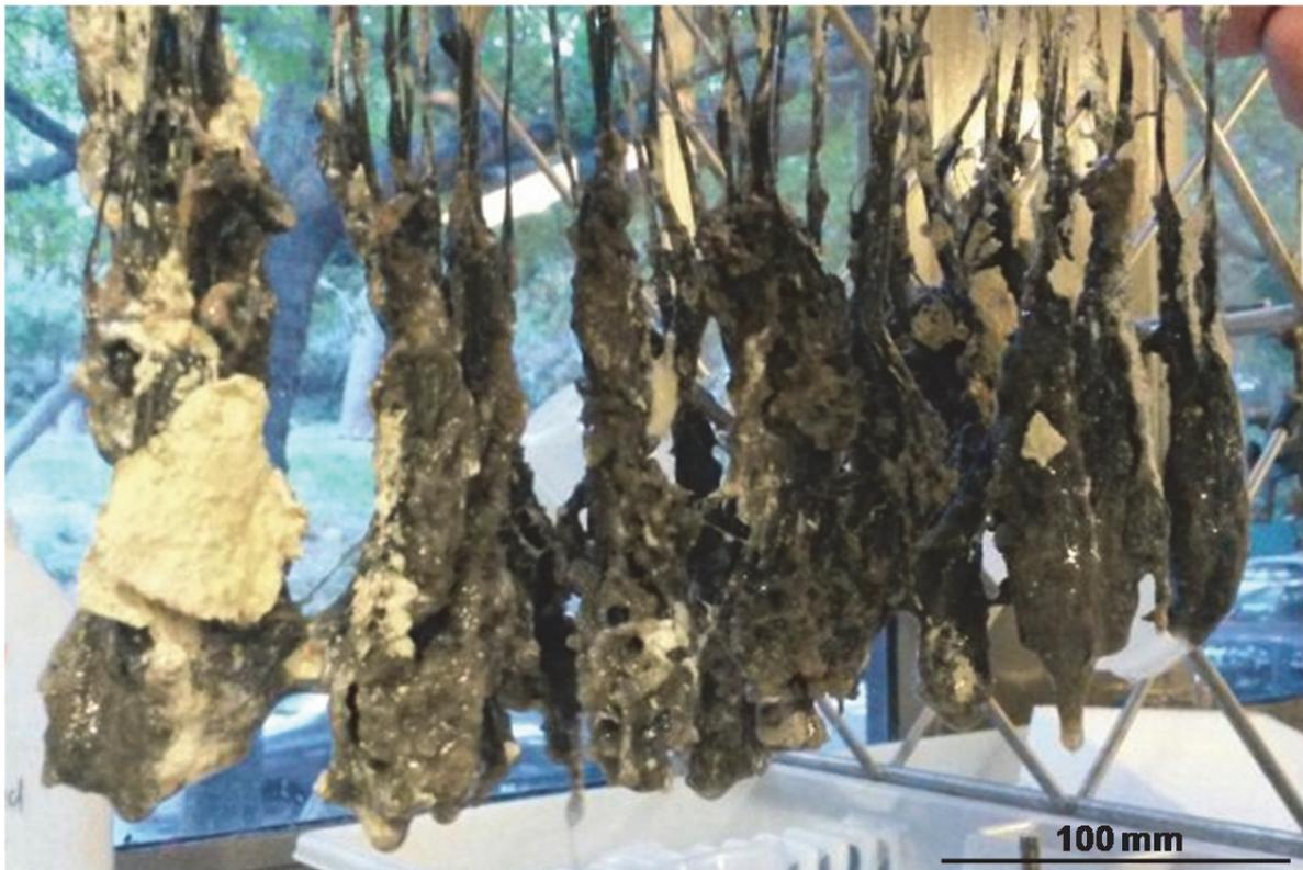
Figure 42: Photograph showing the extent of colonisation of the carbon fibres in the channel reactor
