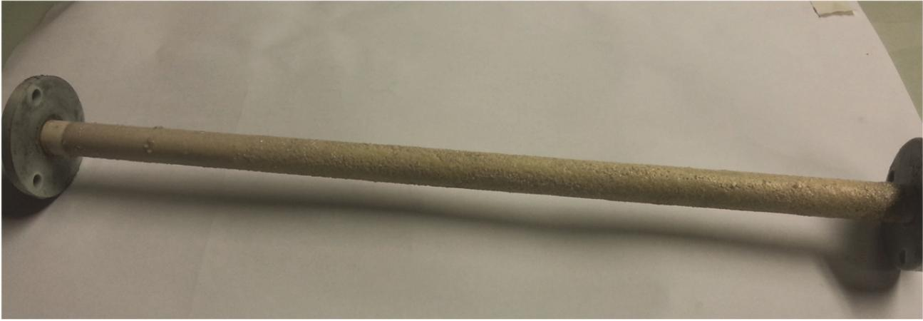
Figure 33: Photograph showing elemental sulphur deposition on the outer surface of the membrane. The sulphur layer is progressively thicker toward the right hand side of the image
