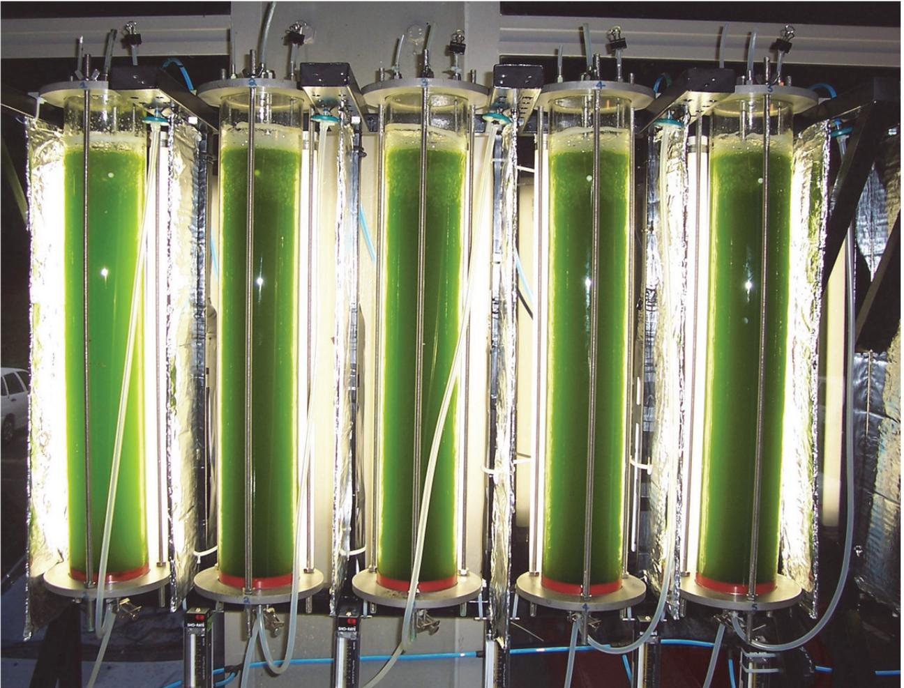
*Figure 2: Photograph showing a bank of five airlift photobioreactors used to perform the algal growth experiments*
