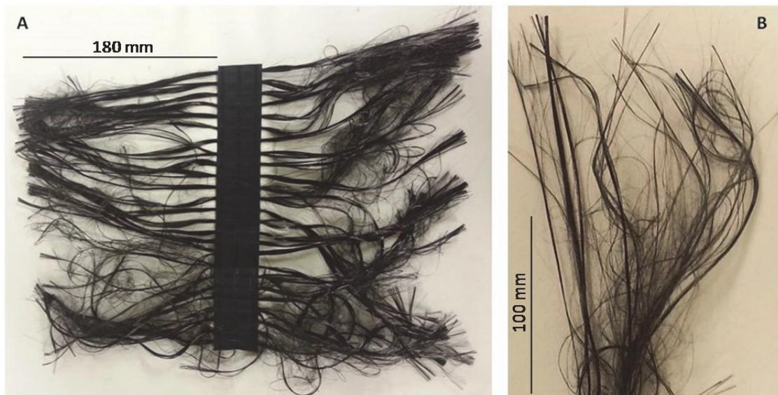
Figure 8: Photograph of carbon microfibres showing macrostructure (A) and detail of a single bundle (B) illustrating the large surface area for microbial attachment
