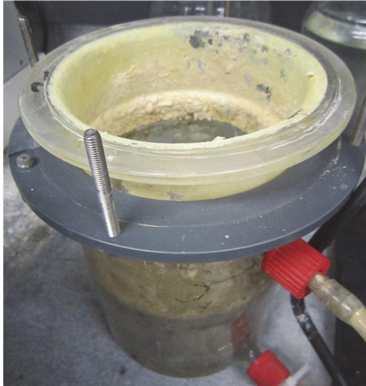
Figure 12: Photograph showing the deposition of elemental sulphur on the walls of the reactor near the air/water interface as a result of partial oxidation of sulphide
