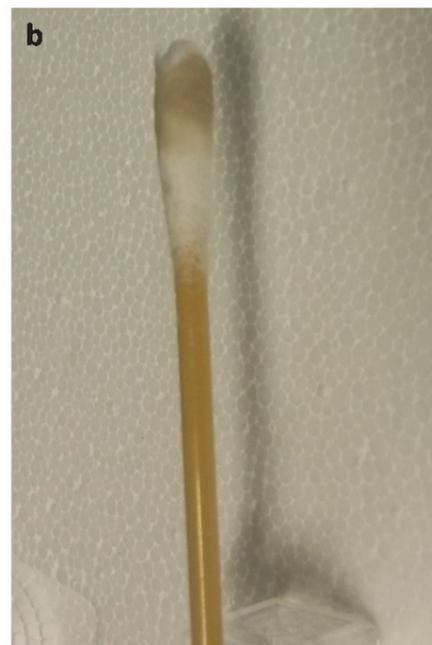
Figure 32: Photographs of (a) the base plate support the membrane showing biofilm growth on the base-plate and (b) biofilm scraped from the lumen of the membrane
