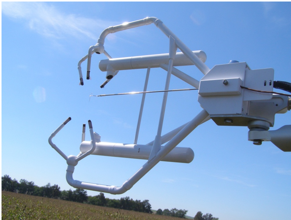
Figure 5. EC150 CO 2 and H 2 O Open-Path Gas Analyzer and 3D Sonic Anemometer with fine wire thermocouple in the middle.
