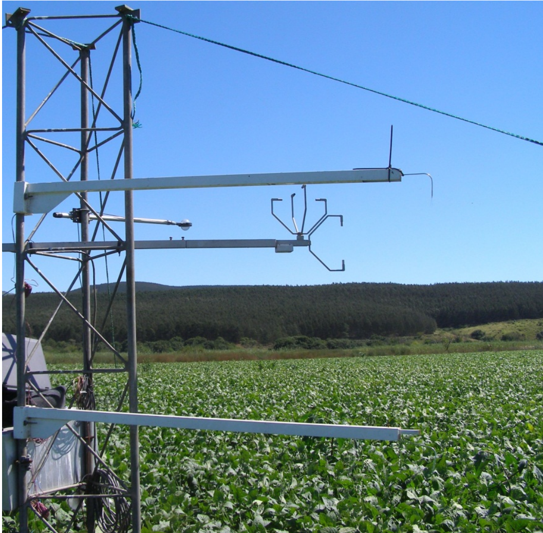
Figure 8. An Applied Technologies, Inc. (ATI) sonic anemometer, two surface renewal arms with fine wire thermocouples, and a net radiometer mounted on a lattice above the soybean canopy.
