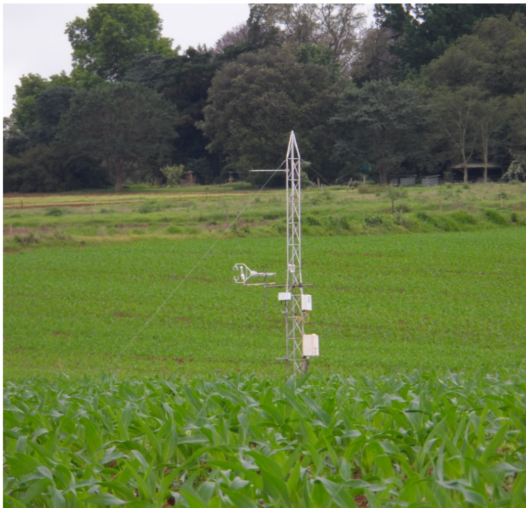
Figure 11. An extended Open Path (CSAT 3) eddy covariance system installed on a lattice mast above maize canopy.
