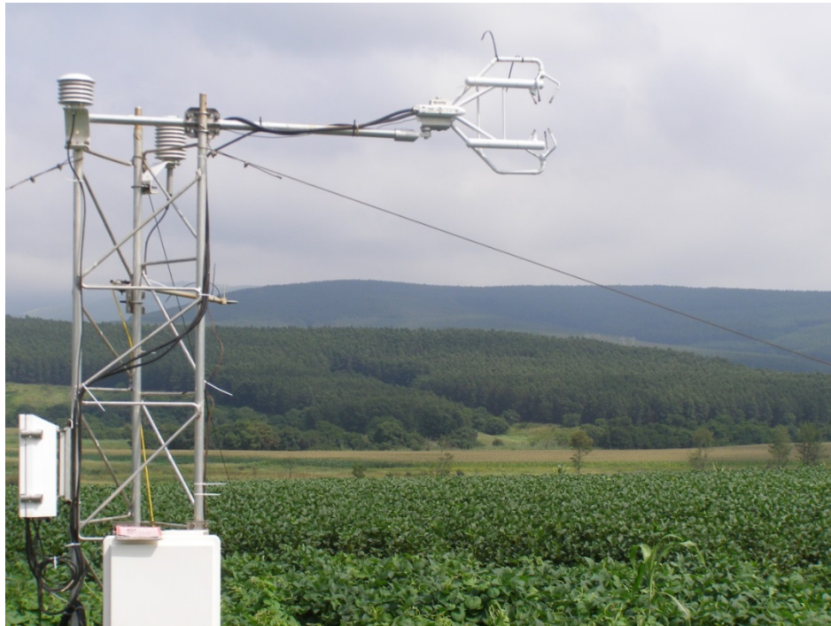
Figure 10. The EC150 eddy covariance system installed on a lattice mast in the middle of the soybean field.
