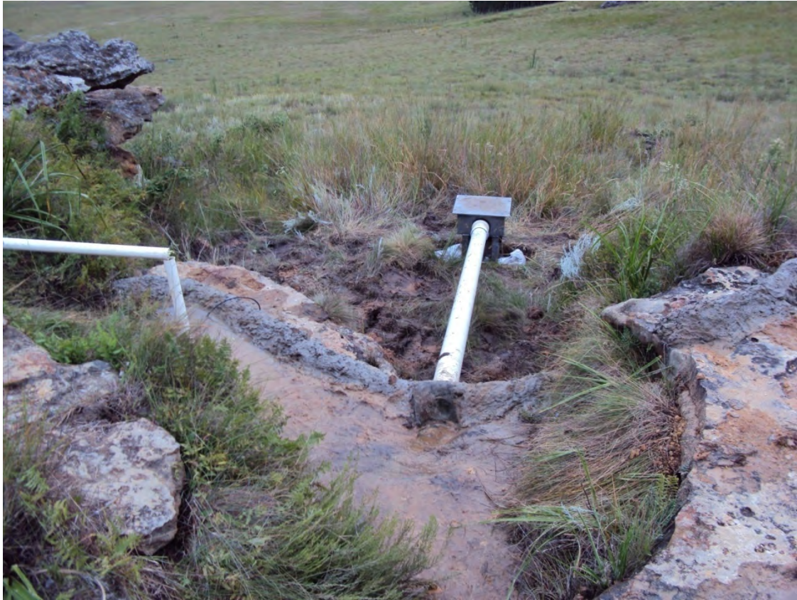
Figure 92 Tipping bucket measuring outflow from a selected portion of hillslope immediately below the investigated sites TB1 to TB4 shown in Figure 87c and in the cross section in Figure 88.
