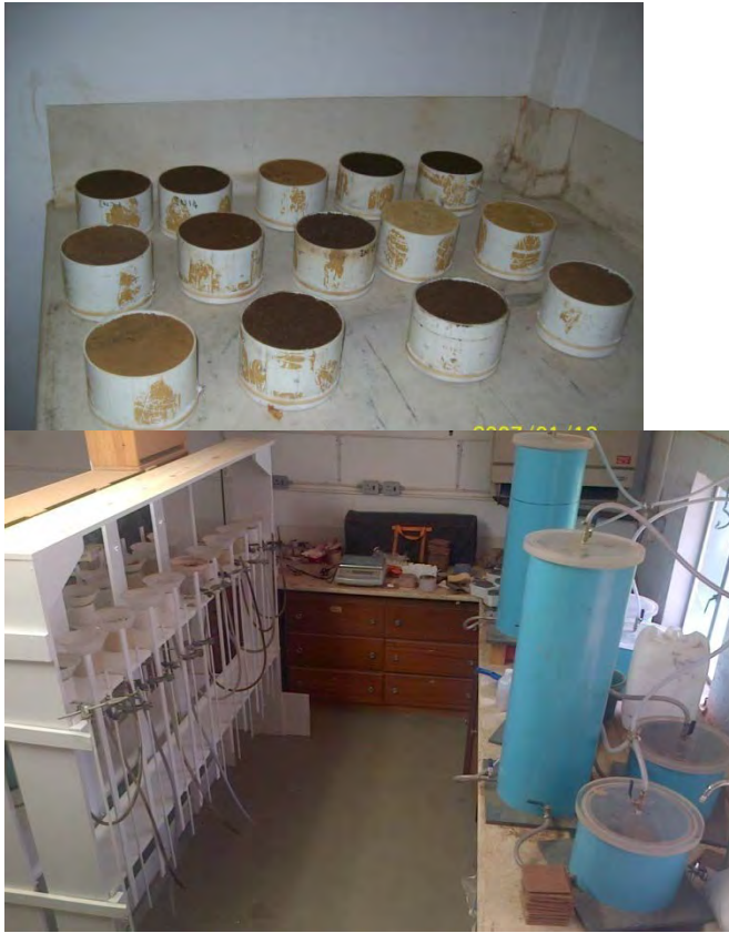
Figure 223 Photos illustrating (a) undisturbed core samples, (b) the laboratory vacuum/saturation chamber and hanging water column setup for determining water retention curves
