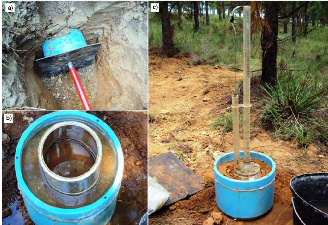
Figure 89 : Proposed method to determine lateral hydraulic conductivities in the field: a) the PVC ring being forced into a specific horizon by means of a hydraulic jack; b) the setup for double ring K measurements with the core now orientated vertically; c) the setup for lateral K(h) measurements by tension infiltrometer.
