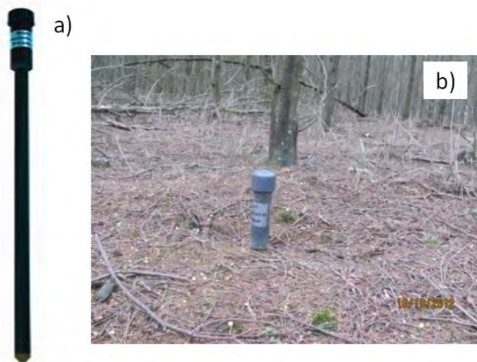
Figure 204 Standard version of 800 mm DFM capacitance probe with 6 sensors
