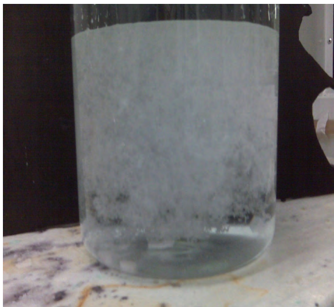
Figure 37: Ice and trapped salt at the top of the settling vessel.
