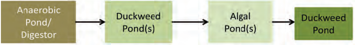
Figure 2-81: Suggested sequence of unit processes for optimum nutrient removal and effluent polishing
