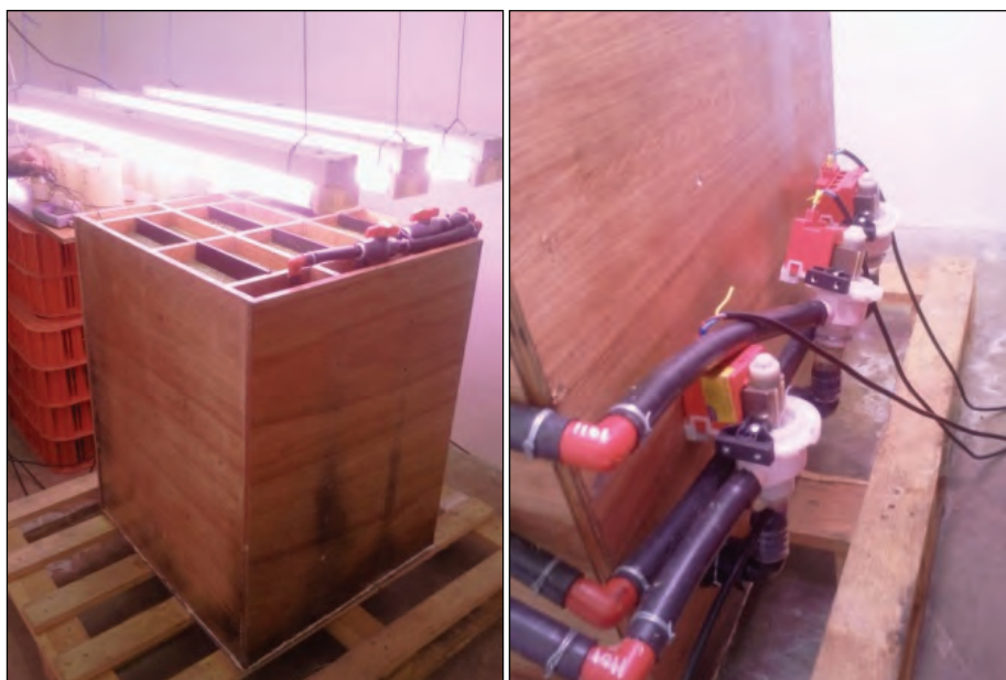
Figure 2-3: Reactor and light set up (left) and recirculation pumps (right)
