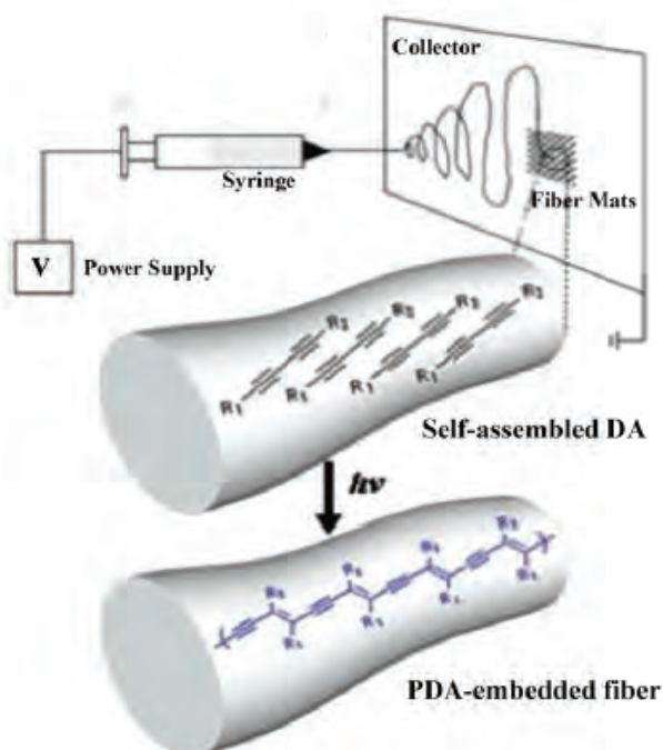
Figure 2.12: Schematic representation of the preparation of PDA embedded electrospun fibres (Yoon et al. , 2007)
