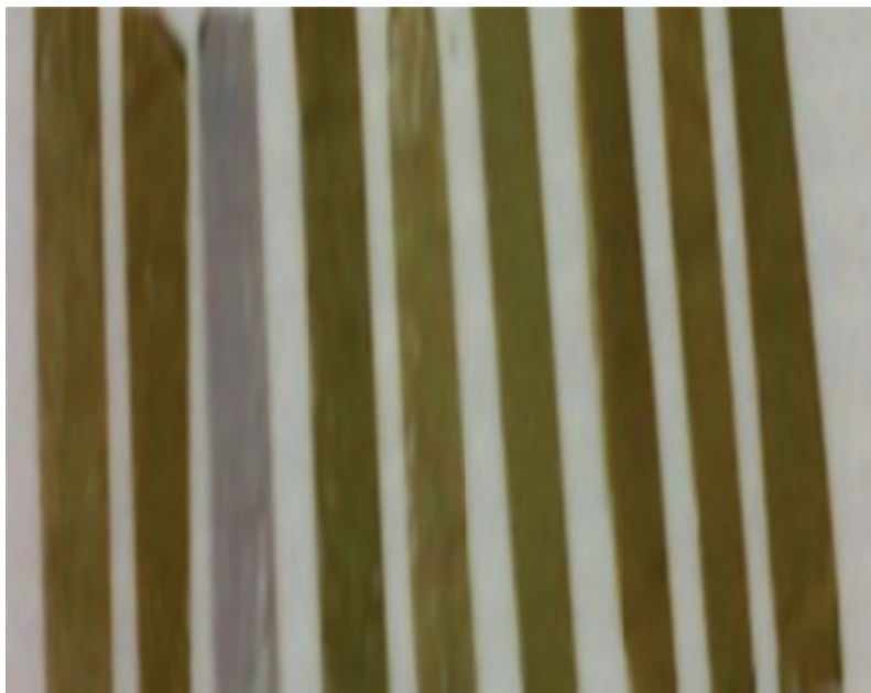
Figure 8.5: Colorimetric responses of the fibre strips to various solutions from left, \text{H}_2\text{O} , \text{Pb}^{2+} , \text{Ni}^{2+} , \text{Fe}^{2+} , \text{Na}^+ , \text{Cr}^{3+} , \text{Ca}^{2+} , \text{Mn}^{2+} and \text{Co}^{2+} respectively
