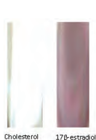
Figure 10.13: Interaction of the probe with cholesterol and 17 \beta -estradiol under the same conditions; 800 \mu g/mL, after 30 s contact time, alkaline conditions and at ambient temperature
