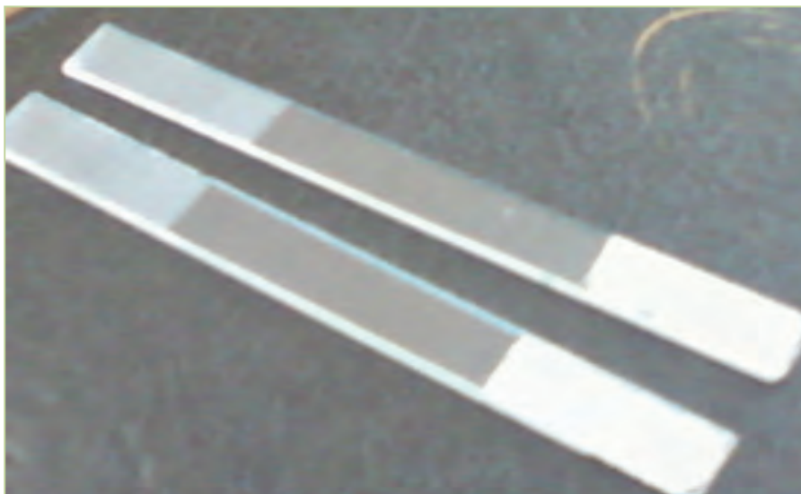
Figure 7.1: Photograph of glass slides coated with fluorescent nanofibres
