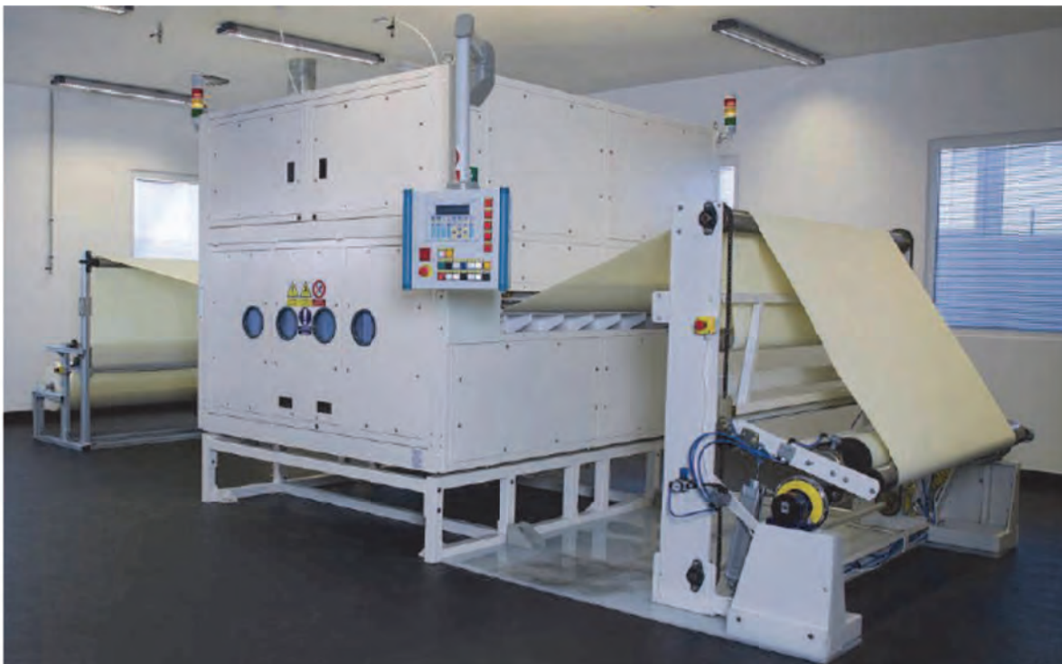
Figure 2.9: Nozzle-less production electrospinning line (Nanospider™) (Petrik and Maly, 2010)
