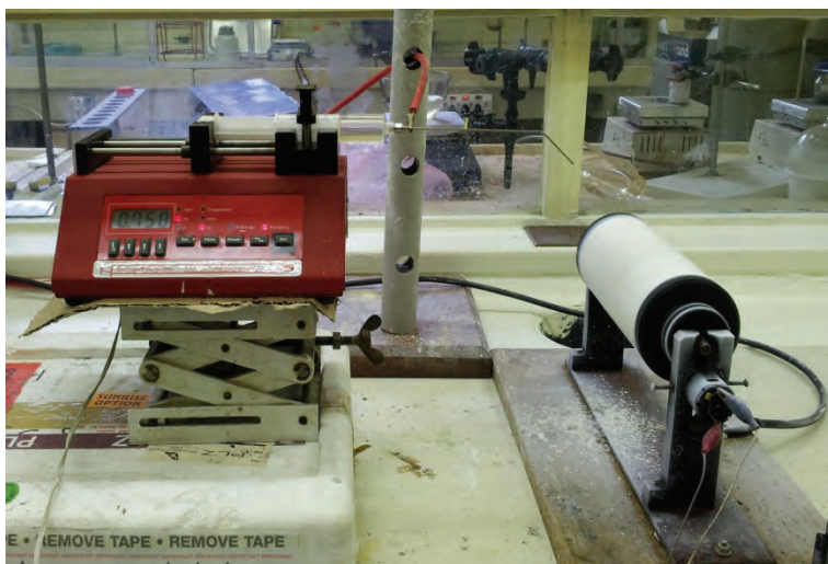
Figure 6.1: Electrospinning setup for fabrication of nylon 6 composite nanofibres
