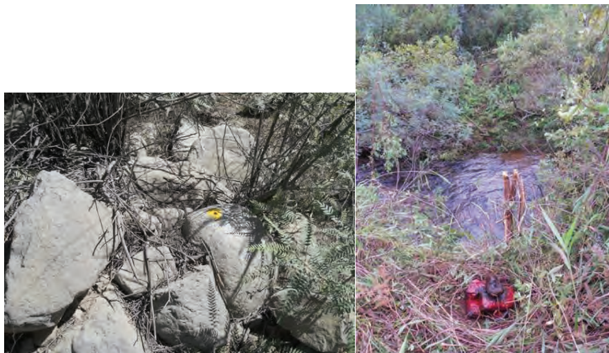
Figure 5.7 A permanent control point in a rock or as a metal stake cemented into the ground surrounded by a pyramid of rocks.
