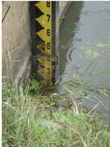
Figure 5.10 A stage plate photograph records the water level on the day.
