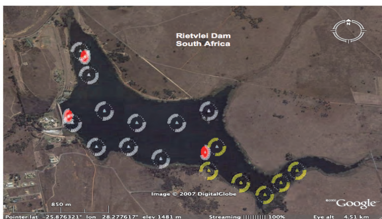
Figure 2-5: Placement of SolarBee machines in Rietvlei Dam. Yellow circles = first installation July 2008, White circles = second installation May 2009 and Red circles indicate sampling points.
