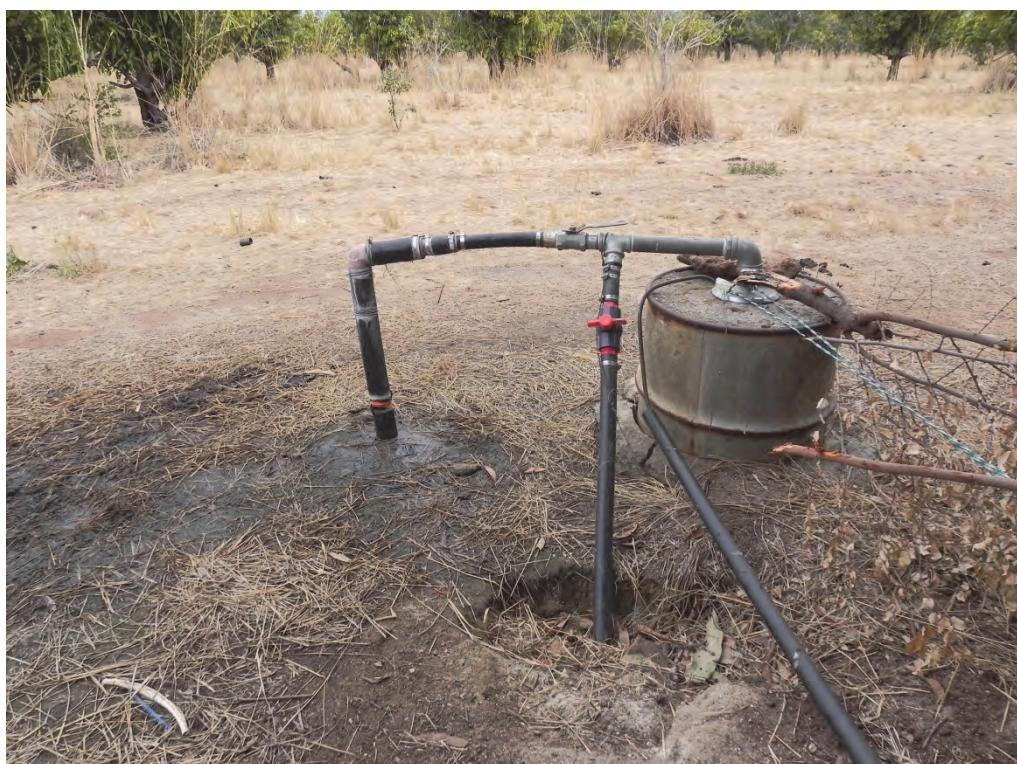
Photograph 7: Pumping equipment on respondent D's farm. Irrigating directly from the borehole is expensive.
