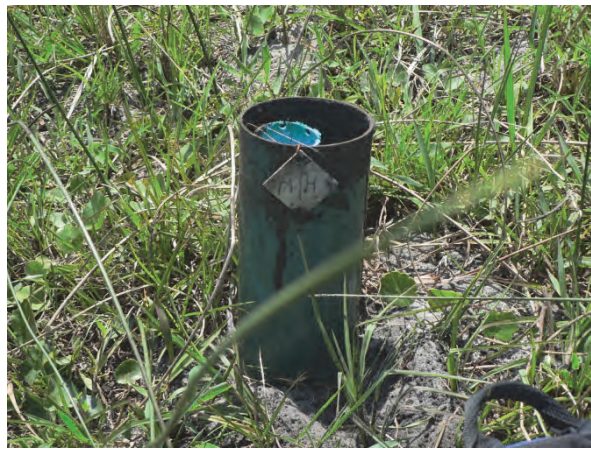
Figure 5.9: Example of a groundwater monitoring site on the Eastern Shores. Note the PVC well with steel protection and numbered tag.
