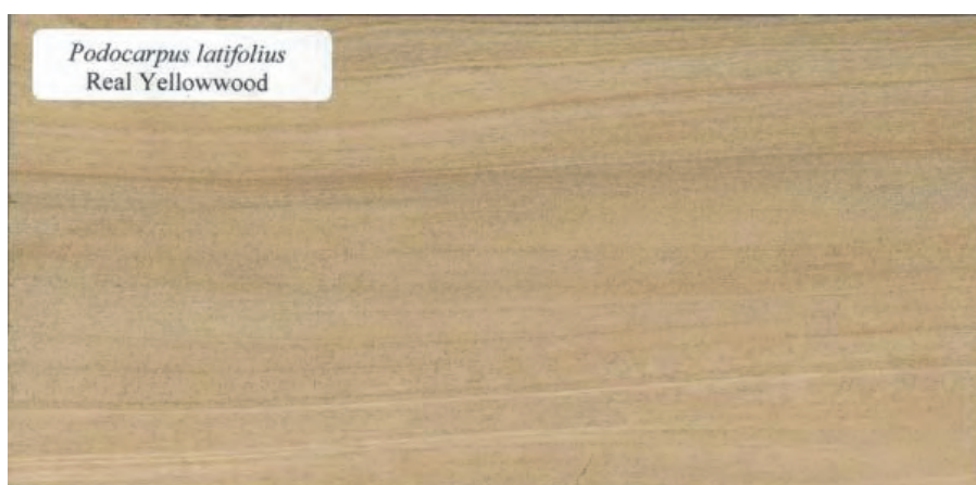
Figure 22. Standard untreated sample of Podocarpus latifolius (Photo: B. James).
