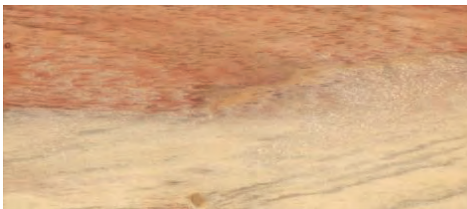
Figure 25. Standard untreated sample of Vachellia kosiensis , ex RBM mine path, showing the pink colouring of the heartwood (Photo: B. James).
