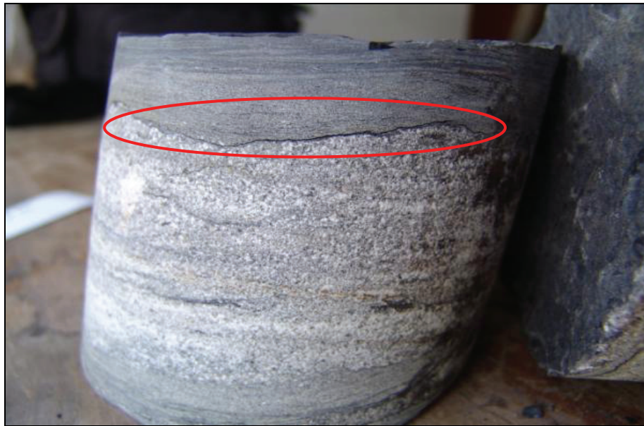
Figure 91: Rocks from the fractured aquifer zone, showing a bedding plane fracture (circled).
