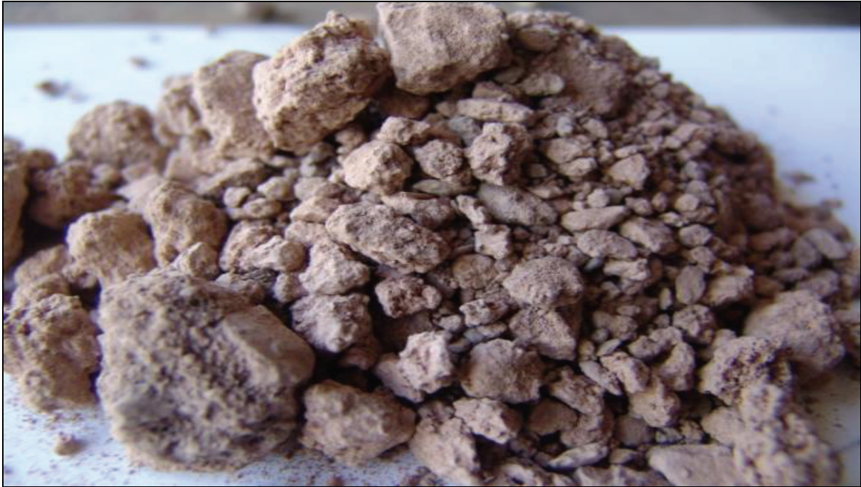
Figure 72: Sample GGSVZ1.4 4 m below the surface with acid potential.
