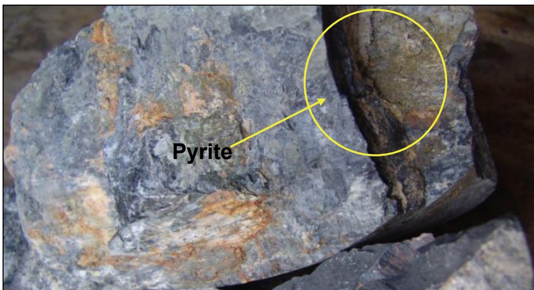
Figure 66: Sample SS6 showing the presence of pyrite.
