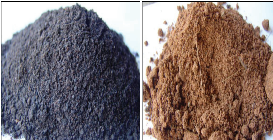
Figure 68: Samples GT1.9 and GT7.1, respectively, with acid potential.
