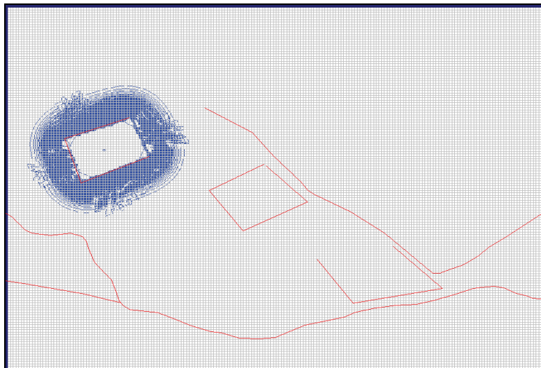
Figure 127: Dewatering of layer 4, showing layer 3's drawdown cone.
