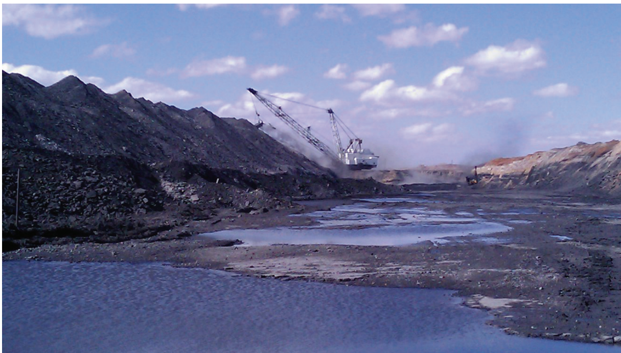
Figure 3: Dragline mining in an opencast pit.
