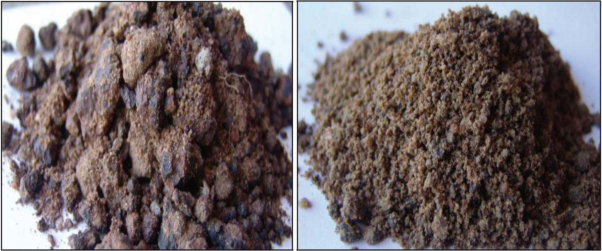
Figure 70: Sample GT3.2 (on the left) with acid potential and sample GT3.3 (on the right) with no acid potential
