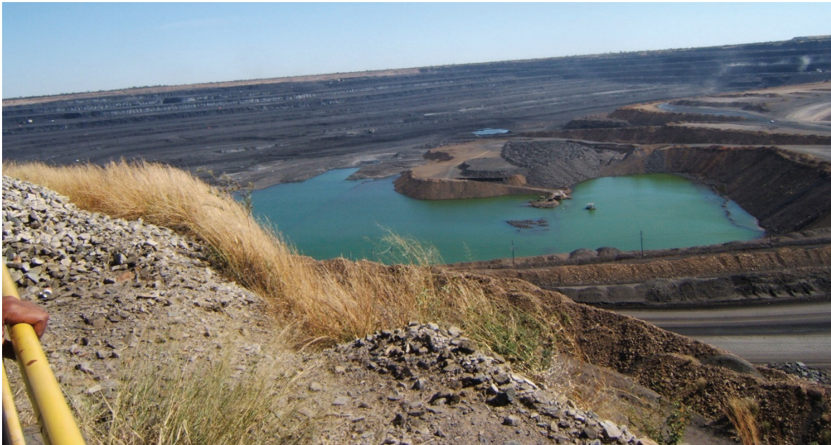
Figure 159: Surface runoff and groundwater inflow concentrated in a single location in the mine workings (courtesy of the Grootegeluk mine).
