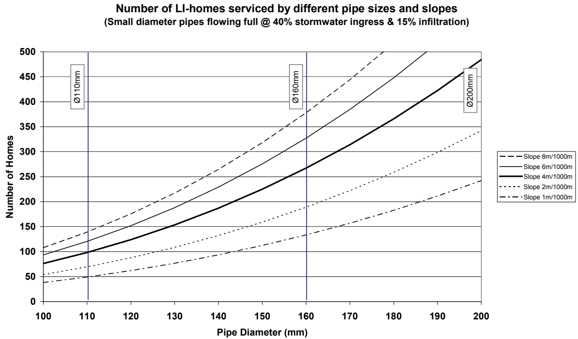
Figure 5.6a: Relationship between number of LI-homes, pipe diameter and slope ( D < \varnothing 200 mm)
