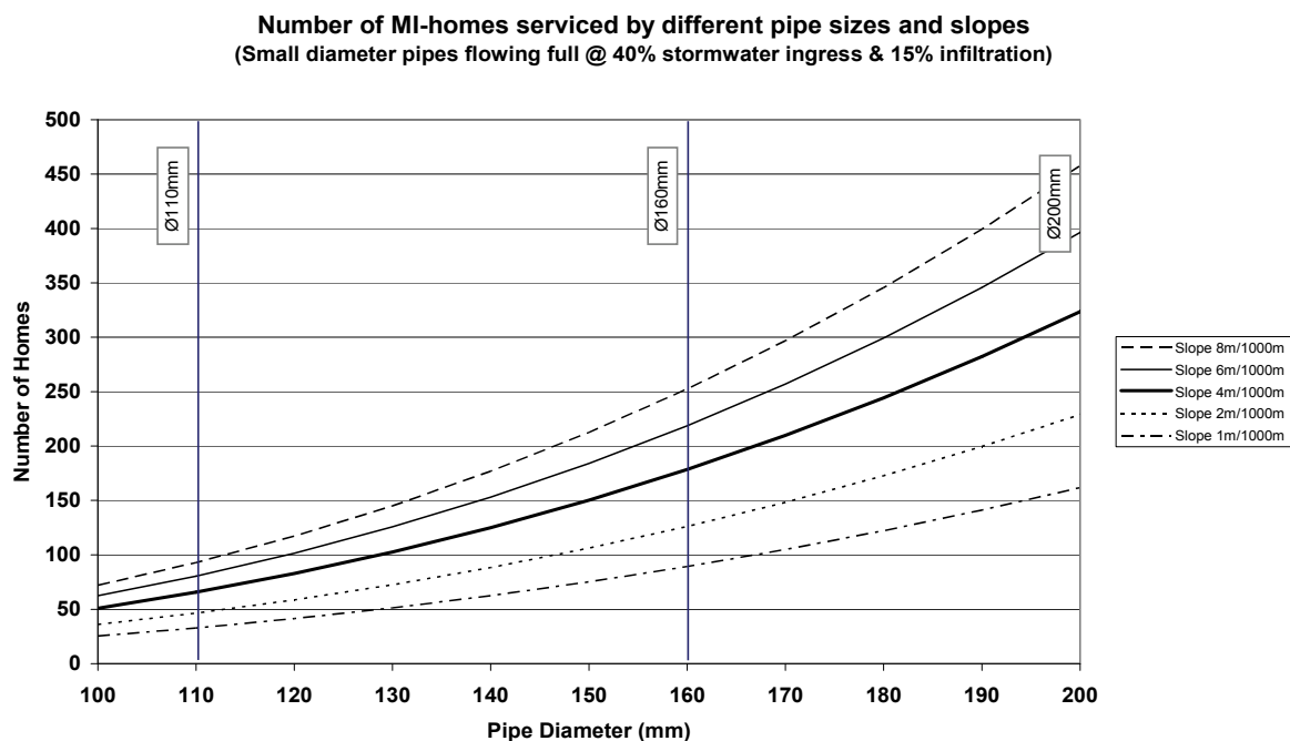
Figure 5.7a: Relationship between number of MI-homes, pipe diameter and slope ( D < \text{Ø}200 \text{ mm} )
