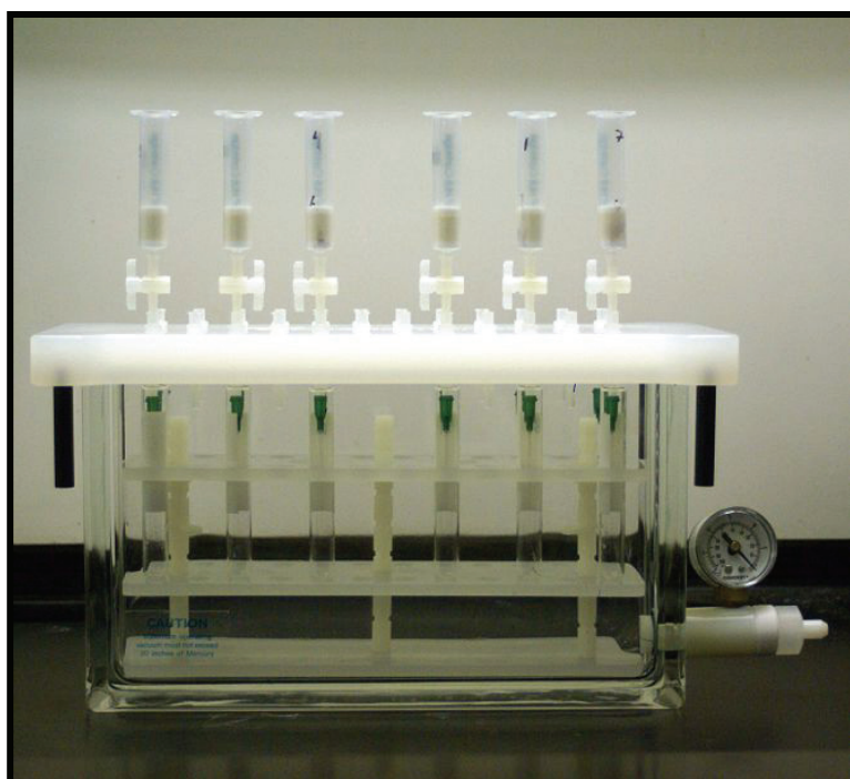
Figure 2b: An example of a solid phase extraction manifold
