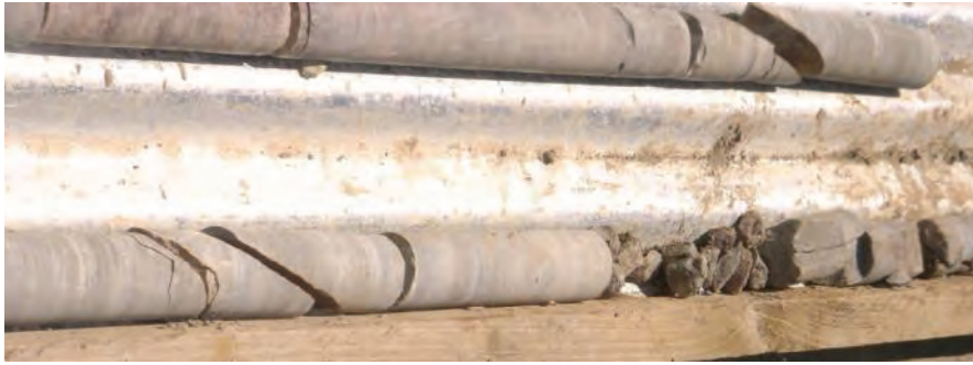
Figure 3-20 Fractured zone (13-18.5 m) in borehole BH4
