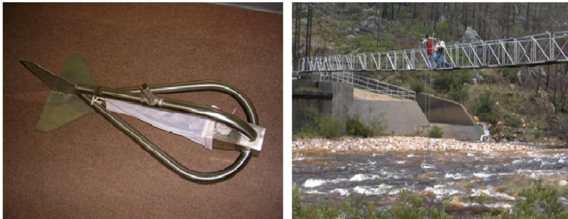
Figure 4.3-2 Typical bed load sampler (BL-84) and testing of the bed load sampler on the Berg River
