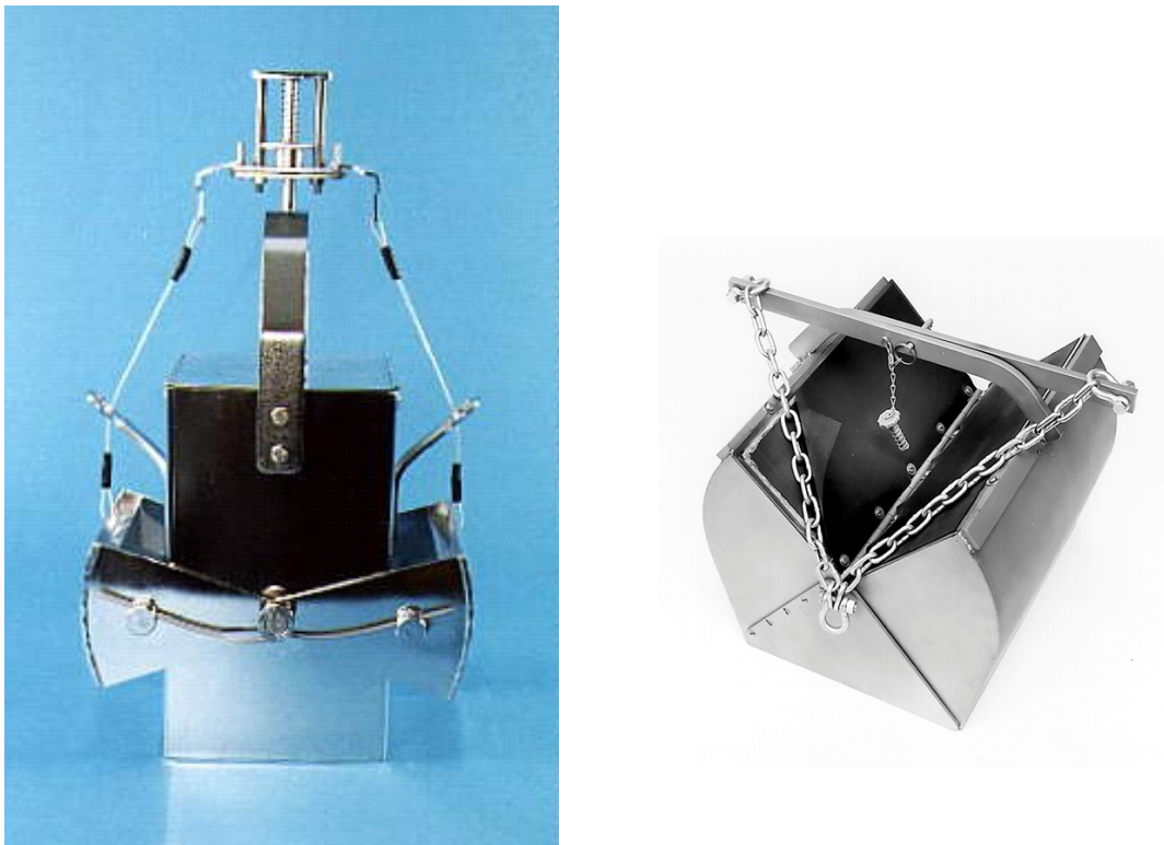
Figure 4.3-3 Ekman (left) and Van Veen (right) bottom sediment grab samplers
