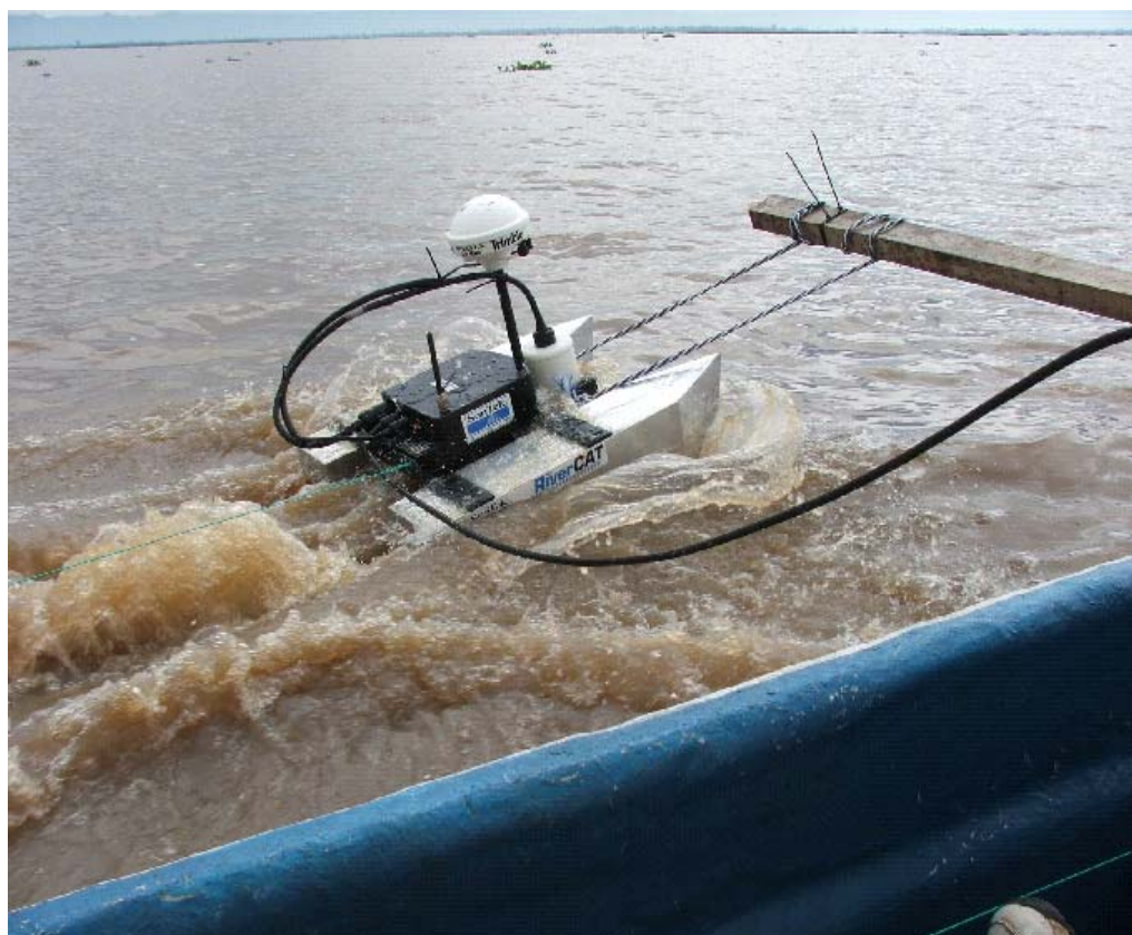
Figure 4.3-4 ADCP for discharge measurement
