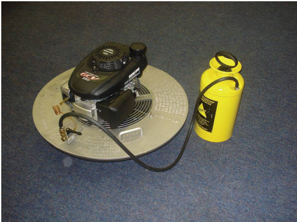
Figure A1: The smoke generator machine acquired by eThekweni Water Services to assist with the detection of direct stormwater to sewer connections
