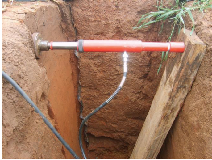
Figure 3.6 Illustration of how undisturbed soil samples for bulk density determination were obtained. The core sampler was gently pressed into the soil using a hydraulic jack.
