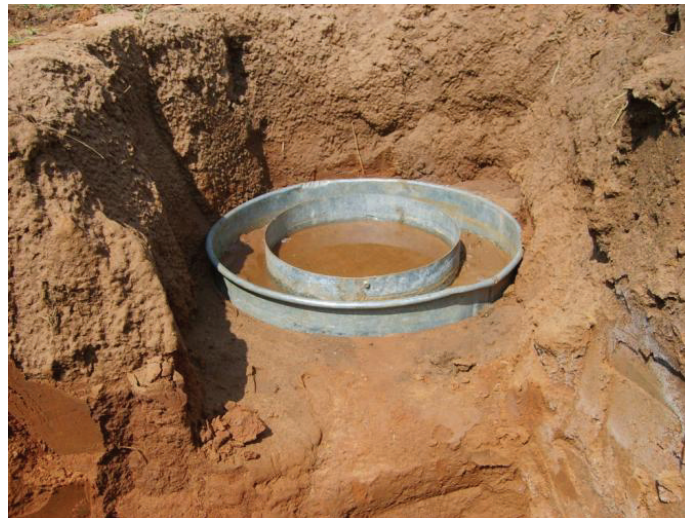
Figure 3.5 Example of the double ring method used to determine saturated hydraulic conductivity at the 300 mm soil depth.
