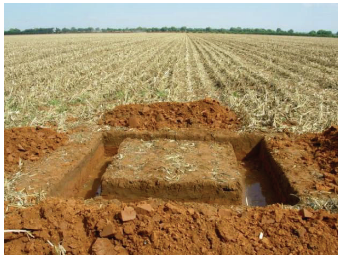
Figure 3.4 Example of a monolith at Orange-Riet Irrigation Scheme for determining the internal drainage parameters of the soil.
